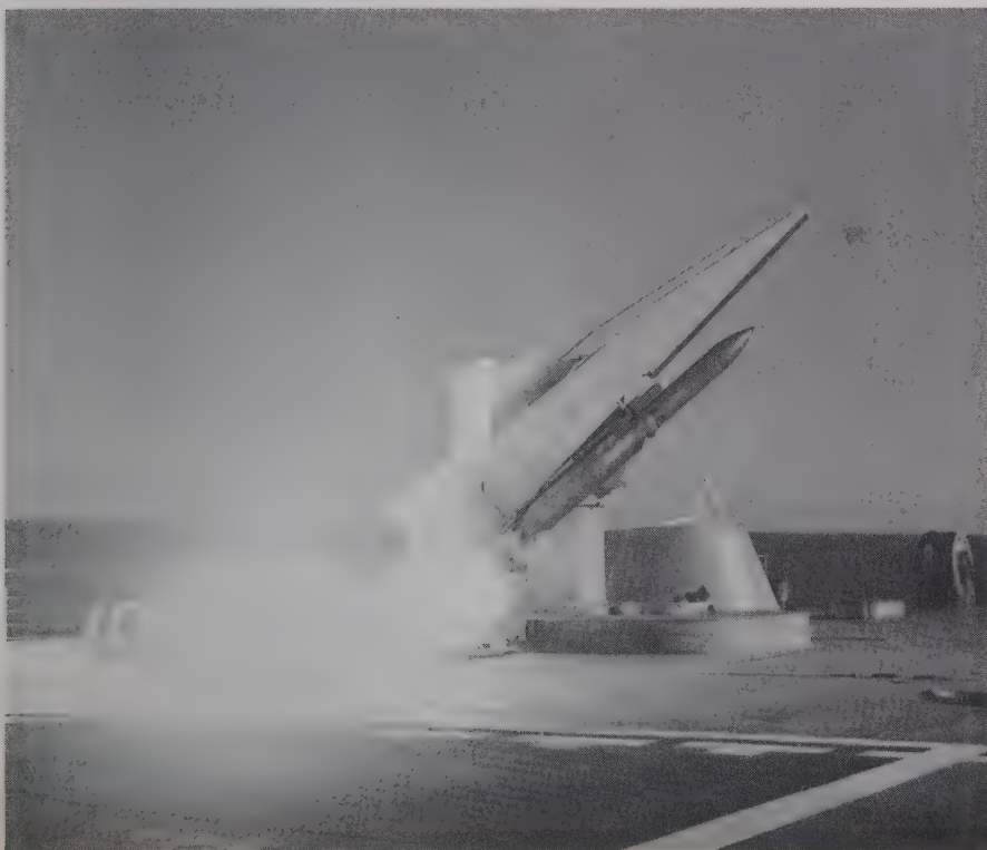
1 THE MISSILE LAUNCHING SYSTEM MARK 10 MOD 7 (ASROC)
