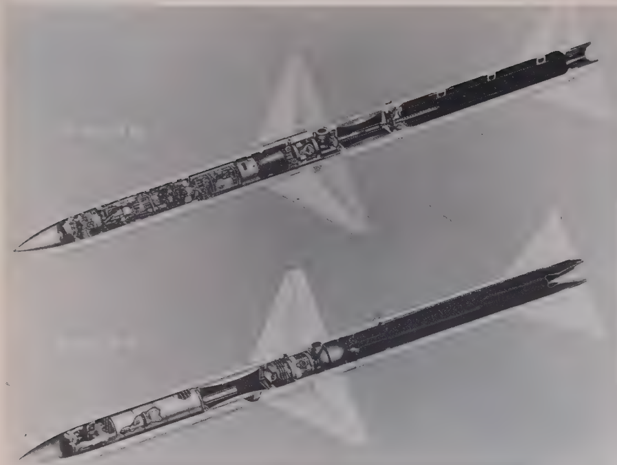
Although most Sparrows appear identical externally, the series has seen very considerable evolution. This 1973 sketch compares AIM-7E with -7F, the latter having a much larger rocket engine and far more compact electronics, permitting movement of the warhead forward of the wings.
