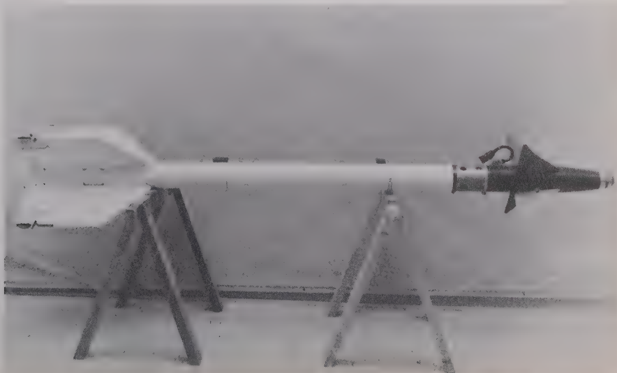
AIM-9L is the current version of the Sidewinder, with an IR seeker sensitive enough for all-aspect attacks and a longer-range rocket motor.
