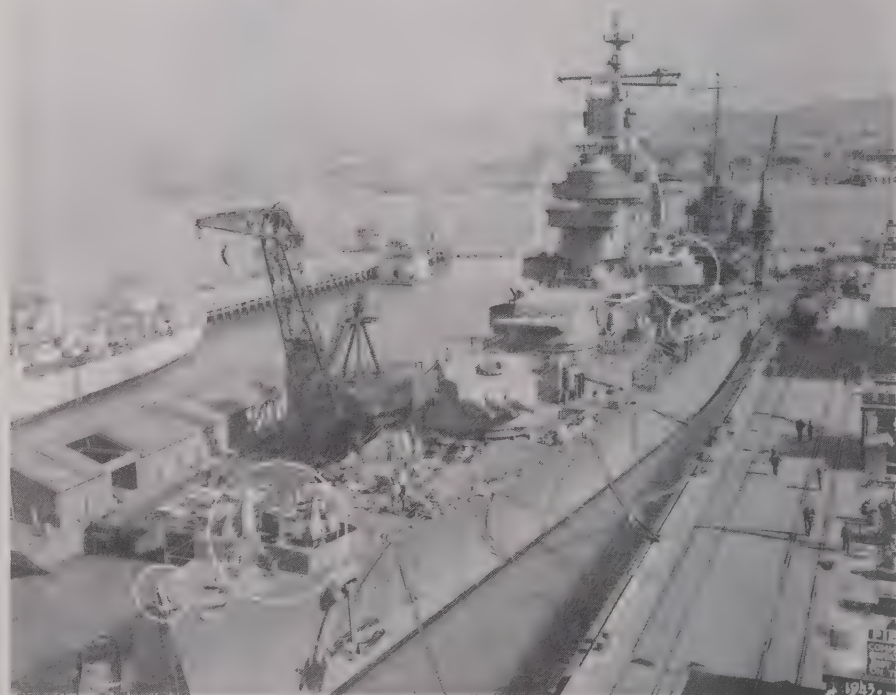
2 The cruiser Portland , refitting at Cockatoo Dockyard, Sydney, Australia, in 1942 shows typical US triple 8in turrets, all three guns clearly in the same sleeve. Shutters to either side of the guns cover pointer's and trainer's sights, and each turret carries an armored rangefinder. Fire control was by the Mk 27 director at the foretop, surmounted in this case by a Mk 3 radar, and with splinter shields for 20mm guns surrounding its base. Below and to either side are Mk 33 anti-aircraft directors to control the 5in/25 battery, each topped by a Mk 4 radar. Also visible are two antine measures: degaussing cables along the hull, passing just above the number '33' and then aft; and chains for paravanes, suspended from the eyes of the ship. The two search radars above the main battery director are SC and SG (surface search), but as yet the ship has no IFF.
