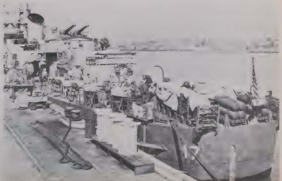
The destroyer escort Edward C. Daly , refitting at Mare Island, shows both the new teardrop-shaped Mk 9 depth charge and also the effect of roller-loading: note the stowage of arbors under each thrower, rather than under each charge. Economy of space was particularly important in a DE, with eight K-guns (rather than the four or six of a destroyer) concentrated aft.
