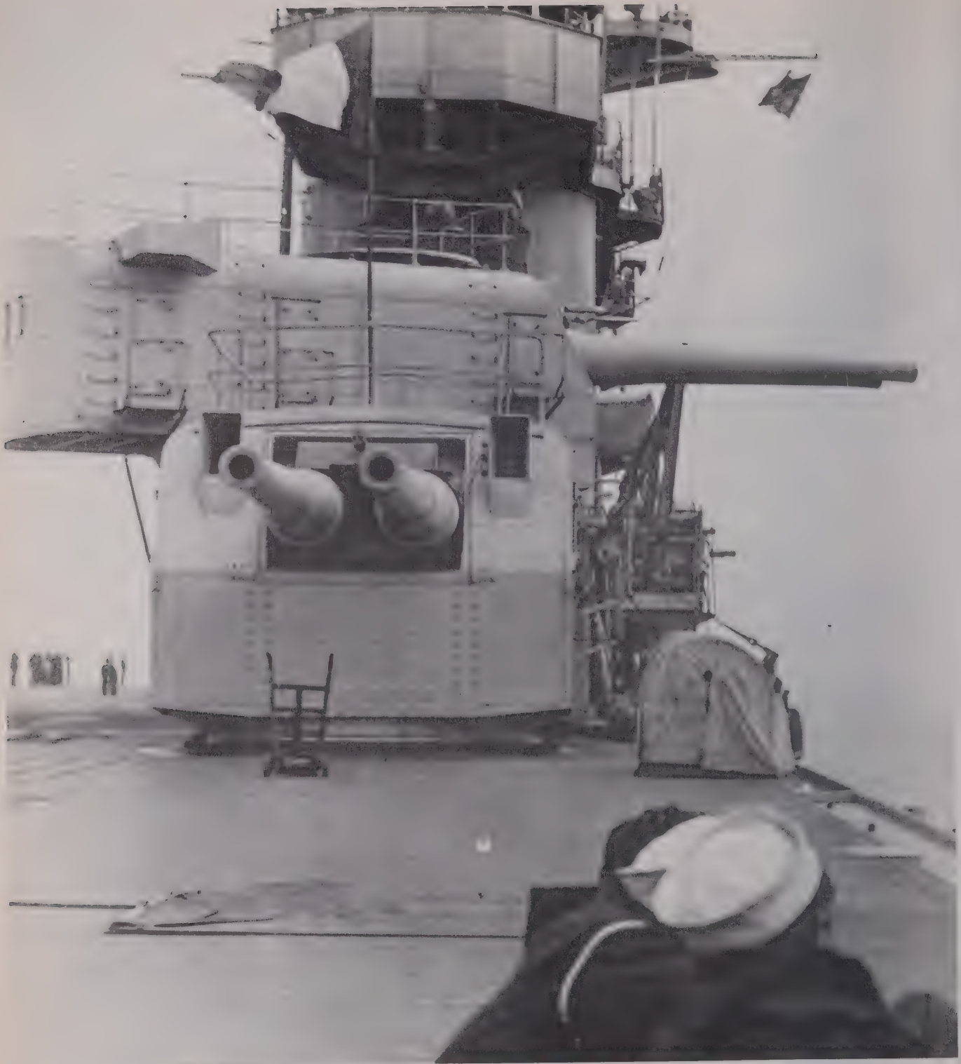
The 8in/55 No 3 mount aboard the fleet carrier Lexington during firing trials off San Pedro, 1928.
