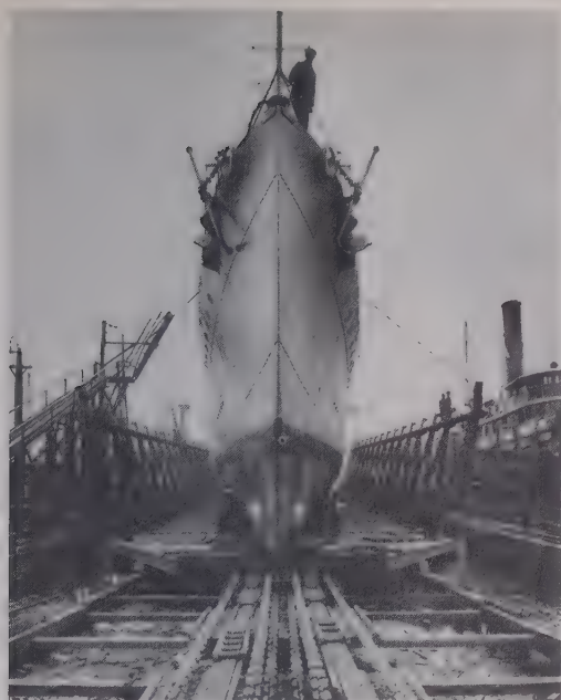
1 The destroyer Blakely shows her hydrophones in this drydock view, May 1919. They were installed in the two blisters just above her keel, visible on either side of her bow, and were aboard several US destroyers of this period. Listening at sonic (rather than the later supersonic) frequencies, they were relatively ineffective, and plans to fit all destroyers with such equipment were never implemented.
