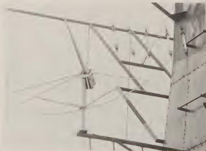
A "sword" antenna typical of those feeding the WLR-1 pulse analyzer. This is on board a British ship, but U.S. "swords" (i.e., monopoles emerging from ground planes consisting of a few wires) are identical. WLR-1 also employs higher-frequency "derby" antennas, which are analogous in design. (A. Raven)
