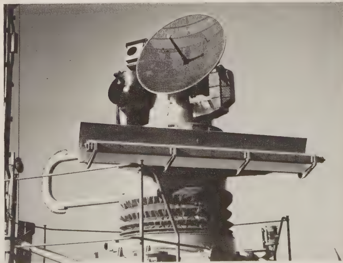
Sea Hunter 4: the upper forward stabilized mount shows the search antenna, track antenna, and Sea Killer Ku-band command antenna below the television camera. The search antenna could also be mounted separately. (Contraves)
