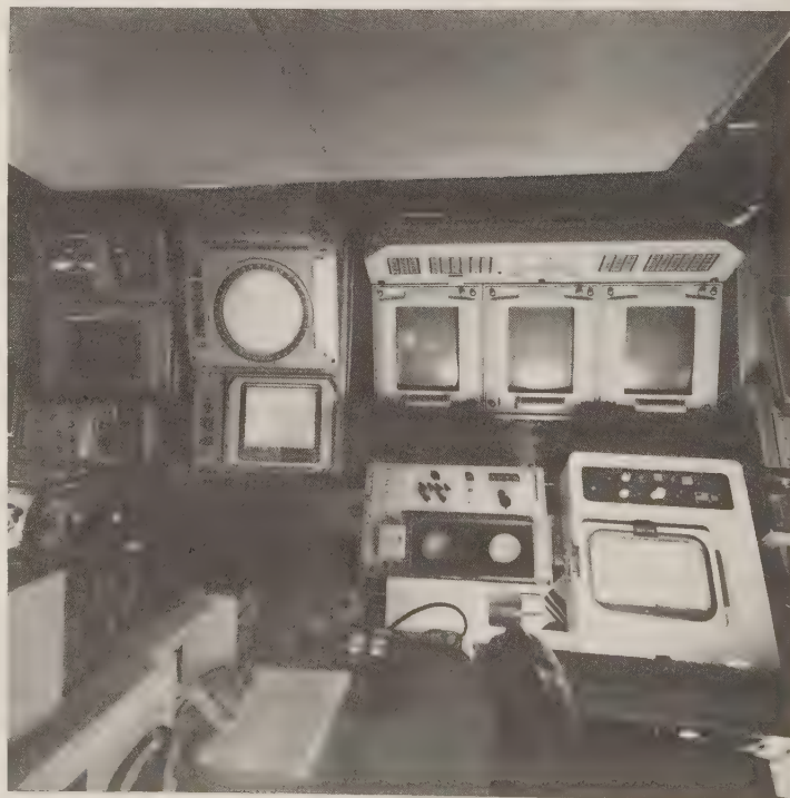
Agosta CIC, showing the torpedo FCS display (DLT), DUUX 5, and the panoramic (integrated) sonar displays. (Thomson Sintra)
