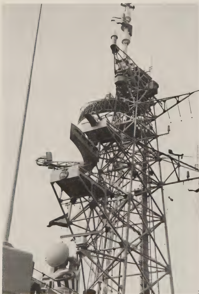
A Canadian Annapolis -class destroyer shows, top to bottom, SPS-10D (turned toward the mast), SPS-503, and Mk 127E (the slotted waveguide at bottom), with SPG-515 below atop the director. (G. Till)
