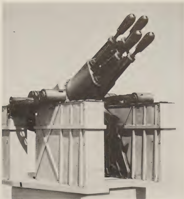
The Mauser Vierling CIWS gun. The Mauser Vierling is also now being called Taifun. First sea trials (1991) will be run with a modified Bofors L70 mounting. An entirely new mount should be ready in 1993. Meanwhile, the German navy is leasing Goalkeepers as interim replacements for the RAM missiles planned for its frigates. (Mauser)
