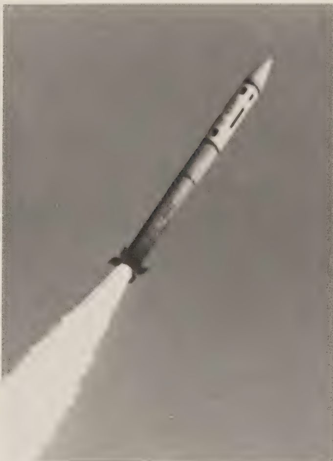
Sea Lance prototype in flight, January 1989. The payload must be shrouded (which is not the case in ASROC) because the missile is so fast. (Boeing)
