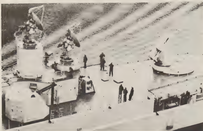
A French 57-mm/60 twin gun mount on board the missile destroyer Dupetit Thouars , 1964. The radars are U.S.-supplied SPG-51s, to control the Tartar missile shown on its launcher. (U.S. Naval Institute)
