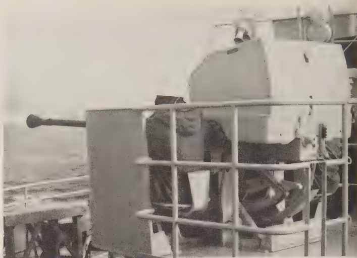
Bofors 40-mm/70 fitted with a new Trinity 99-rnd magazine, as in West German service. (Bofors)
