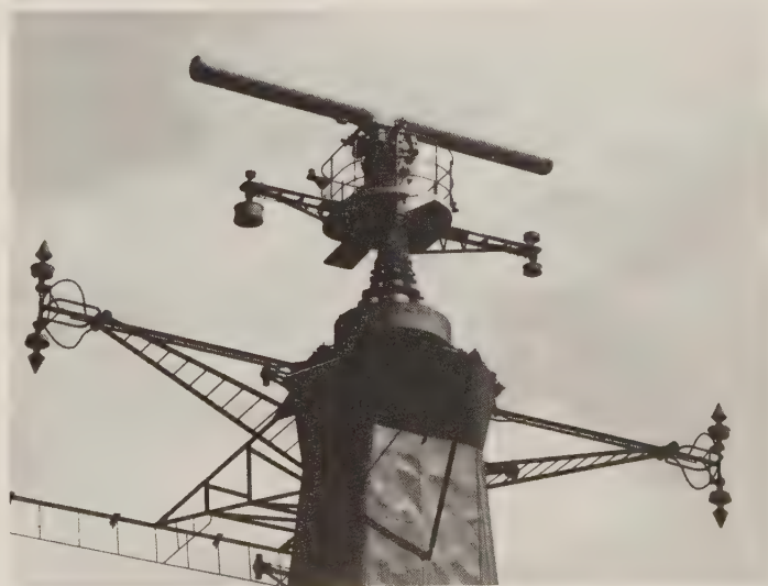
Type 992 on board HMS Ark Royal , 1990, with the UAA-1 DF array below it. The 4 small radomes at the ends of the short yards below the antenna platform are the omnidirectional antennas of UAA-1, for IFM. The "candlesticks" on the longer yards are UHF radio antennas. (Author)
