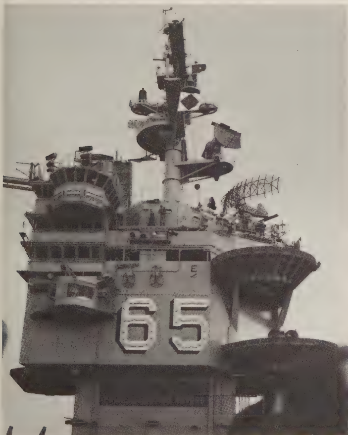
SPN-43 is the solid antenna above the larger SPS-49 on board the carrier Enterprise , 1987. The tub below SPS-49 carries SPN-42, and the 1 below that carries a Mk 91 Sea Sparrow missile director. (J. Kuersner)
