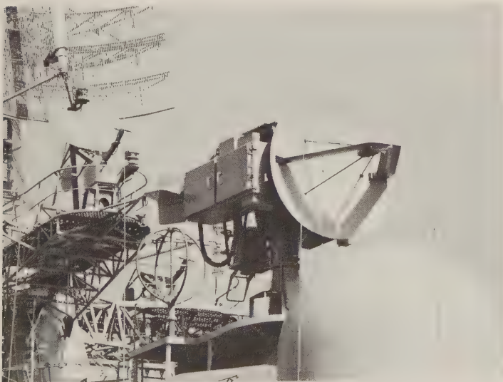
Kite Screech B radar director for 130-mm guns, on board the destroyer Otlichnyy at Norfolk, 1989. The hole is for a television camera. The radar abaft the director is Palm Frond. (S. Zaloga)
