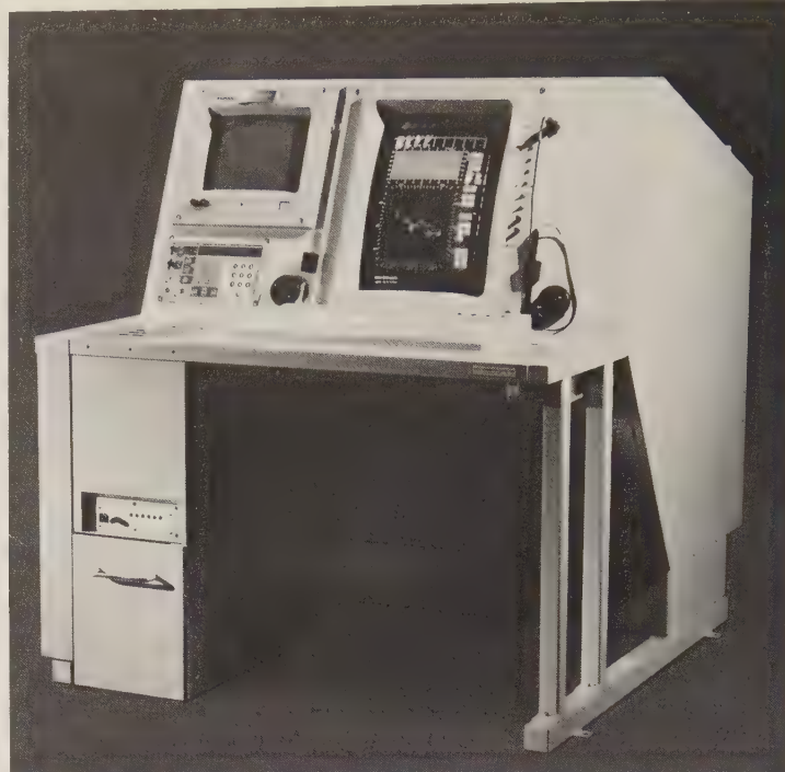
General-purpose operator station (GOS) of an M-class ( Karel Doorman -class) frigate. Several such stations are arranged side by side in the frigate's operations room. (Signaal)
