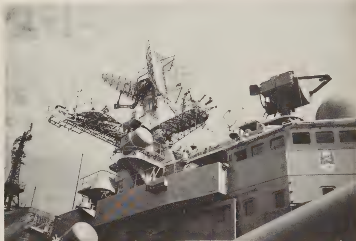
Wine Glass is the large radome visible just atop the bridge wing of the Sovremennyy -class missile destroyer Otlichnyy . The squat radome below it appears to be the upper portion of Bell Shroud; the radome on the yardarm above is Bell Squat. Other ships of this class have only Bell Shroud and Bell Squat. (S. Zaloga)
