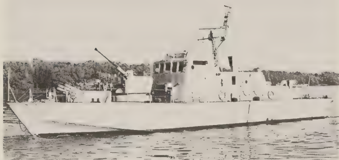
Bofors 40-mm L70 on board a Yugoslav Type-80 fast patrol boat. The launchers forward of the gun are for chaff/illumination. (U.S. Naval Institute)
