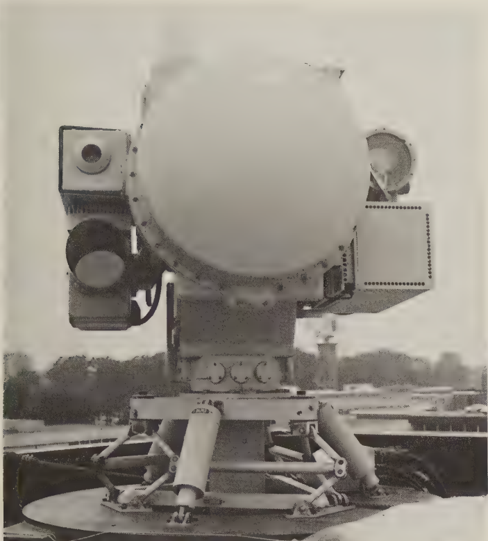
LIROD, the radar version of LIOD. (Signaal)
