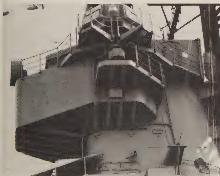
SLQ-32(V)3 on board the battleship Wisconsin , 1988. The small box under the main SLQ-32 box carries Band 1 antennas; it is usually mounted at the end of the yardarm, but this ship has no suitable location other than that at the head of the fire-control tower. (S. Terzibaschitsch)
