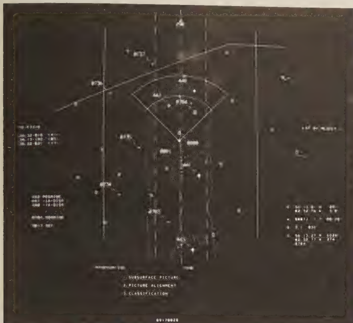
NAUTIS-M tactical display during sonar search, showing the search plan, the history of the ship's track, and sonar coverage with sonar contacts. (Plessey)
