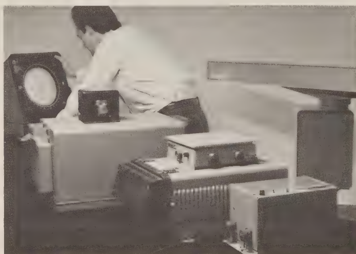
The 75-kW version of the LN-66 radar. A modified form is installed on board U.S. Navy LAMPS helicopters. (Canadian Marconi)
