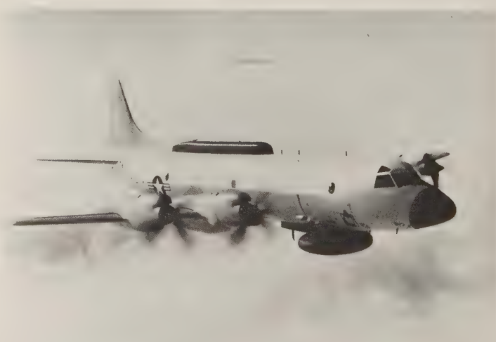
An EP-3E, showing its large belly radome. Japan is reportedly converting 4 P-3Cs to a similar configuration, for naval surveillance. (Lockheed Aeronautical Systems Co.)
