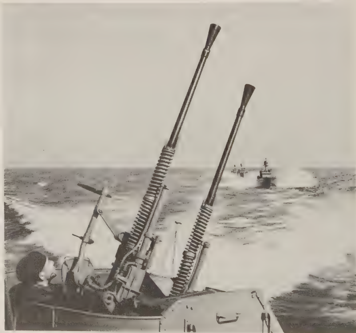
Twin 25-mm anti-aircraft guns on board a P-6-type motor torpedo boat, about 1962. (TASS from SOVFOTO)
