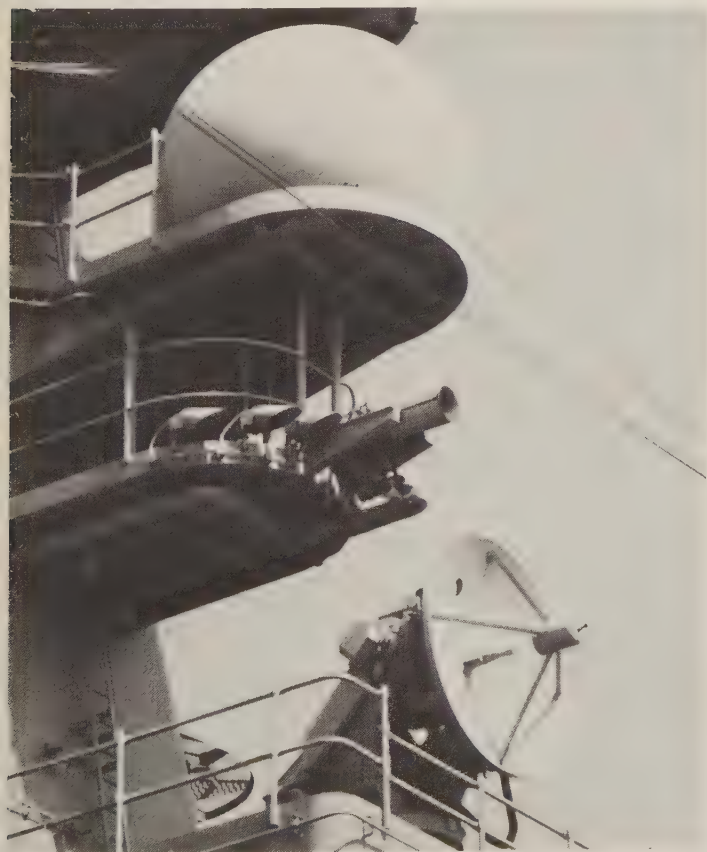
The 2 radars of the Mk 86 GFCS on board the USS Mississippi , June 1988: radome-enclosed SPQ-9A above, SPG-60 below. The hole in the SPG-60 antenna is for the television tracker. (Stefan Terzibaschitsch)
