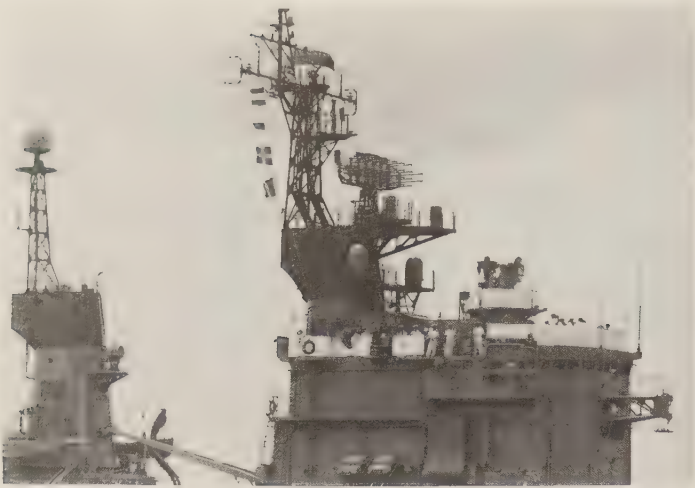
OPS-11 on board a Takatsuki -class destroyer, with OPS-17 surface-search radar above, and GFCS-1 atop the bridge. The big radomes are part of a jamming system called OLT-3; the small ones are probably DF radomes (NOLR-6). (Author)
