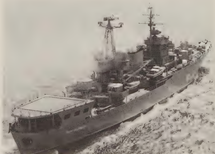
The Don-class submarine tender (floating base, in Soviet parlance) Viktor Kotel'nikov shows her 2 Big Ball satellite communications antennas, a type of equipment formerly carried by now-defunct Sverdlov -class command cruisers. The lattice mainmast carries the Slim Net air-search radar and 2 Square Head IFF interrogators.
