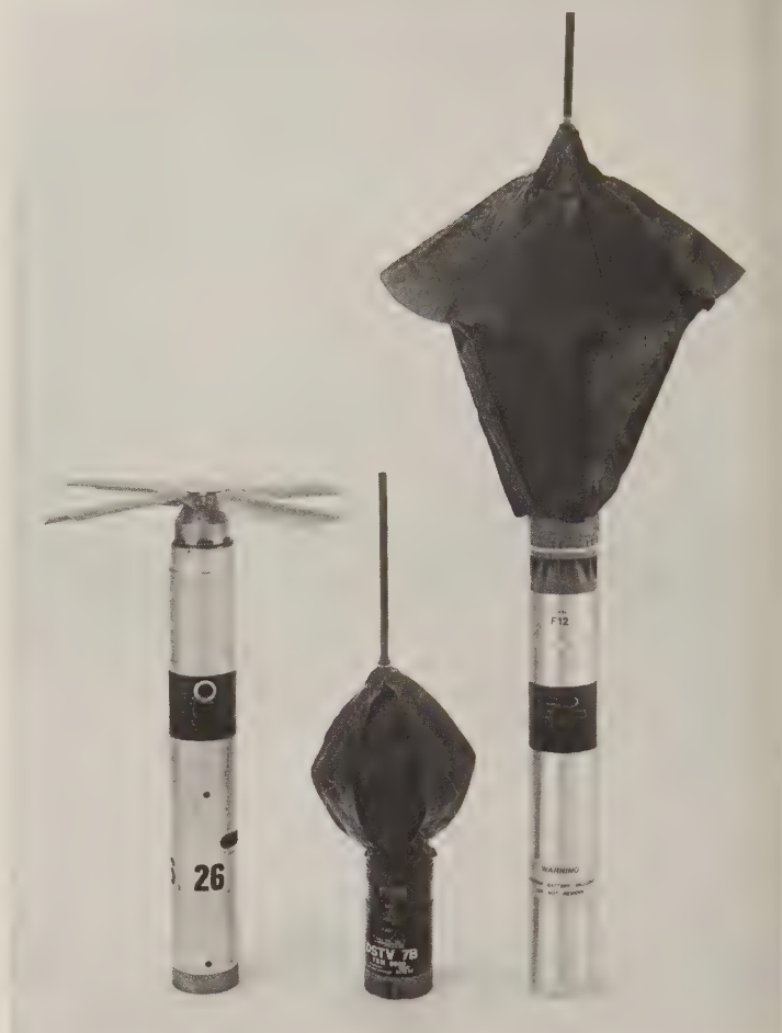
Standard French sonobuoys: DSTV-4M at left, the A/3-size DSTV-7B in the middle, and a range-only active buoy at right. The buoy on the left shows the rotochute that slows its descent. The other 2 show the inflated floats that keep their radio antennas above the surface. (Thomson Sintra)
