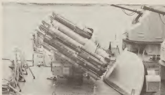
The French version of the Bofors 375-mm rocket launcher. The flare-launching racks are alongside the rocket tubes. The guns are twin 57-mm/60s, also a French version of a Bofors original. (L. van Ginderen)
