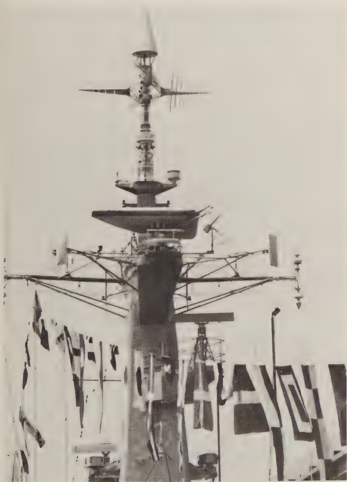
A Leander -class frigate shows a Type 1006 surface-search radar (the slotted waveguide) below her Type 994 "quarter cheese" short-range air/surface-search antenna. The masthead array is UA-13, and below it are UA-8 and -9. The "sword" on the right just below Type 994 is a standard Anglo-American intercept antenna. This photograph was taken in 1986. [Author]
