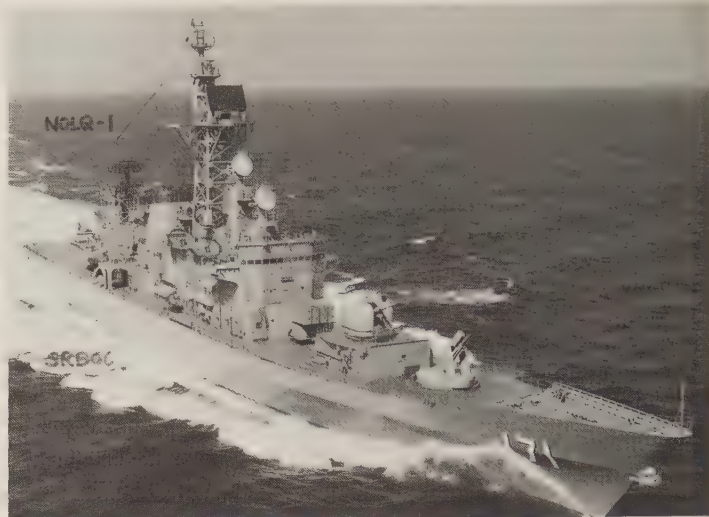
EW systems of the missile destroyer Hatakaze . NOLQ-1 combines the masthead array, the antenna just forward of the main air-search radar (SPS-52C), and the flat array at the base of the big lattice mast. The 2D radar aft is OPS-11C, and the slotted array at the masthead is the OPS-28B anti-sea-skimmer set. (JMSDF)
