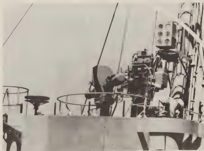
Mk 52 gunfire-control system with Mk 26 range-only radar, on board a destroyer escort. (Naval Historical Center)
