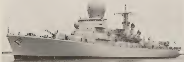
SPS-01 occupies the large radome of the Dutch destroyer Tromp . The small radome forward of the bridge is for a Signaal WM-25, and 2 SPG-51s aft control the Standard Missile. The 2 slotted-waveguide surface-search radars are Decca 1226s. (U.S. Naval Institute)
