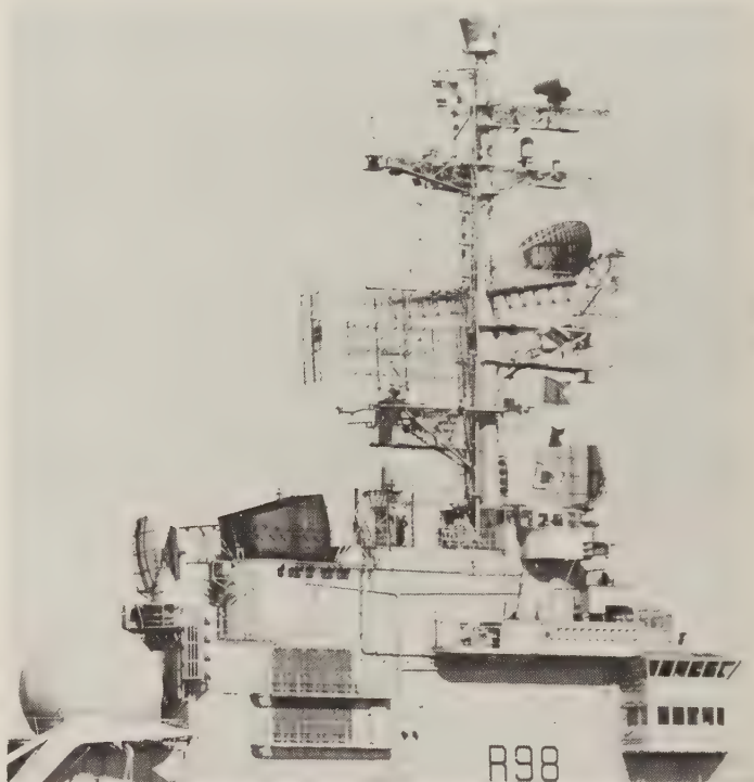
The French carrier Clemenceau , 1972, shows typical radars: from top to bottom, they are: TACAN, IFF Mk 10, DRBV 22, DRBV 20 (large-ship version), DRBI 10 (both fore and aft of the funnel). (Giorgio Arra)
