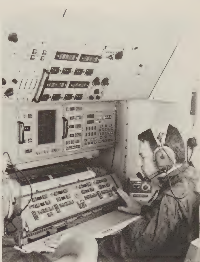
An AQA-7 sensor station on board a P-3C shows both the CRT and the multichannel hard-copy recorder below it. The CRT is fed by a computer memory; operators can switch among buoys or among narrow bands without losing the data on the other buoys or the other bands. The hard-copy recorder, however, has no memory beyond what is on the paper, so it is very limited in the number of channels it can handle. (U.S. Navy)
