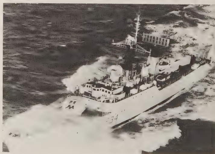
HMS Puma , a Type 41 anti-aircraft frigate, shows her Mk 6 director with its Type 275 fire-control radar (just abaft her bridge). The gun mount forward is a 4.5-in Mk 6. Two sisters survive in the Bangladesh Navy. (HMS Excellent )
