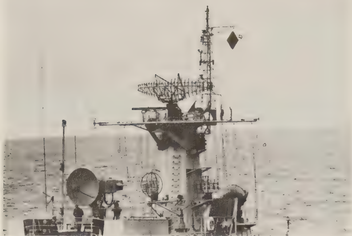
Strut Curve air-search radar on board an East German Koni-class frigate, 1978. (U.S. Naval Institute)
