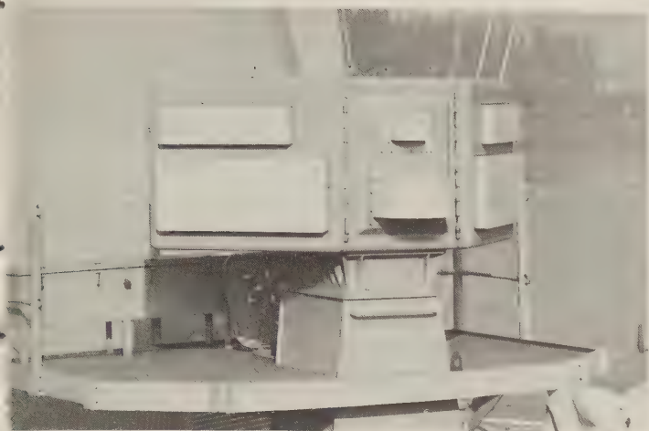
SLQ-32(V)2, USS William S. Sims , 1986. The upper antennas cover Band 3, the lower (larger) ones Band 2. The flat plates cover the DF lenses; the semicircular radomes cover semi-omni antennas. The system also includes Band 1 quadrant antennas at the yardarms. The simpler (V)1 version is limited to the Band 3 antennas but uses the same box as (V)2. (L. van Ginderen)
