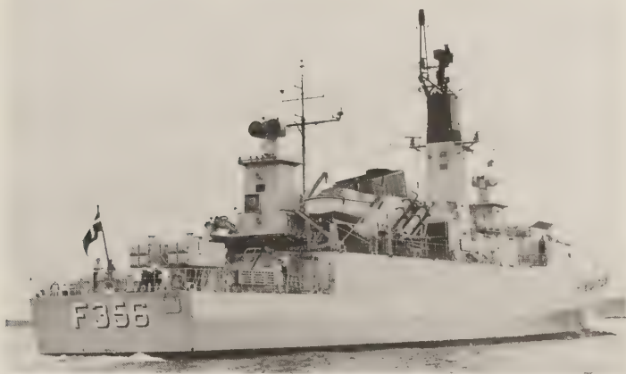
AWS-5 at the foremasthead of the Danish frigate Peter Tordenskjold , with a NATO Sea Sparrow fire-control radar (Mk 91) aft. The 2 slotted waveguides are probably Decca TM 1229s (Skanter 009). (L. Van Ginderen)
