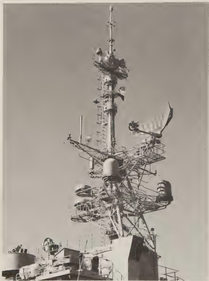
Janet jammer on the foremast of a Saudi Al Madinah -class frigate (the 2 round radomes on the left, one above the other). The wire arrays near the masthead are for a Telegon VI HF/DF. The collars below them are a pair of standard French navy mast UFH antennas (AN 192). The big rounded radomes conceal Otomat control antennas. The radar visible is Sea Tiger. The DAGAIE decoy launcher (without its "suitcases") is on the platform below the top of the superstructure. (Thomson-CSF)
