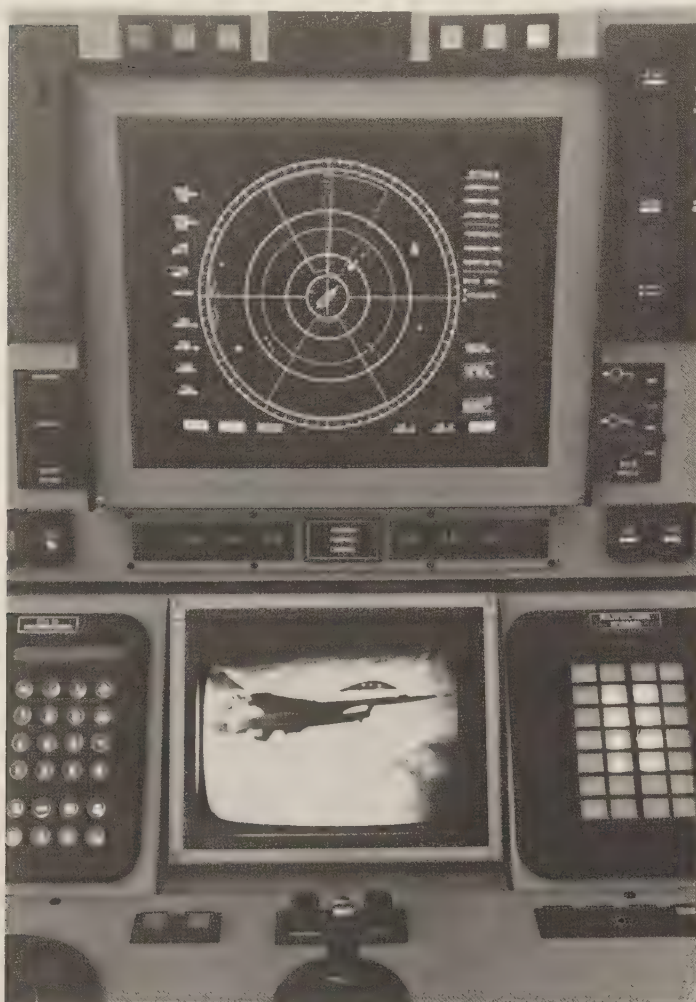
NA-18 optronic fire-control console, showing a combination of synthetic video on the upper screen and a television image below. (Selenia)
