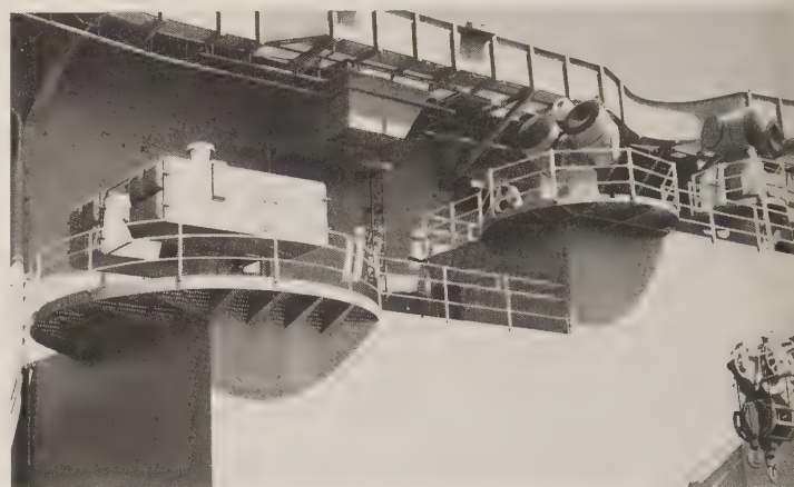
NATO Sea Sparrow launchers and Mk 91 illuminators (radar Mk 95) on board the carrier USS Ranger , July 1986. An electro-optical tracker is located between the 2 radomes of the radar illuminator-tracker. (Hughes)
