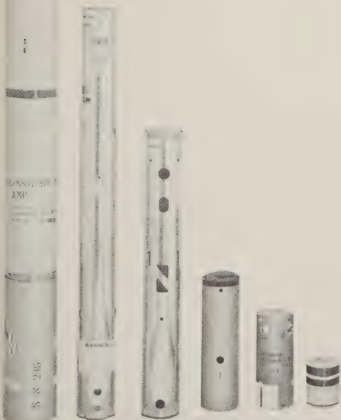
B-size Stretch A A-size G-size F-size A/6 The range of sonobuoy sizes. (Sparton)
