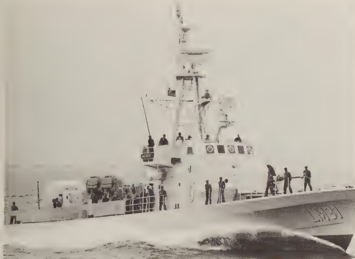
The Ecuadorian missile boat Quito has a Triton air/surface-search radar on her mast (with an ESM array above it), and a Pollux fire-control radar. The mast platform just aft of the Pollux dish carries a Decca 1229, barely visible because its antenna is end-on to the camera. (U.S. Naval Institute)
