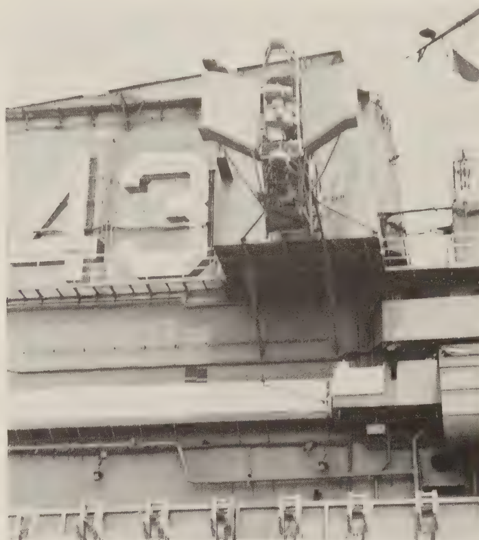
ULQ-6 on board the carrier Coral Sea at Norfolk, 1986, with the array trained. The middle portion of the antenna is SLA-12 or -15. (S. Terzi-baschitsch)
