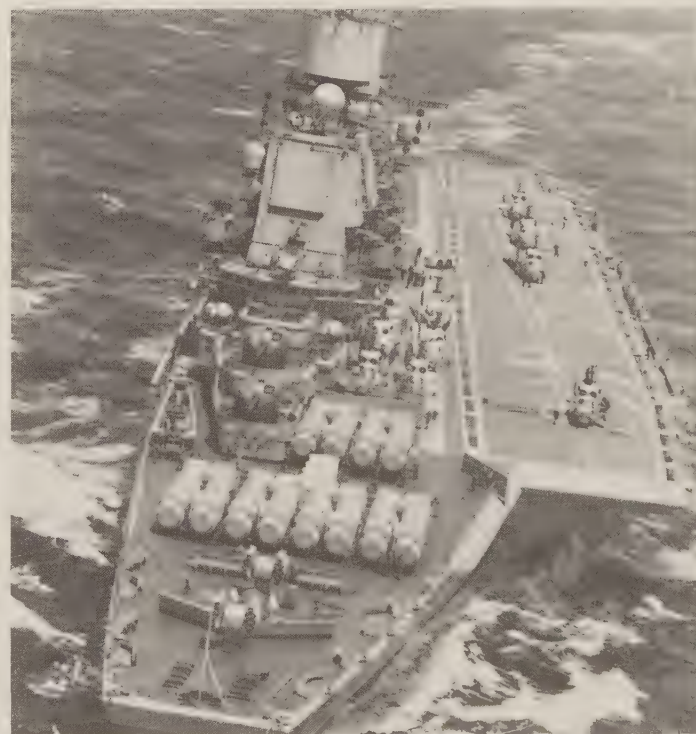
The carrier Baku introduced a new RBU launcher, seen here. The cylindrical vertical launchers immediately abaft the breakwater are for SA-N-9, and the big tubes are for SS-N-12. (U.S. Naval Institute)
