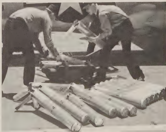
Standard A-size sonobuoys being loaded. The vanes protruding from their heads are rotochutes, which slow the buoys as they descend. (U.S. Navy)
