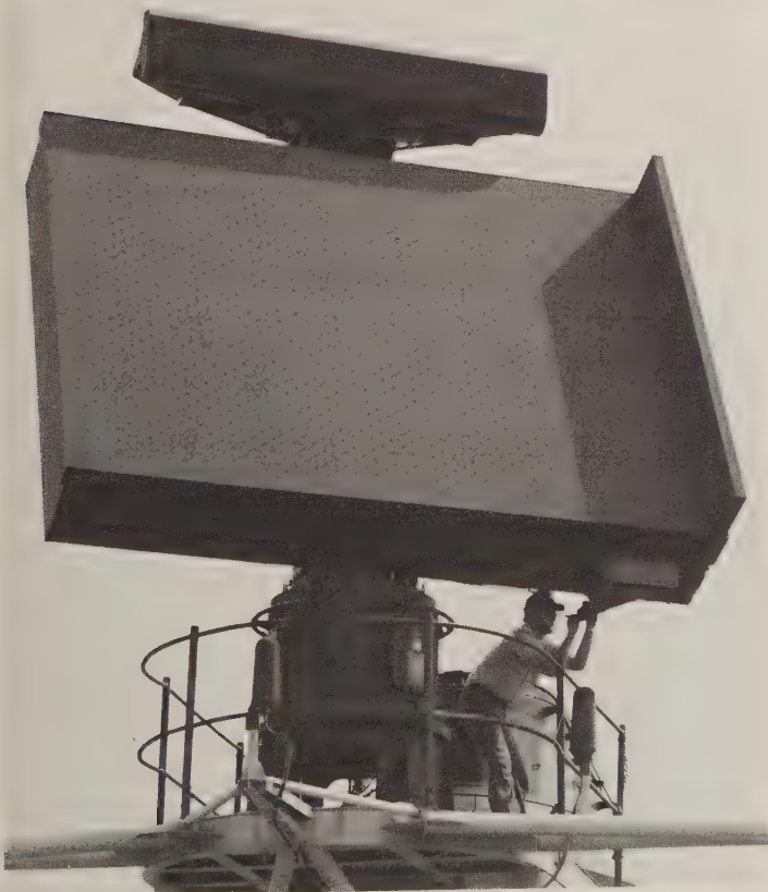
An SPS-52C antenna, on board USS Tattnall (DDG 19), the first ship so fitted. The bar above is an IFF interrogator. (Hughes)
