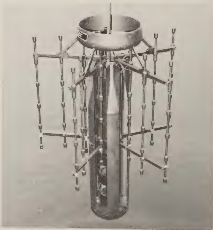
Cormorant (PMS 122) lightweight dipping sonar, with its transducer array extended. (Plessey)
