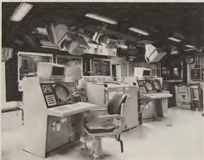
The combat information center (CIC) of the newly completed frigate Curtis shows 2 standard OJ-194/UYA-4 consoles flanking the TAO (summary) console (OJ-197/UYA-4), with an SPA-25 radar repeater in the background. Not visible between the 2 status boards behind the consoles is a large backup vertical (manual) plot. The trackball of the console in the foreground has not yet been installed, but one is visible on the console on the right. (U.S. Navy)
