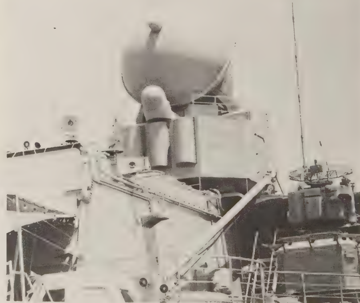
Top Dome missile-guidance radar on board the Soviet Slava -class missile cruiser Marshal Ustinov at Norfolk, 1989. (D. Steigman and S. Zaloga)
