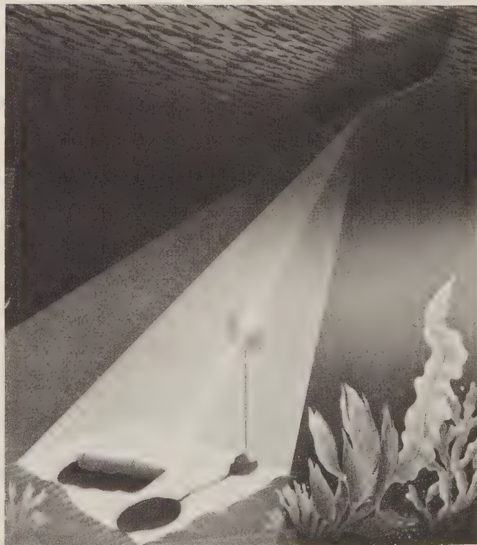
IBIS V minehunting system shows the shadowing effect of mines illuminated by an overhead sonar. (Thomson Sintra)
