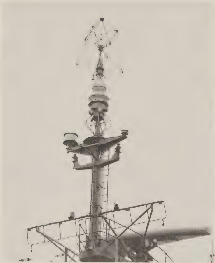
A standard FH-series (in this case serving FH 12) HF/DF array at the foretop of a Leander -class frigate, 1988. Below the "bird cage" array are omnidirectional antennas and 4 antennas for DF, with omnidirectional antennas (for IFMs) on the crosstree below them. They serve UA-8/9. (A. Raven)
