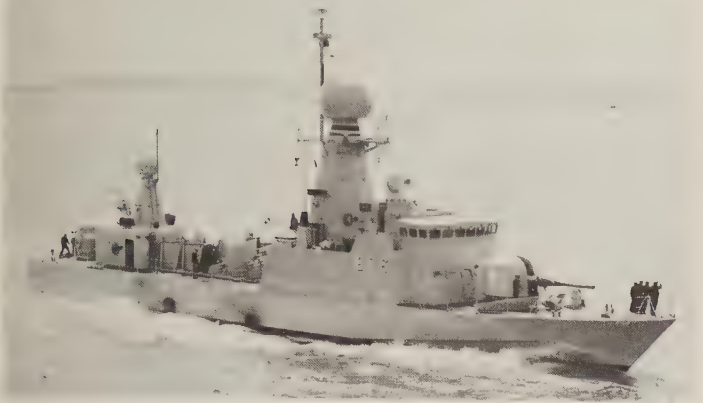
The Egyptian patrol boat El Yarmouk shows a Marconi S1810 radar in a radome on her foremast and a Cygnus jammer in the smaller radome on her mainmast. At her fore masthead she carries Cutlass and Matilda ESM, and she also carries 2 Protean chaff mortars. (L. Van Ginderen)
