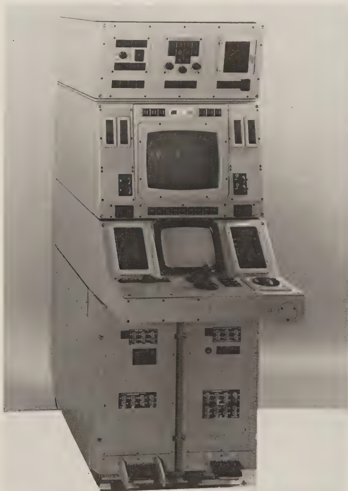
NA-18's display-and-control console, for one-person operation. (Selenia)
