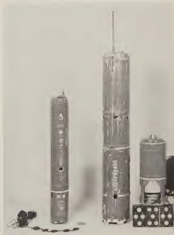
BM-1 (left) and BM-2 (right) sonobuoys, with BM-1 hydrophone at lower left and BM-2 array at lower right. (U.S. Navy)
