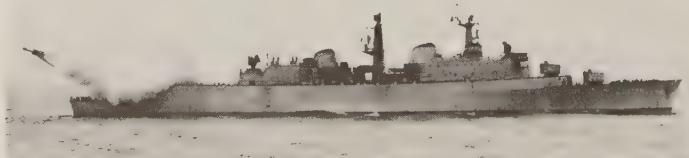
HMS Devonshire fires a Sea Slug. The cylindrical radar just forward of the helicopter platform is Type 901; forward of the after funnel are the Type 278 height-finder and the Type 965 (AKE-1 antenna) search radar. (U.S. Naval Institute)
