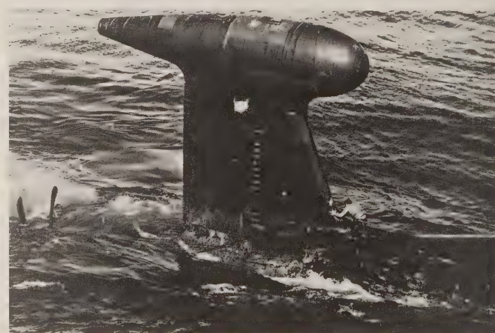
A Soviet Victor-III-class submarine displays her towed array pod atop her vertical fin. This particular submarine had fouled the towing cable of a U.S. towed array, and her crew was trying to break the cable. The submarine was trimmed down by the bow, so her unusual double propeller (two 4-bladed propellers in tandem, turning together) is visible. This type of propeller was adopted by many early steam-torpedo and destroyer builders as a way of transmitting considerable power without cavitation and without accepting unduly large propellers. The scale of the pod and fin are clear from the figure of the Soviet crewman trying to cut the cable. This photograph was taken in the fall of 1983. [U.S. Navy]
