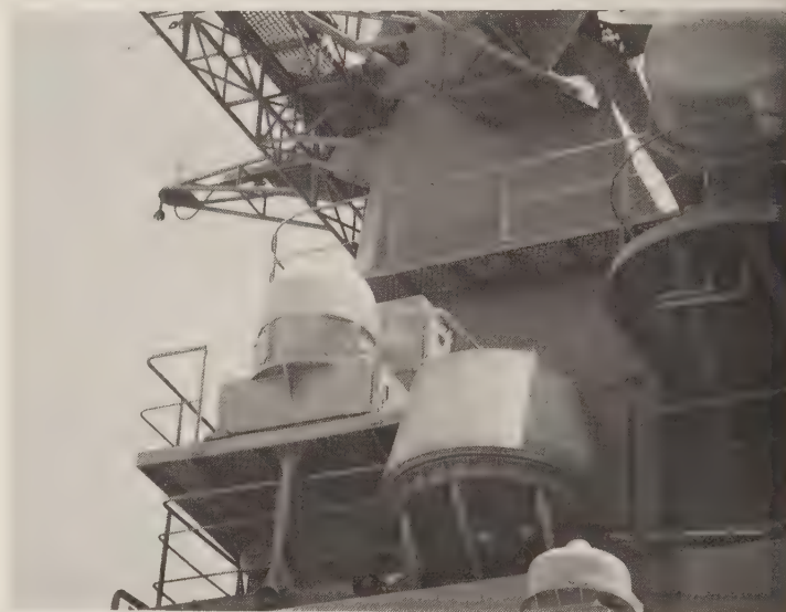
The Sovremennyy -class destroyer Boevoy shows a Wine Glass jammer with, below it, the 2 components of Bell Shroud. In most ships the small radome, with its bulb, is mounted above the large shroud. (S. Zaloga)
