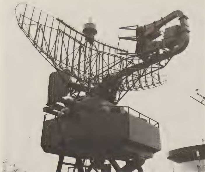
LW-08 on board a van Heemskerck -class missile frigate. This version has a double feed; there is also a single-feed version. (Signaal)
