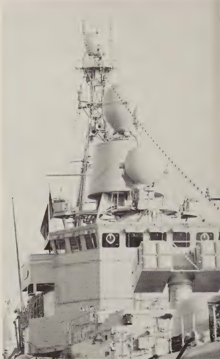
FL1800S on board the German frigate Karlsruhe , 1990. The omni antenna (for IFM) is carried between the STIR antenna and the Signaal "egg," and the usual pair of jammers is visible just above the bridge windows. The DF array is in the masthead radome. (G. Arra via Ships of the World )
