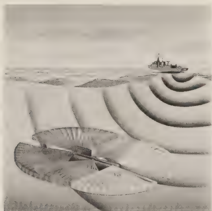
The overlapping preformed beams of PRS 3-15. (KAE)
