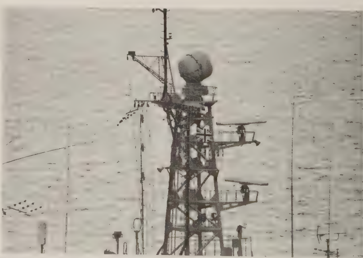
Drum Tilt radar at the masthead of the former East German training ship Wilhelm Pieck , which was visiting London in 1990. The slotted arrays are the standard TSR-333 used on board many East German warships. (B. Sullivan)
