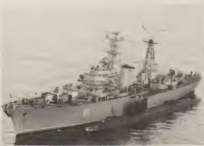
The Don-class submarine tender Dmitriy Galkin shows the standard Soviet Vee Cone long-range HF antenna on her lattice mainmast. The angle between the cones can be varied, and the sides of the cones are solid in some ships. The weapons and sensors date from the 1950s and 1960s—100-mm guns in open mounts, a Wasp Head main-battery director with a Sun Visor radar, and 2 Hawk Screech secondary fire-control radars.
