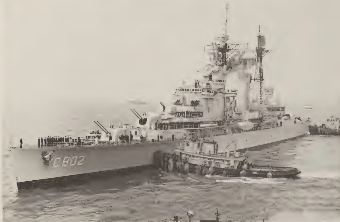
The Dutch cruiser de Ruyter (now Peruvian) shows both the Bofors twin 6-in and twin 57-mm/60 (superfiring above the 6-in turrets) guns. (U.S. Naval Institute)
