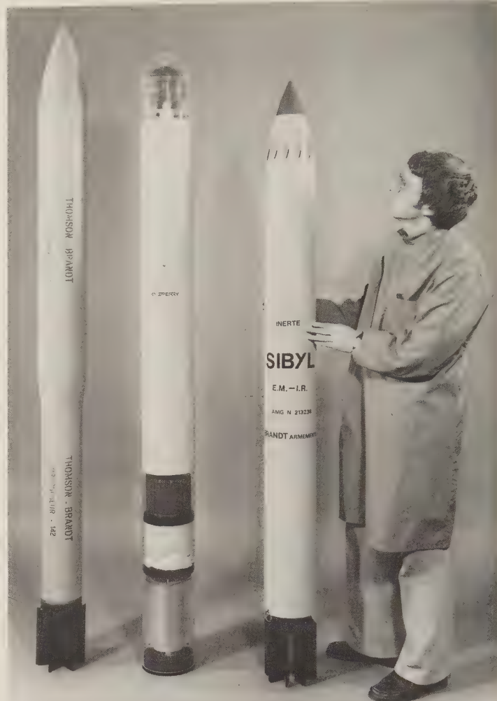
Sibyl decoy rockets, with the combined chaff/IR round on the right. (British Aerospace)
