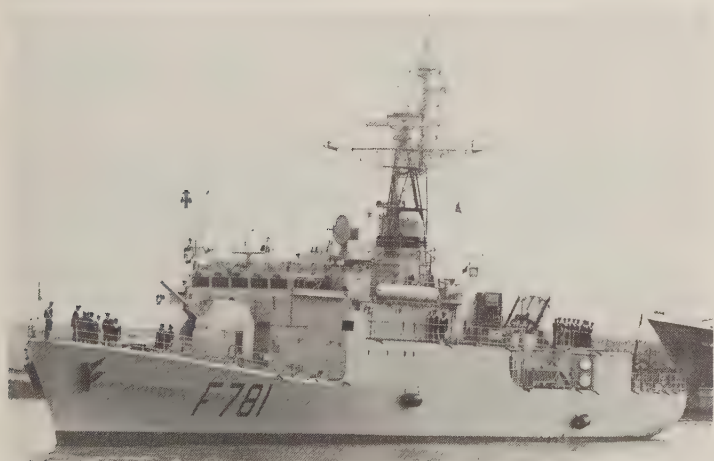
The corvette d'Estienne d'Orves shows a DRBV 51A main search radar and a DRBC 32E fire-control radar atop her superstructure. The 2 light-colored circles in the after superstructure cover 2 torpedo-firing catapults. The small slotted waveguide immediately above the bridge is DRBN 32. (U.S. Naval Institute)
