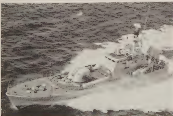
Sea Giraffe on board a Spica-II-class attack boat, at the masthead. The gun is a Bofors 57-mm/70 Mk 2. The box launchers aft carry RBS 15 missiles. (Ericsson)
