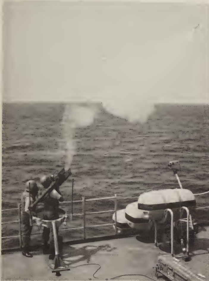
A Stinger is fired from shipboard. Note the supporting ring. (General Dynamics)
