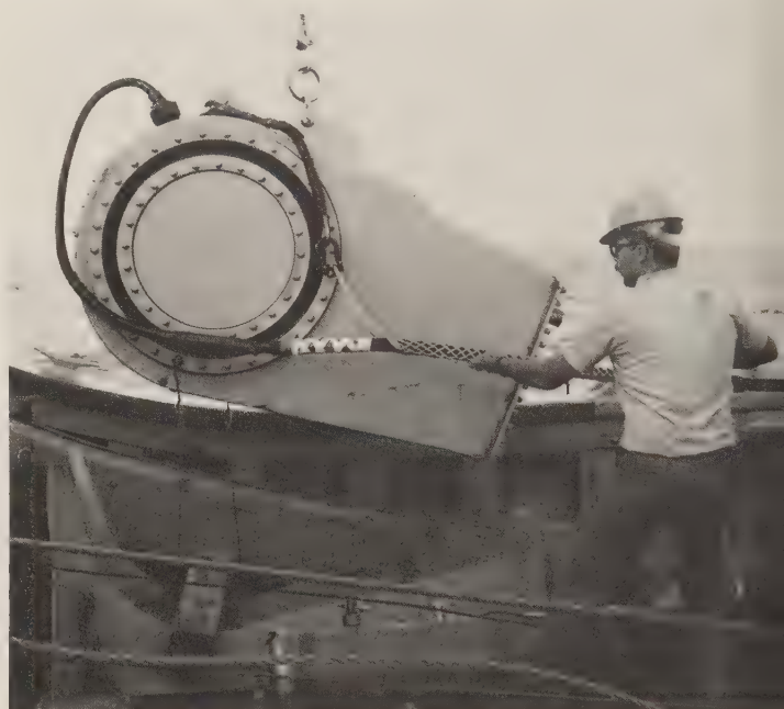
A U.S. acoustic sweep, photographed in 1987. It resembles, but is not identical to, the old A Mk 2. It is streamed suspended from an O-type float. (U.S. Navy)
