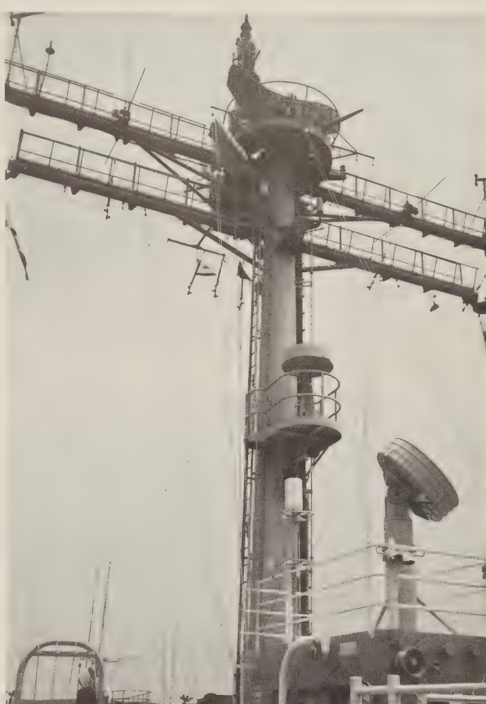
LN-66 occupies the small radome halfway up the mast of the USS Barnstable County , 1986. The masthead antenna is SPS-10, and the "washtub" in the foreground is the OE-82 satellite-communications dish. (S. Terzibaschitsch)
