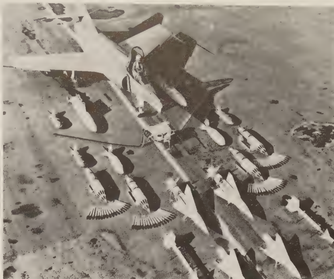
An Étendard attack fighter displays the standard French guided and unguided weapons, including the standard rocket pods and AS 30 missiles and DEFA 552A guns. (ECP Armées)
