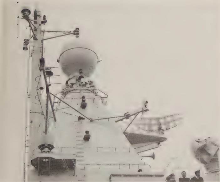
The Dutch frigate Van Kinsbergen shows a Sphinx DF array around her foremast, under the egg-shaped radome of her Signaal WM25. The mast above carries the characteristic triplet of omni antennas for the system's IFM: 1 large cylinder (foreground), 1 small cylinder with a cone above (on the yard facing away from the viewer), and (on the yard facing forward) 1 small cylinder with a smaller 1 below it. The surface-search radar is ZW-08. (L. van Ginderen)
