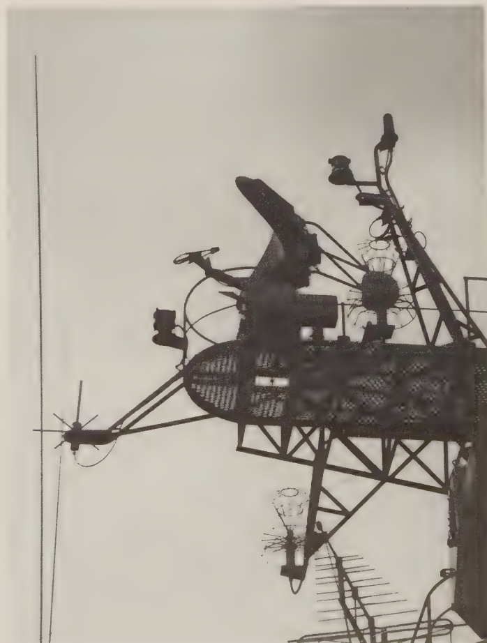
Pole Star is the array at the extreme left. The radar is Palm Frond; the original of this photo shows a set of dipoles, presumably for IFF, on its feed. (H. J. Verhoefen)
