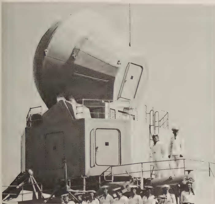
Top Dome missile-guidance radar on board the Soviet Slava -class missile cruiser Marshal Ustinov at Norfolk, 1989. (D. Steigman and S. Zaloga)
