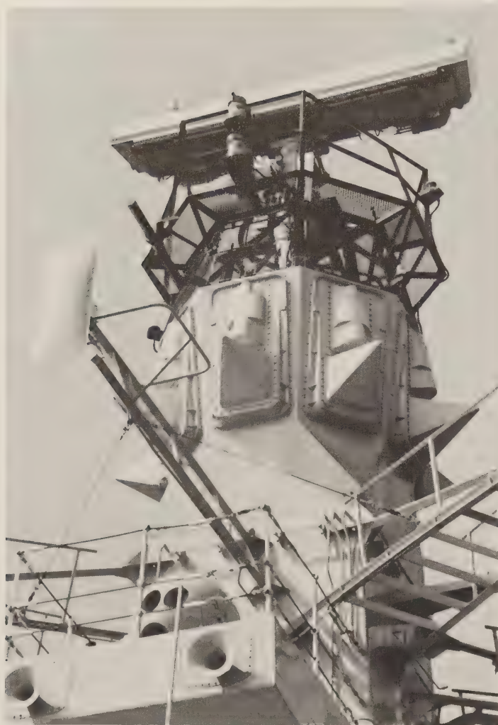
UAF-1 array at the masthead of HMS Norfolk, with Type 996 radar above, May 1990. (A. Preston)
