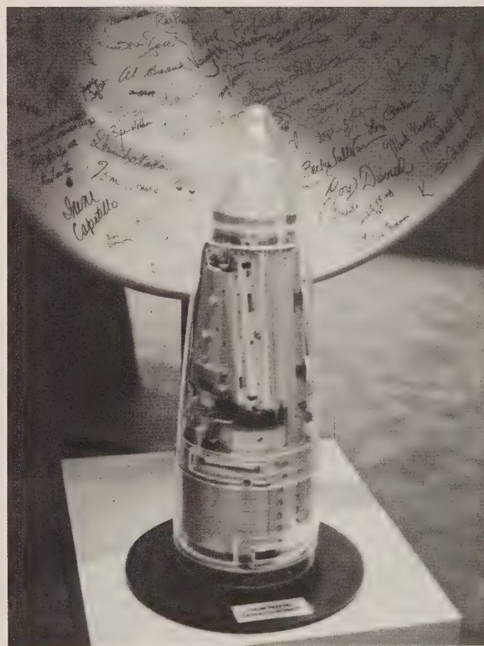
HARM Block IV seeker head, displayed by Texas Instruments at the 1991 U.S. Navy League show. The object in the background is a radar antenna through which a missile of this type had passed, signed by the members of the development team. Note the spiral antenna in the missile's nose. (Author)
