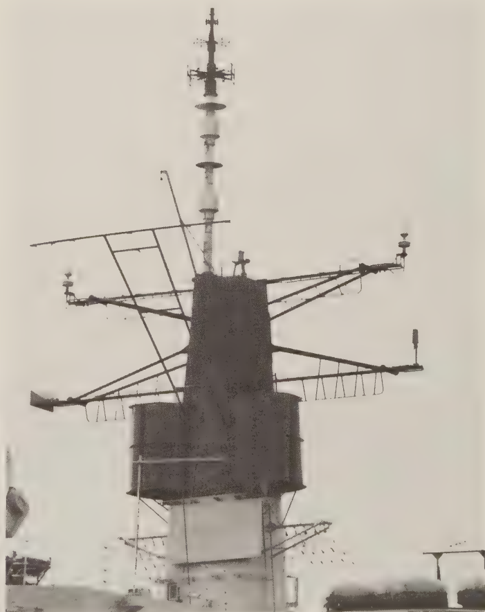
AS-3112/SRD-19 antennas, part of the Classic Outboard suite, are shown at the masthead of a British Type 22 frigate: the DF array covers the VHF range in 3 bands. The upper 2 are covered by Adcock arrays, the lower by closed loops. The entire array is 85 in high. The 2 cylindrical objects below the array are UHF receive and transmit antennas. (A. Raven)
