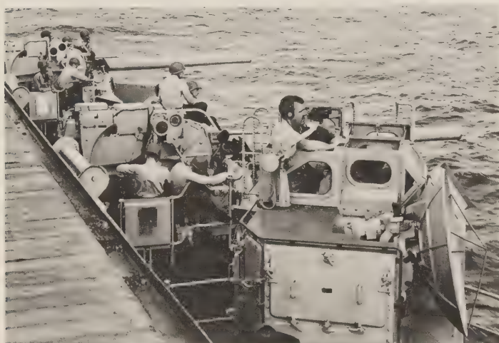
Mk 56 gunfire-control system, in this case controlling 5-in/38 guns on board a U.S. Essex -class carrier, now discarded. (U.S. Naval Institute)
