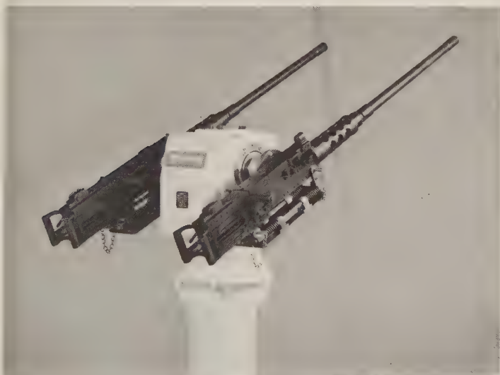
Radamec Sea Venom, a pair of remote-controlled 0.50-cal machine guns on the company's stabilized 429 servo platform. (Radamec)
