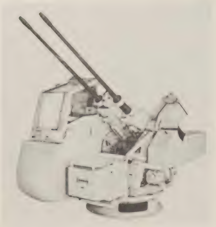
The Oerlikon 30-mm twin manned antiaircraft gun (GCM-A03-1). The A03-2 version has provision for local control (the sidecar lacks a wind-shield) but can also be remotely controlled. A03-3 is entirely remotely controlled. (Oerlikon)
