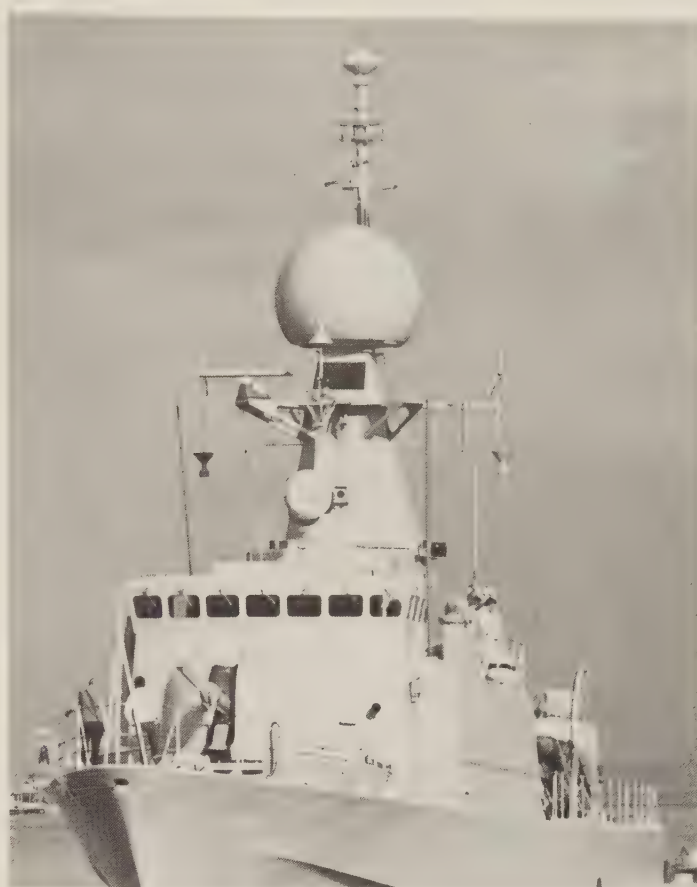
An Egyptian Ramadan -class missile patrol boat equipped with Cutlass ESM gear, visible clamped to her mast above the big radome of her Marconi S1810 radar. The masthead array is probably the AEG Telegon HF/DF. The Cygnus jammer has not yet been mounted aft. (Giorgio Arra)
