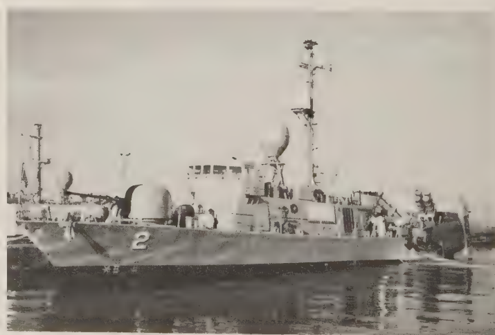
APS-137 was mounted experimentally on board the hydrofoil missile boat Hercules , to provide OTH ship identification, using ducting and the ISAR capability of the radar. It occupies the mast radome. (Texas Instruments)
