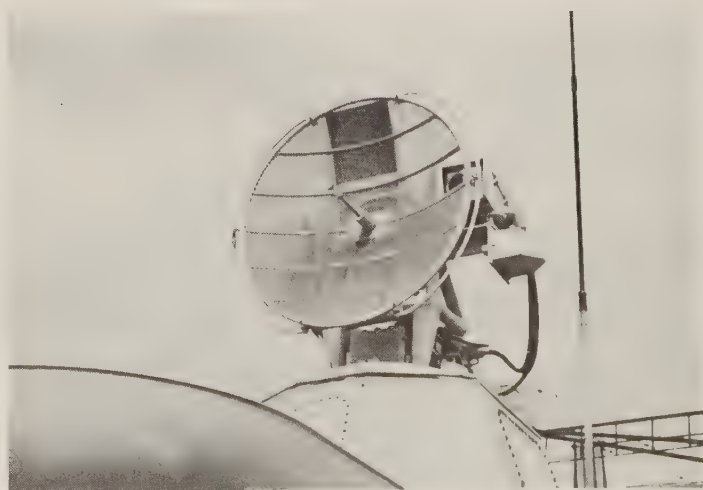
Type 912 radar director as installed on board a Type 21 frigate, with television camera visible at right. (GEC Sensors)
