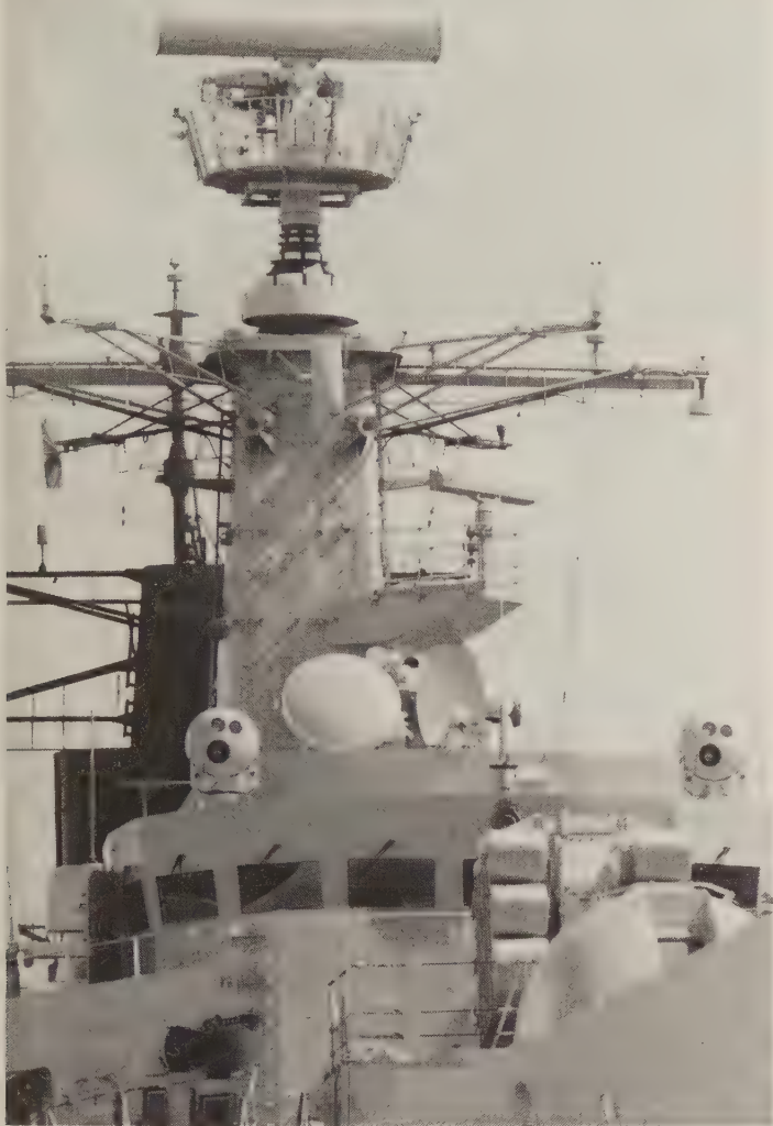
Sea Archer 30s atop the bridge of the British frigate HMS Cumberland , with a Sea Wolf director between them. (G. Arra, 1989)
