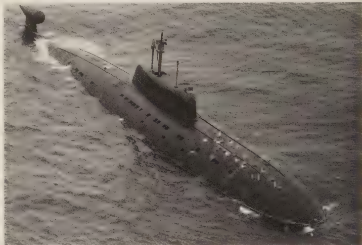
Snoop Pair (with its associated Rim Hat ESM antenna) is the second antenna from aft on this Sierra-class submarine; the cone abaft it is Pert Spring (satellite navigation). (Royal Norwegian Air Force, 1984)
