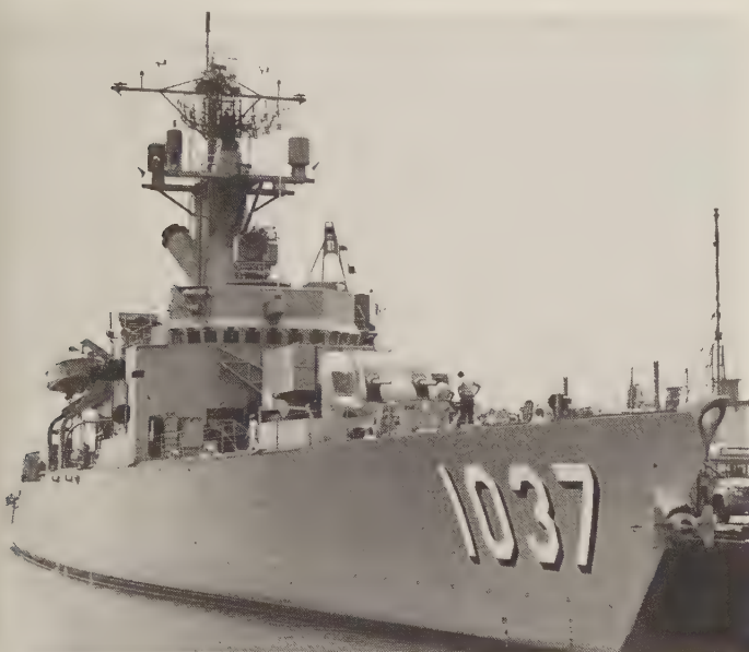
USS Bronstein shows an SPS-5C surface-search radar, above her SPS-40 air-search set. Comparison with ships carrying SPS-10 will show how much smaller the -5C's antenna is. (U.S. Navy)
