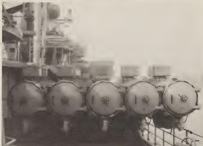
Quintuple torpedo tubes, on board the cruiser Kerch , 1989. The loading trolley is under the muzzles of the tubes. (Eric Grove)
