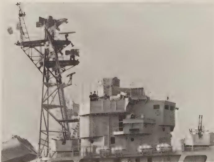
An Egyptian Jianghu -class frigate shows, on her mast, an Eye Shield air-search radar at top and a Square Tie missile target-designator 2 levels down. One of the slotted waveguides is a Decca radar; the other is a Chinese Type 756. The director carries what appears to be a yagi array (like that of the old British Type 285) on its roof. The twin 37-mm guns are locally controlled. (U.S. Naval Institute)
