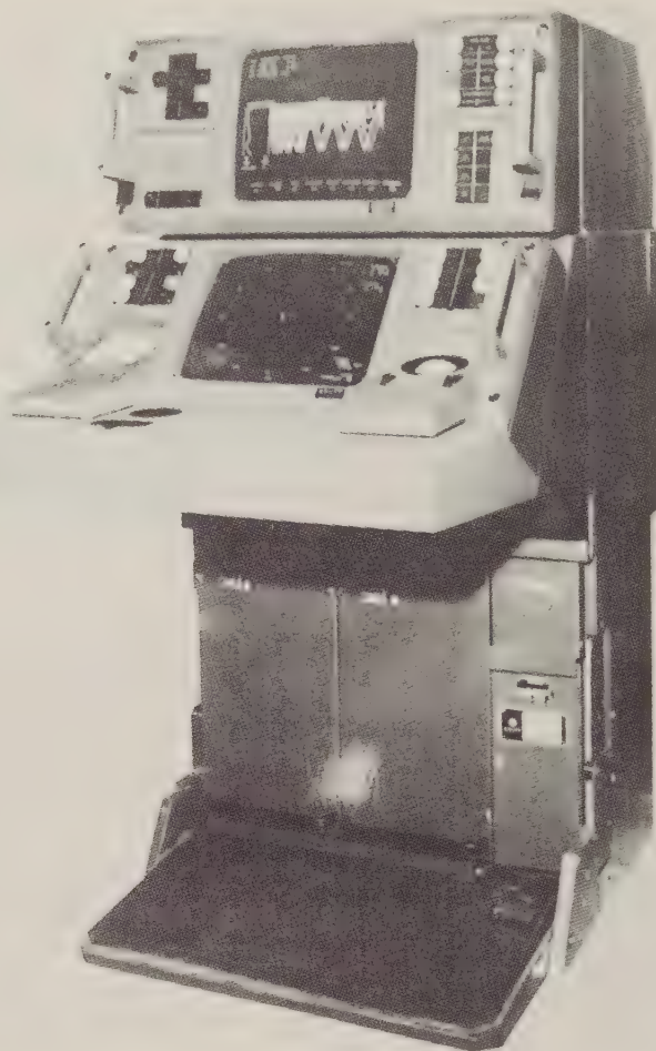
Console for a DSQS-21 sonar, showing a ray-trace indicator on the upper display and a PPI (plan position indicator) below it. (Krupp-Atlas Elektronik)
