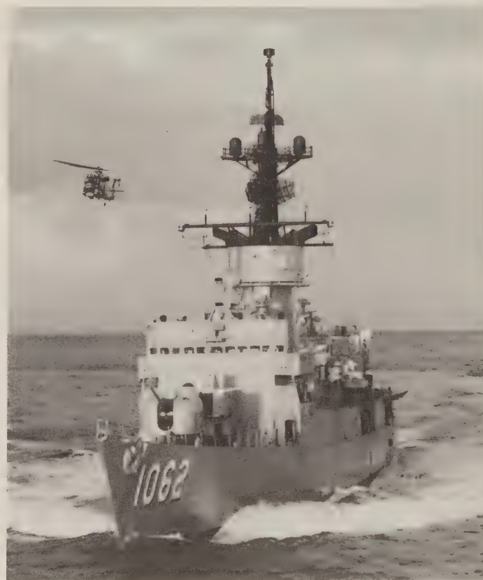
USS Whipple has an SPS-10 surface-search radar and an SPS-40. The tall antenna above the SPS-10 is her LAMPS data link. (U.S. Navy)
