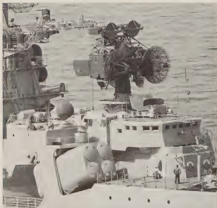
Don Kay surface-search radar is visible below and forward of the Head Lights C missile-guidance director on board the "Kresta II"-class cruiser Vasily Chapaev. The small radomes visible just abaft the missile director (1 pointed up, 1 down) are the Bell Slam and Bell Tap associated with the Side Globes ECM system. The larger radome on the centerline is Bell Clout. (Sea Power)
