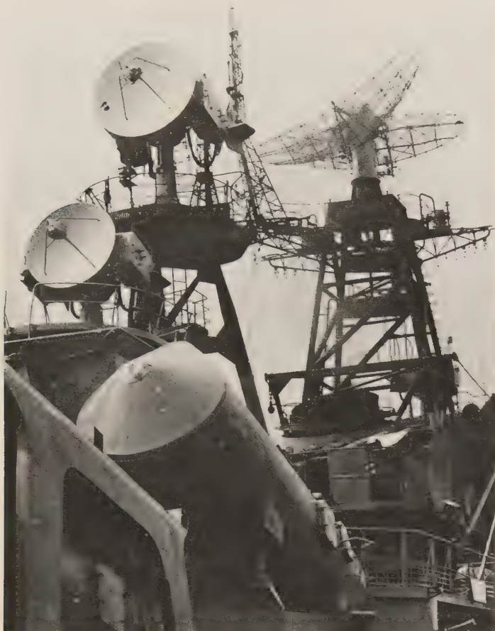
The Mod Kildin-class missile destroyer Ozorlivyy shows Owl Screech (above) and Hawk Screech (below). Owl Screech is the larger and has its feed at 45 deg to the horizontal. (Markku J. Paananen, 1979)
