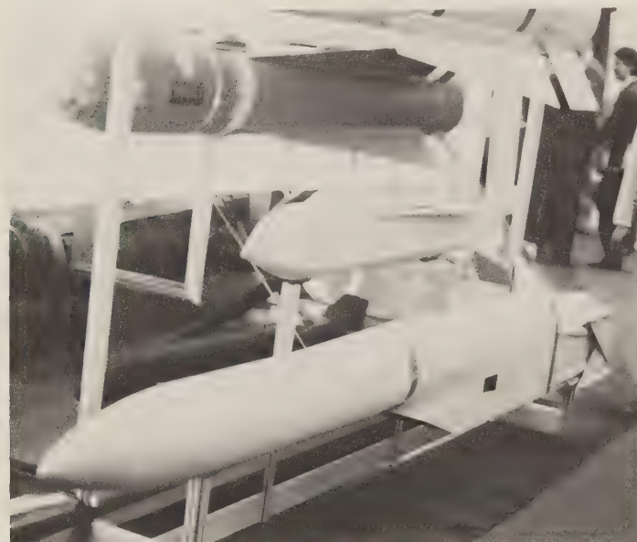
The Hughes/McDonnell Douglas version of AAAM, showing folding tail fins for tighter packing. (Author)
