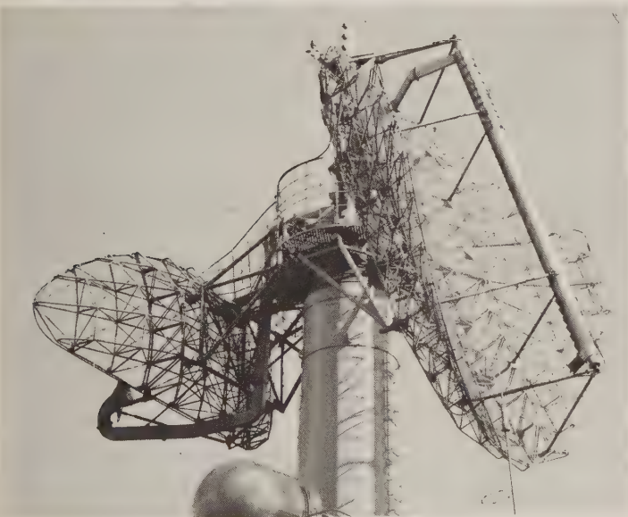
Top Pair radar on board the missile cruiser Marshal Ustinov , Norfolk, 1989. Note the interrogator (IFF) atop the array. (S. Zaloga)
