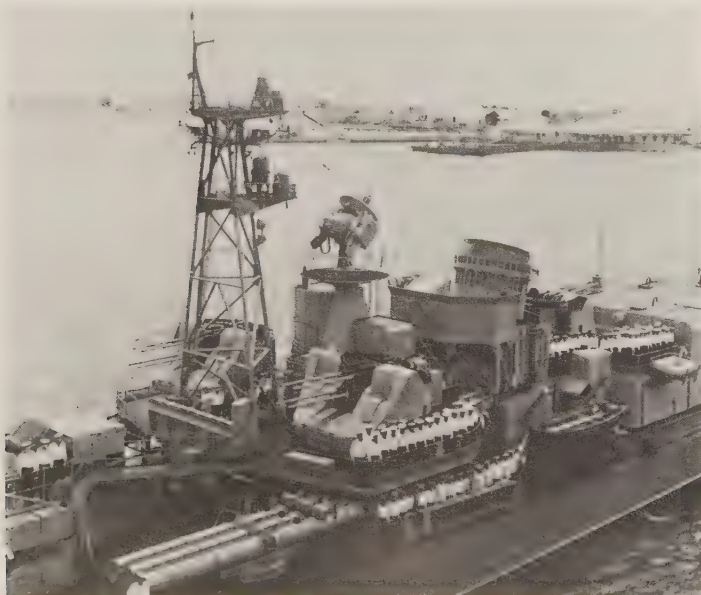
Quadruple 57-mm guns on board a Krupny-class missile destroyer. The mast radomes are presumably a pair of Top Hat jammers with the associated Bell-series ESM above. (U.S. Navy)
