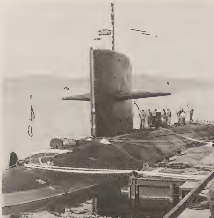
Sea Lance capsule being loaded onto an attack submarine. The submarine's HF sonar transducer is in the forward edge of the sail, and the surface-search radar is atop the sail. (Boeing)
