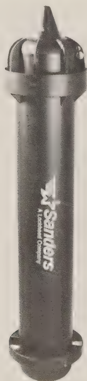
The dipping body of the Sanders-GEC LF helicopter sonar. It is the only 1 of the ALFS alternatives not to use extending arms for more directional reception. (GEC)
