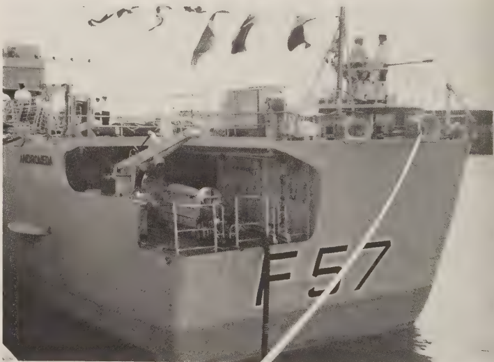
A Type 182 decoy and its handling crane on board the frigate Andromeda , 1985. (R. Cheung)
