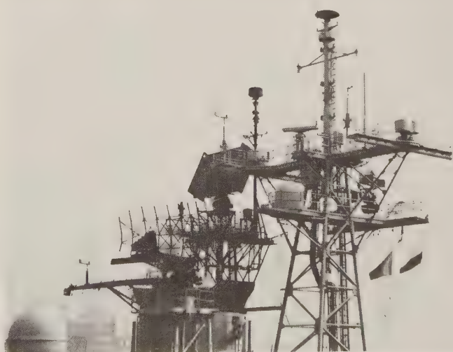
The small radome on the lower mast platform of this Spanish Perry -class frigate (mast at right) houses the directional data link for her LAMPS III helicopter. LAMPS I uses a vertical omnidirectional antenna. (S. Terzibaschitsch)
