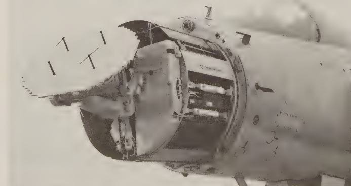
RDY radar; the small dipoles are for IFF. (Thomson-CSF)
