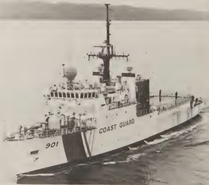
SPS-64 on board the Coast Guard cutter Bear . The egg atop the bridge is a Mk 92 fire-control system for the 76-mm/62 gun forward. Also visible is the box containing an SLQ-32 ESM system, on a platform just aft of the bridge windows. The flat object atop the mast is a TACAN aircraft beacon. (U.S. Naval Institute)
