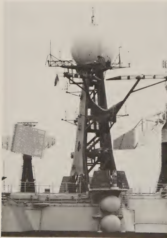
Top Knot (TACAN equivalent) on board the Soviet carrier Kiev , with Top Plate in the background and Vee Bars long-range communication antennas.
