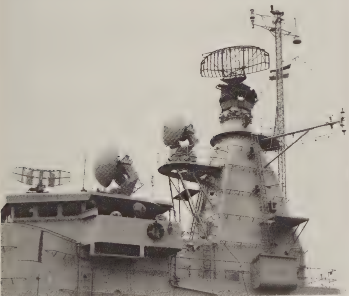
Both versions of STIR with ZW-06 (below) and DA-08 (above) on board the missile frigate Jacob van Heemskerck . (Signaal)
