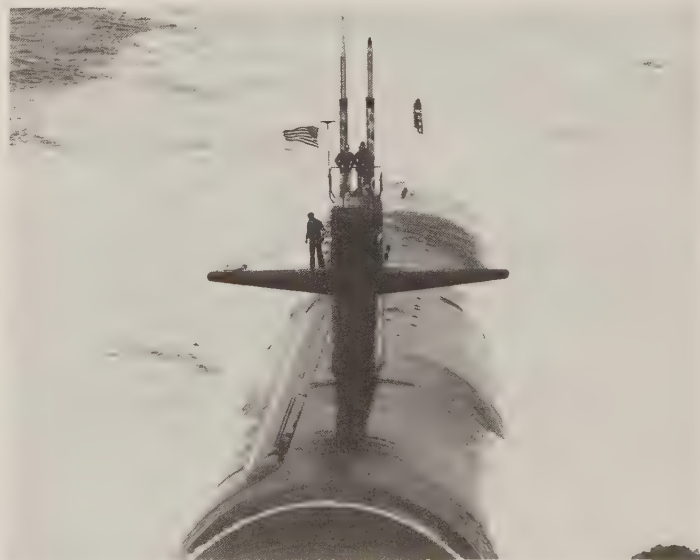
The tube running down one side of the submarine Olympia houses a towed array; there is no space within the single hull for anything so massive. Such stowage in turn limits the maximum length of the array. (U.S. Navy)
