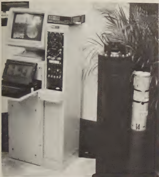
The DRS/Sparton lightweight shipboard dipping sonar, on display at the 1991 U.S. Navy League show. The electronics are at left (note the use of a laptop computer for system monitoring and control, with the larger screen reserved for the system display). At the right, the dark cylinder is the dipping transducer, with a DICASS buoy next to it for comparison. (Author)
