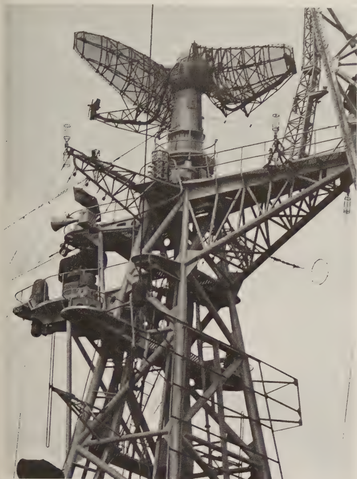
Head Net C air-search radar on board the Kashin-class destroyer Strogii at Massawa, 1972. The object at the base of the radar pedestal is a Watch Dog ESM antenna. (Royal Navy)
