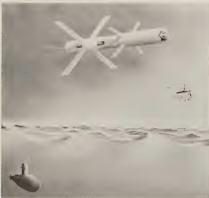
Polypheme-SM in flight, trailing its fiber-optic guidance link. The forward rocket motor is burning. (Aerospatiale)
