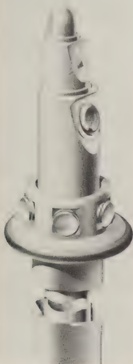
The Barr & Stroud (Pilkington) optronic mast, with ESM ports atop the wake-reducing fairing. (Pilkington)
