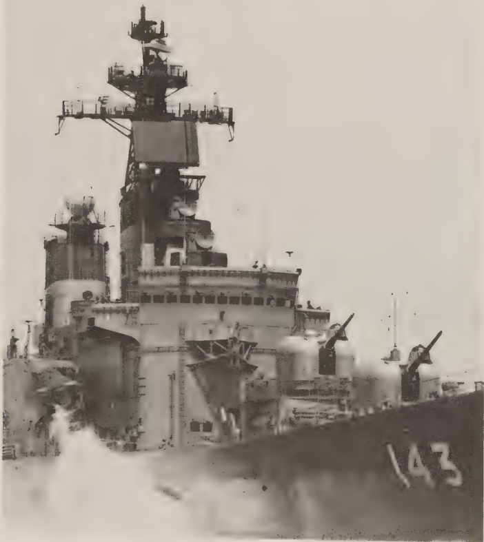
OPS-12 3D air-search radar on board the destroyer Shirane , with OPS-28 above it. The 2 gun directors above the bridge are GFCS-1A. (Japanese Maritime Self-Defense Force)
