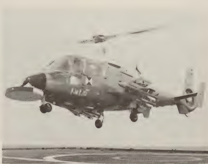
AS 15 TT, as carried by a Dauphin 2 helicopter, with AGRION 15 radar. (Aerospatiale)
