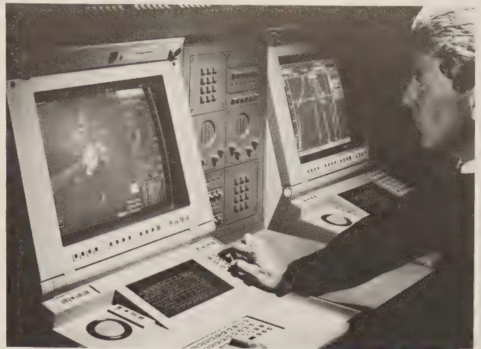
The next-generation British standard surface-ship command display, for the Type 23s' SSCS (surface ship command system). The same type of screen displays radar video at the left and sonar tracks on the right. (Racal)
