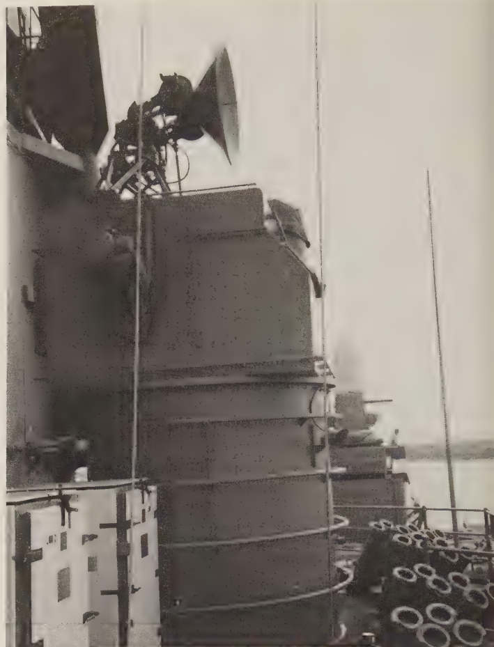
Mk 25 radar atop a Mk 37 5-in director on board the battleship Wisconsin , 1988. SRBOC chaff-launching mortars are visible to the right, on deck. (S. Terzibaschitsch)
