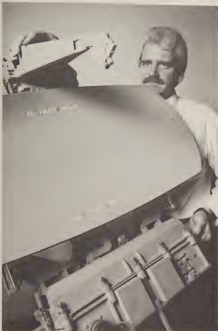
An APS-130 antenna for the EA-6B. This radar is essentially APQ-156 without the interferometer. (Norden Systems)
