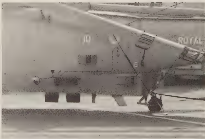
Two Orange Crop antennas (broadside and facing aft) on a Sea King helicopter, off HMS Ark Royal , 1990. There are 2 more such antennas on the nose of the helicopter, and each antenna consists of 2 cavity-backed spirals, to cover 2 frequency bands. (Author)
