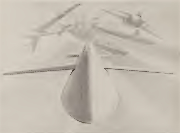
The General Dynamics version of LRCSW. It has an unducted-fan engine, which is not visible here. The wings and tail are swept forward at a small angle, and the vertical fin extends below the missile. (General Dynamics)
