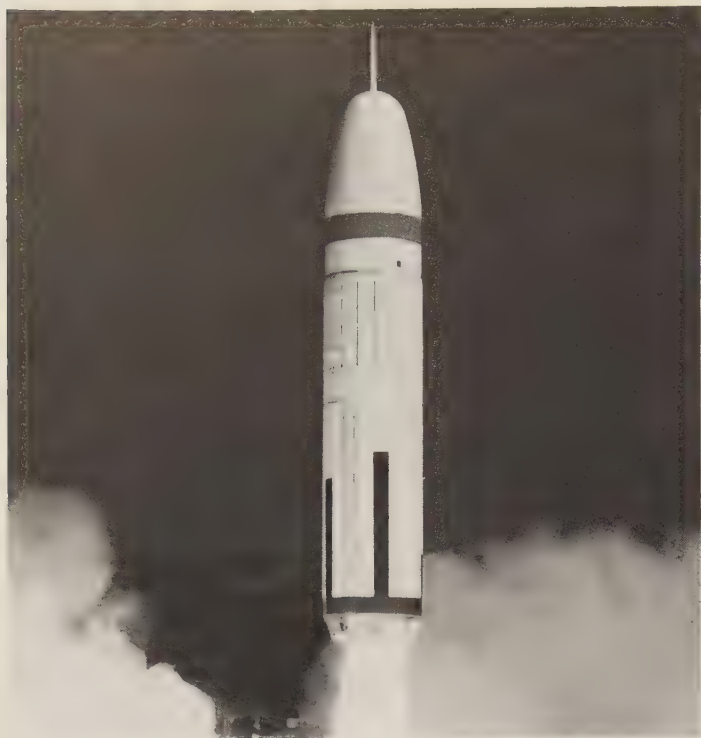
Trident C-4 launching, with the aerospike extended. (U.S. Navy)
