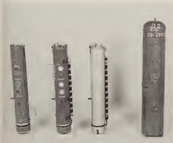
Standard Soviet sonobuoys: 3 RGM (RGB-56) on the left, RGBN (RG-64) on the right. All are still in use. (U.S. Navy)
