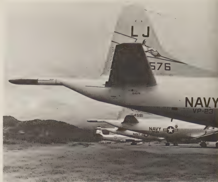
ASQ-81 MAD stingers on a line of P-3 Orions. The radomes below the MAD boom carry the rear antenna of the APS-115 radar, so that a 360-deg search can be maintained without the drag associated with hanging a radome below the airplane. (U.S. Navy)
