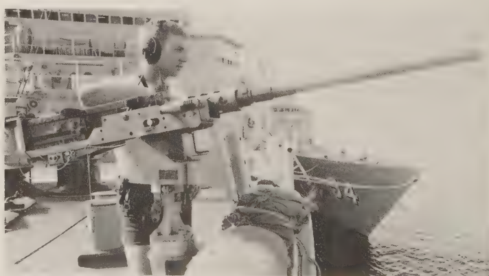
A 0.50-caliber machine gun on board the Mount Vernon in the Persian Gulf, October 1987. There are supports for a splinter shield, which has not been fitted in this case. U.S. ships in the Gulf were also provided with M60 light (7.62-mm) machine guns. (U.S. Navy)
