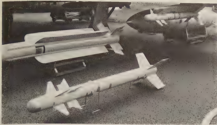
Magic 2. Unlike Sidewinder, Magic 2 has no air-driven gyros on its tail fins. (Author)
