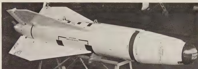
Walleye. Note the television nose (covered until flight) and the wind-mill generator at the tail. (U.S. Navy)
