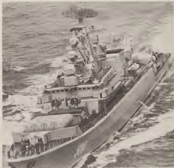
A Krivak-class frigate shows her quadruple SS-N-14 launcher, with a pair of RBU-6000s just abaft it. The 2 shrouded antennas on lattice mast above the bridge are the Eye Bowls controlling the SS-N-14 missiles; above them is a Don Kay surface-search radar, with Head Net C at the masthead. The shrouded object immediately over the bridge is Pop Group, to control SA-N-4 anti-aircraft missiles. (U.S. Naval Institute)
