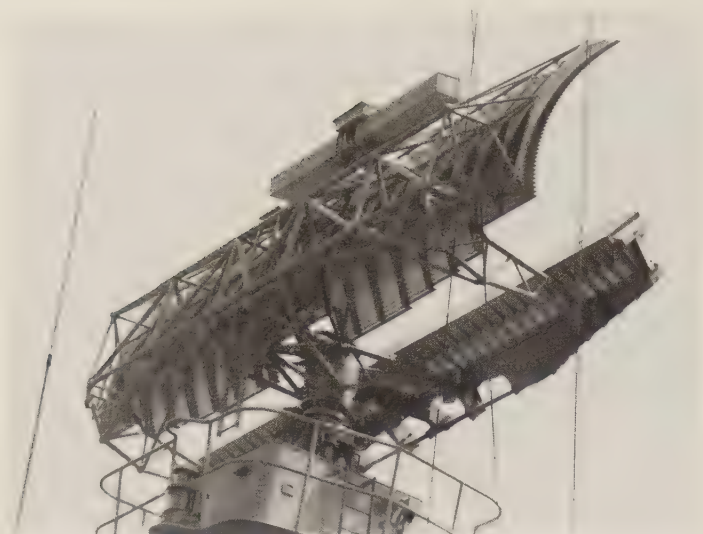
Type 1022 on board HMS Ark Royal , 1986, seen from below and behind. The squintless feed array of horns is visible. [Author]
