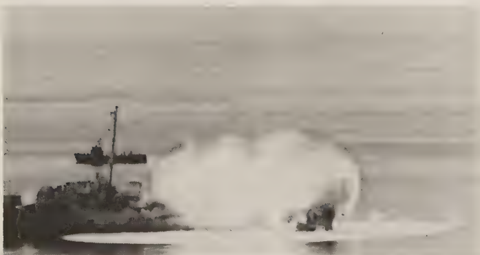
The effect of a fuel-air explosion, shown in a sequence of 1972 photographs of a simulated near miss on the former destroyer escort McNulty . Note the dispersion of the cloud before the detonators are fired into it. The second and third photos show how the cloud envelops the ship and then goes off (note the shock wave in the water). (U.S. Navy)
