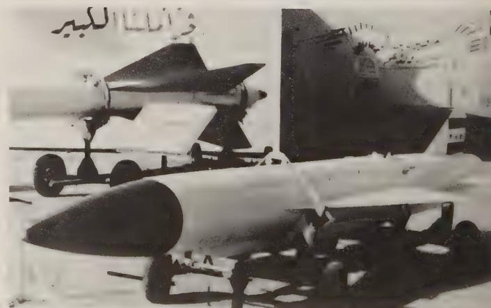
AS-9 antiradar missile. Note the strong family resemblance to the much larger AS-4 and AS-6. This example was displayed in Baghdad in 1989. The missile in the background is Nissan-28, apparently a Soviet-supplied AA-7 mocked up to simulate an antiship weapon.
