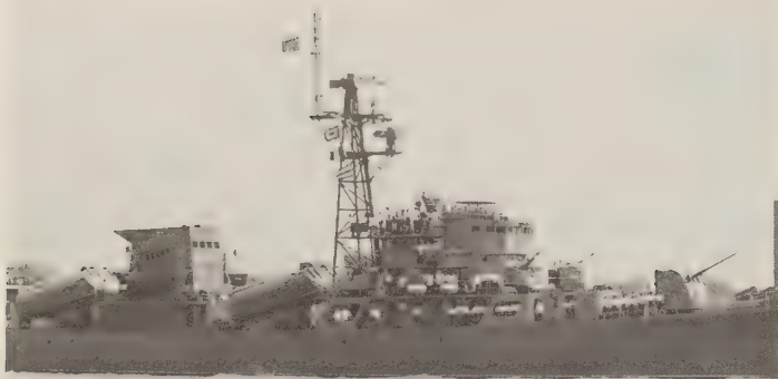
A Chinese Jianghu -class frigate shows an Eye Shield radar at her mast-head, with a Type-756 navigational radar (the slotted waveguide) and Square Tie (missile fire control) below it. (U.S. Naval Institute)
