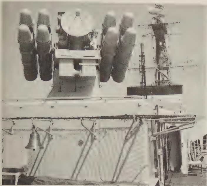
Crotale Naval launcher with colocated fire-control radar. The IR tracker is to the left of the radar dish. (Thomson-CSF)
