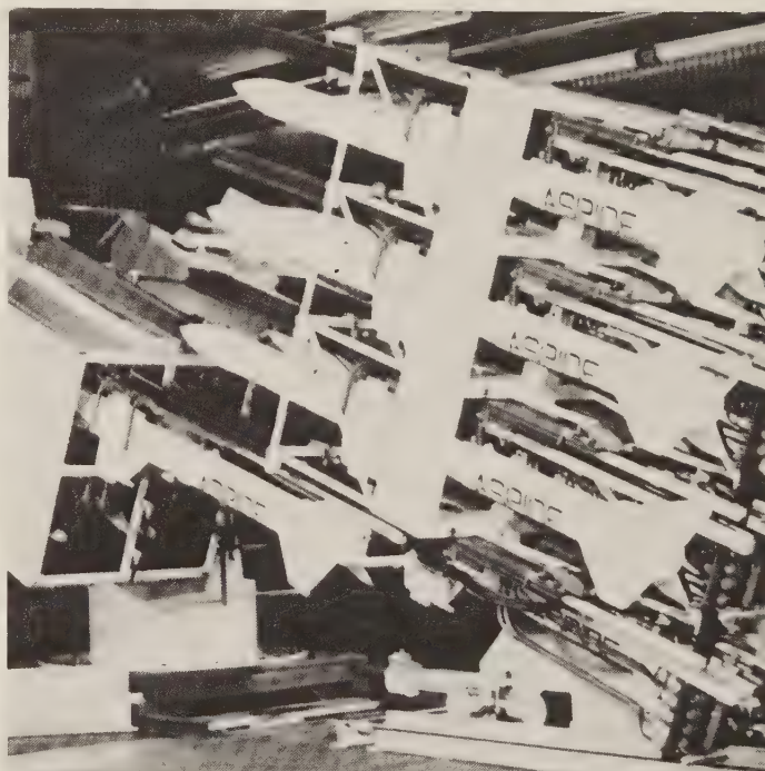
Sixteen-missile automatic loader for Aspide. This system and the Canadian Tribal-class Sea Sparrow are the only Western point-defense missile systems not reloaded by hand. (Selenia)
