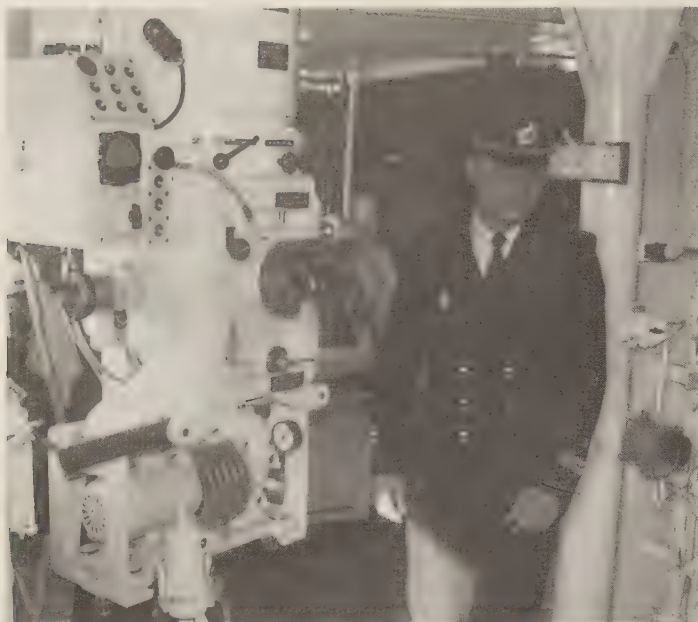
The periscope in the enclosed combat command station of the cruiser Kerch , on the same level as, and abaft, her bridge. This station does not contain radar fire-control equipment but does include radar directors like the one visible in the background, as well as a steering console. (Eric Grove)
