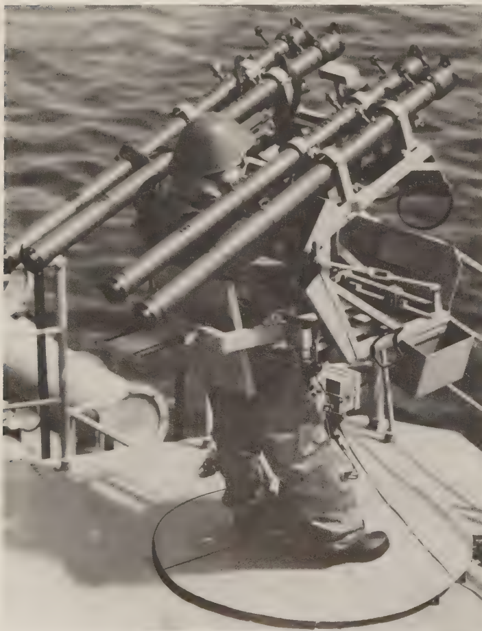
A standard quadruple SA-N-5 mounting. Many Soviet submarines carry single SA-N-5 tubes.
