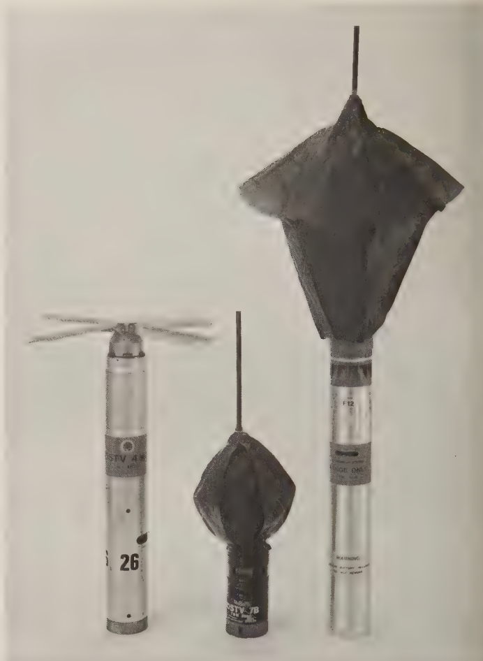
Standard French sonobuoys, showing a rotachute atop the passive DSTV 4M at left and ballute/antenna floats on the DSTV 7B and the range-only active buoys. (Thomson Sintra)
