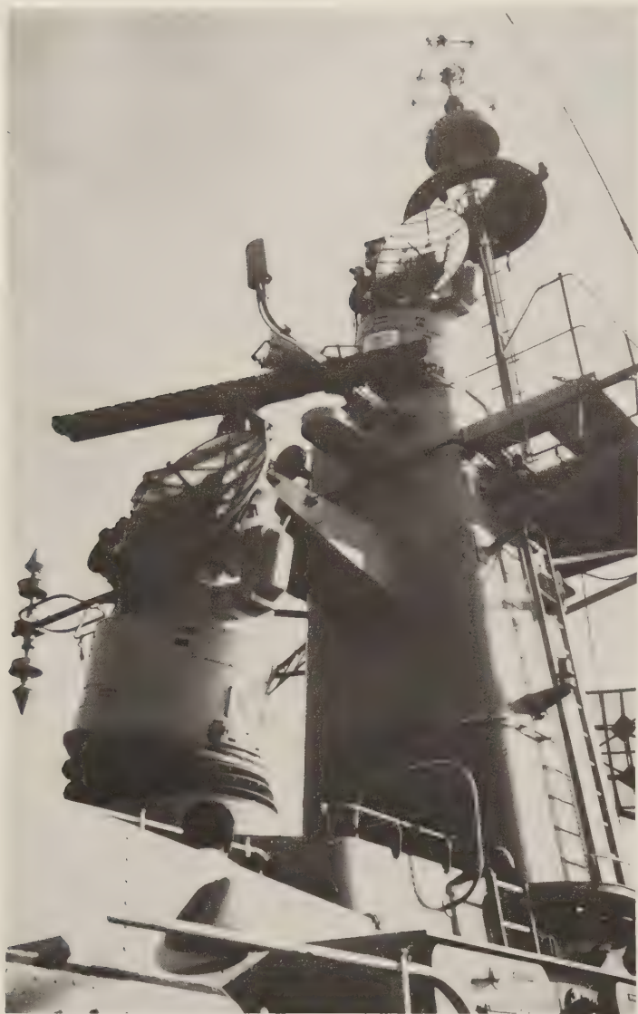
Sea Hunter 4 on board an Iranian Vosper-Thornycroft frigate, with a separate search antenna. Both tracker mounts carry Sea Killer command antennas. (Contraves)
