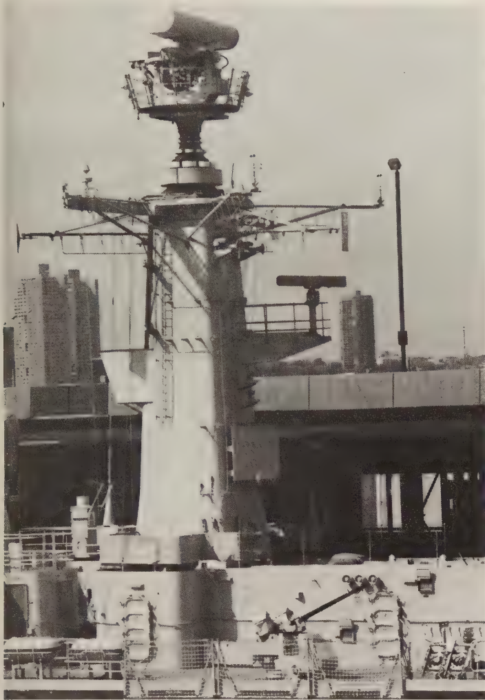
Back-to-back Type 967/968 radars at the masthead of the British Type 22 frigate HMS Cumberland , 1990. The antenna halfway down the mast is a Type 1007 surface-search set. The flat oblong visible near the base of the mast is used to calibrate the ship's forward Sea Wolf director. The array of directional antennas surrounding the mast beneath the 967/968 platform serves the UAA-1 ESM system; several small radomes on yards are omnidirectional antennas (for IFM) for the same system. Near the base of the mast is a DS-30B gun. (Author)
