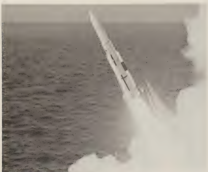
Standard Missile (Medium Range) being fired from a Mk 26 launcher. The SM-1, SM-2, and Tartar missiles are virtually identical in appearance, though quite different in capability. (U.S. Navy)
