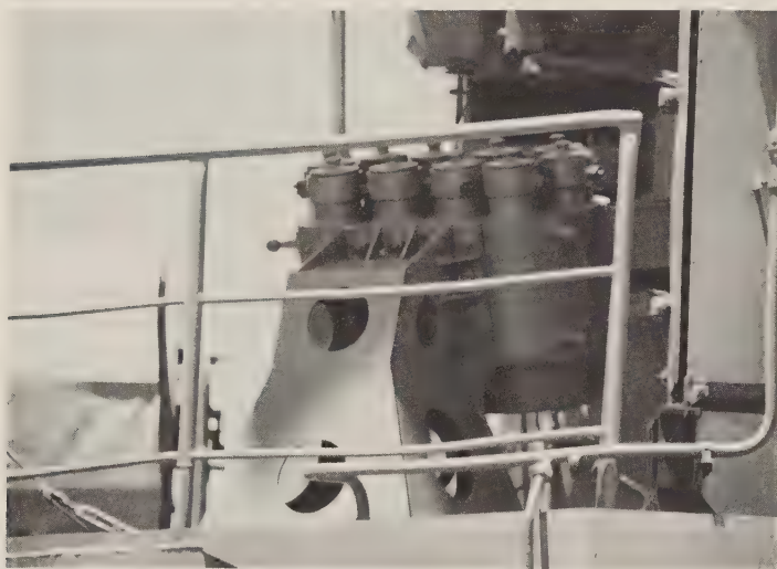
Two of the new 10-tube chaff launchers, 1 horizontal and the other nearly vertical, on board the Udaloy -class destroyer Admiral Vinogradov , July 1990. (S. Zaloga)
