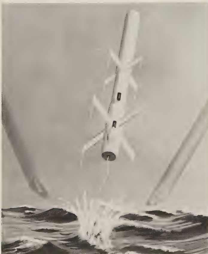
Polypheme-SM emerges from the water, its canister falling away. The after rocket motor is burning. (Aerospatiale)
