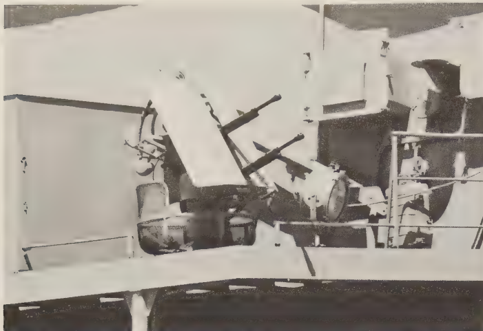
A Soviet under-and-over 12.7-mm machine gun on board the Udaloy -class destroyer Admiral Vinogradov , 1990. The ship carried 4 such mounts. (S. Zaloga)
