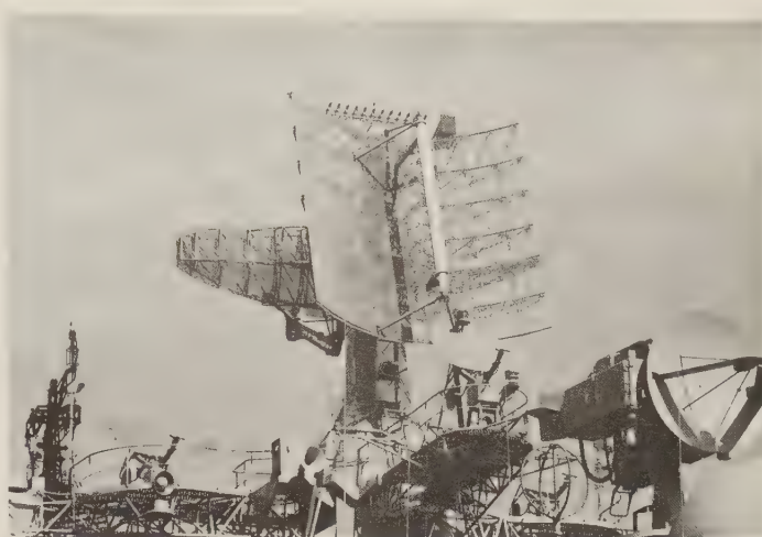
Top Steer radar on the missile destroyer Otlichnyy visiting Norfolk, 1989. The tube running up in front of the radar reflector carries the serpentine feed for frequency scanning. The array above the antenna is the Long Head IFF interrogator. (S. Zaloga)
