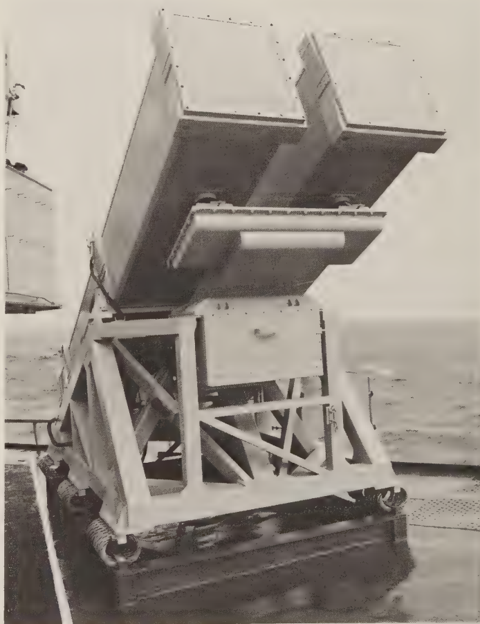
A twin Standard Missile launcher on board a Taiwanese WJ-III (modified FRAM Gearing ) destroyer. This type is unique to the Taiwanese navy. (F. S. Mei)
