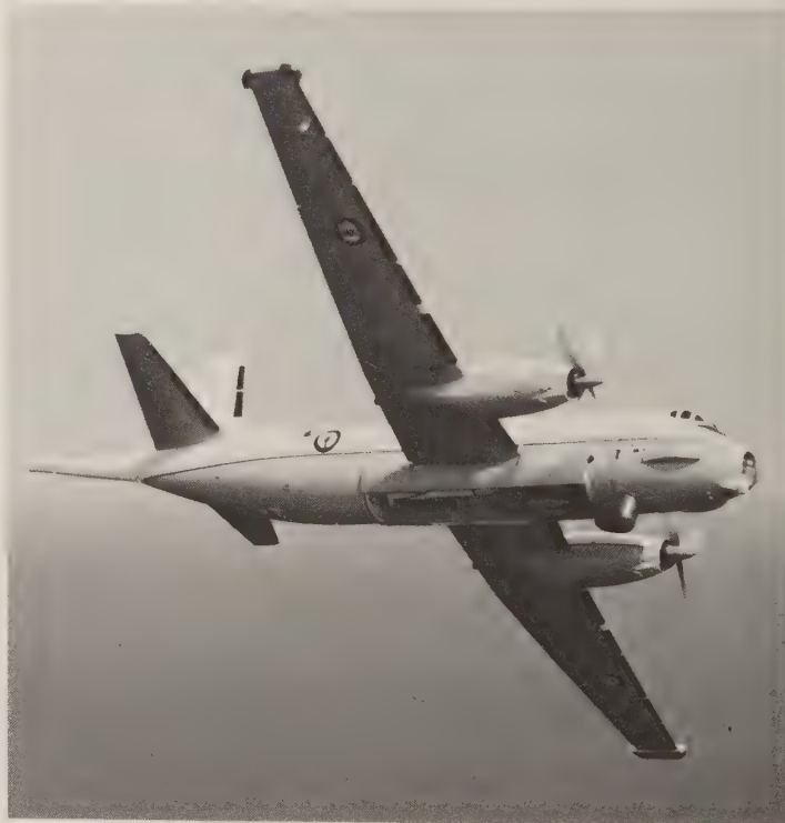
An Atlantique Nouvelle Generation (Atlantique Mk 2) displays its IGUANE radar and its ESM systems in the wingtips. Any radar pushed out into the airstream creates drag, but that offset from the main airframe is the only way a single reflector can cover anything approaching 360 deg. Offset was the solution in aircraft such as the Alizé, the P-2, and the S-2. The alternative is to use 2 reflectors (as in the P-3) or to accept 180-deg scanning (as in the S-3, which has a nose radar). The bulge under the transparent nose contains a gyro-stabilized high-resolution thermal imaging camera, Tango, with a switchable 6.45 \times 4.30/2.15 \times 1.43 deg field of view (the turret can turn to 110 deg to either side of the airplane, and its elevation limits are +15/-45 deg. The output is a 625-line television signal, 50.5 frames/sec. (U.S. Naval Institute)
