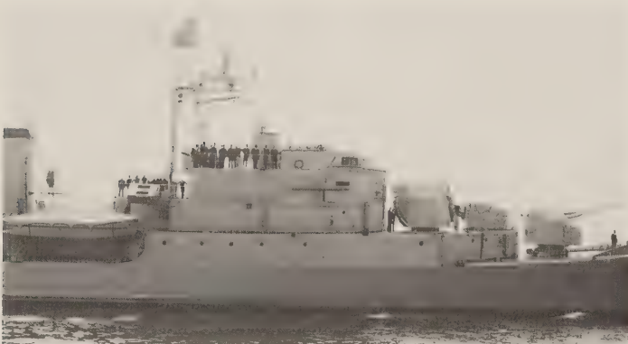
305-mm ASW mortar between bridge and forward gun, Commandant Rivière . The mortar is in the loading position. (Stefan Terzibaschitsch)
