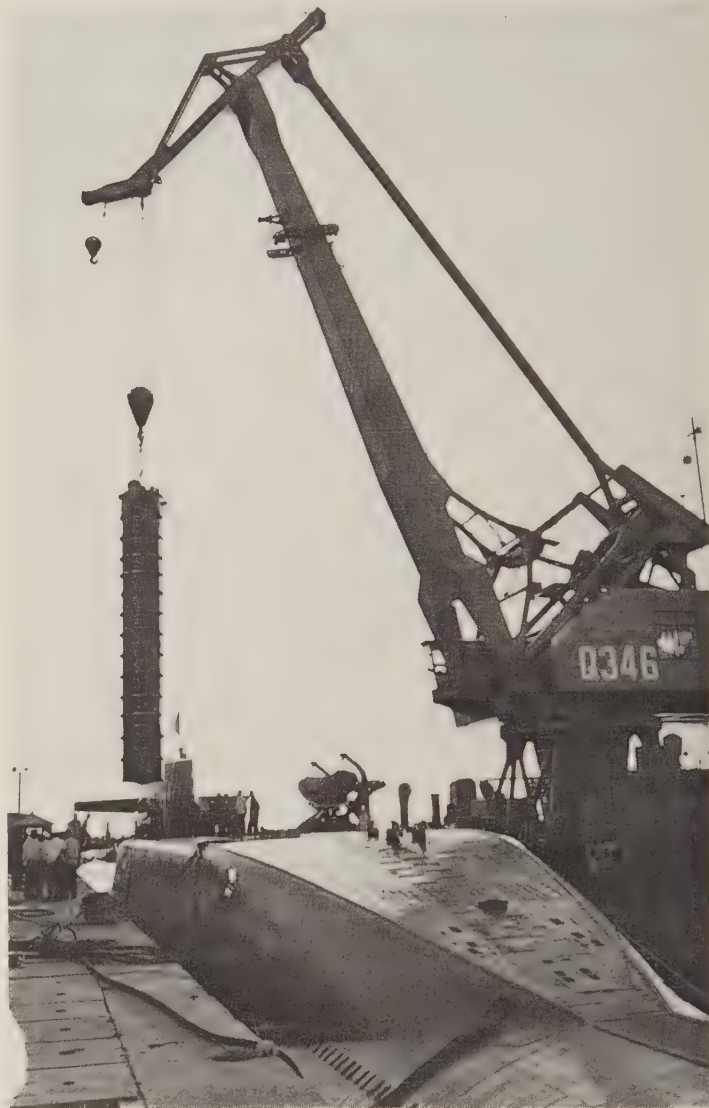
A C-SS-N-3 missile being loaded on board a Chinese Xia-class submarine. ( Ships of the World )
