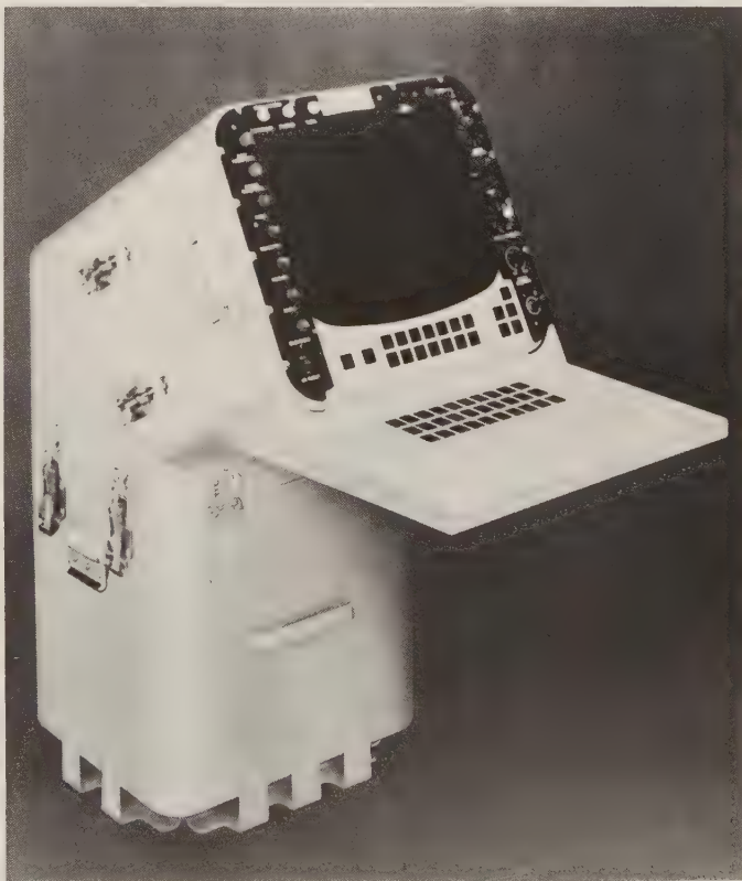
SPA-50G, a new-generation console, parallel in concept to SPA-25G. Such consoles include automatic radar target detectors and, thus, can be used to feed combat data systems such as FFISTS. (ISC Cardion)
