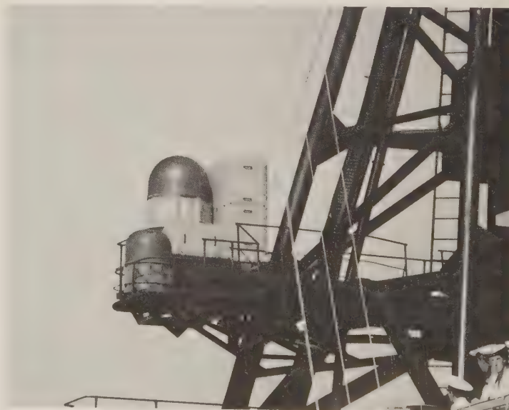
Wine Glass (inboard) and (probably) Bell Crown (outboard) on the mainmast of the missile destroyer Admiral Vinogradov , 1990. (S. Zaloga)
