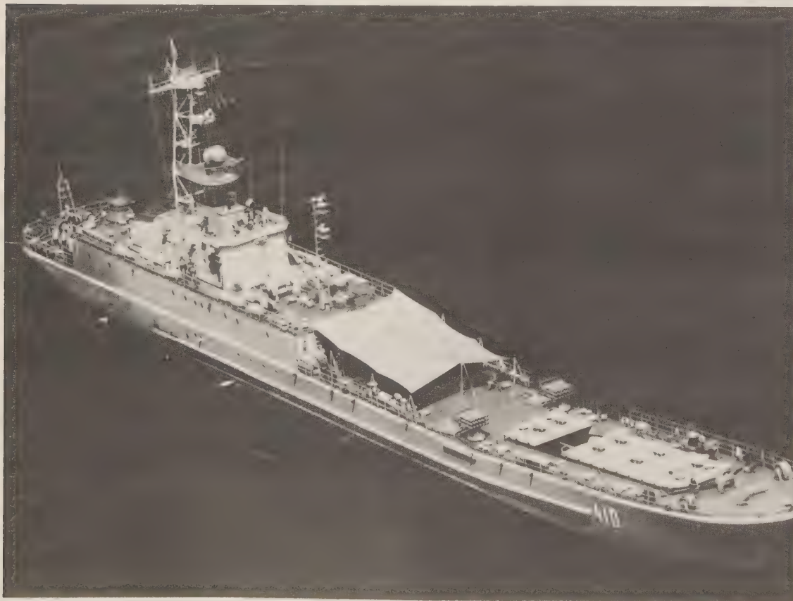
BM 14/18 rocket launchers forward on board a Polnocny -class landing ship. The radar is Drum Tilt, controlling a twin 30-mm gun at the after end of the superstructure. (U.S. Navy)
