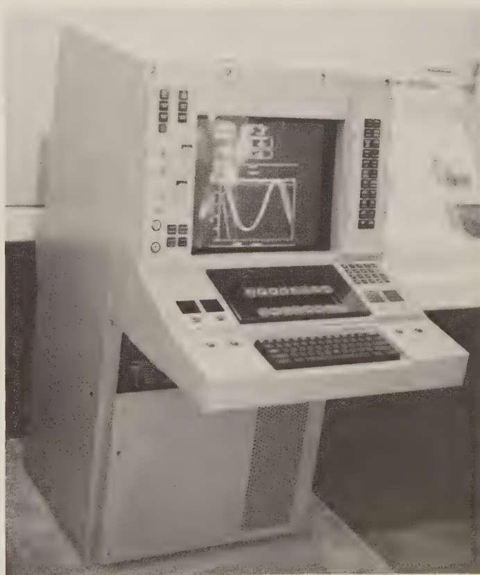
Raytheon's CCS Mk 2 console, which the company hopes also to use for its new integrated combat system. (Author)
