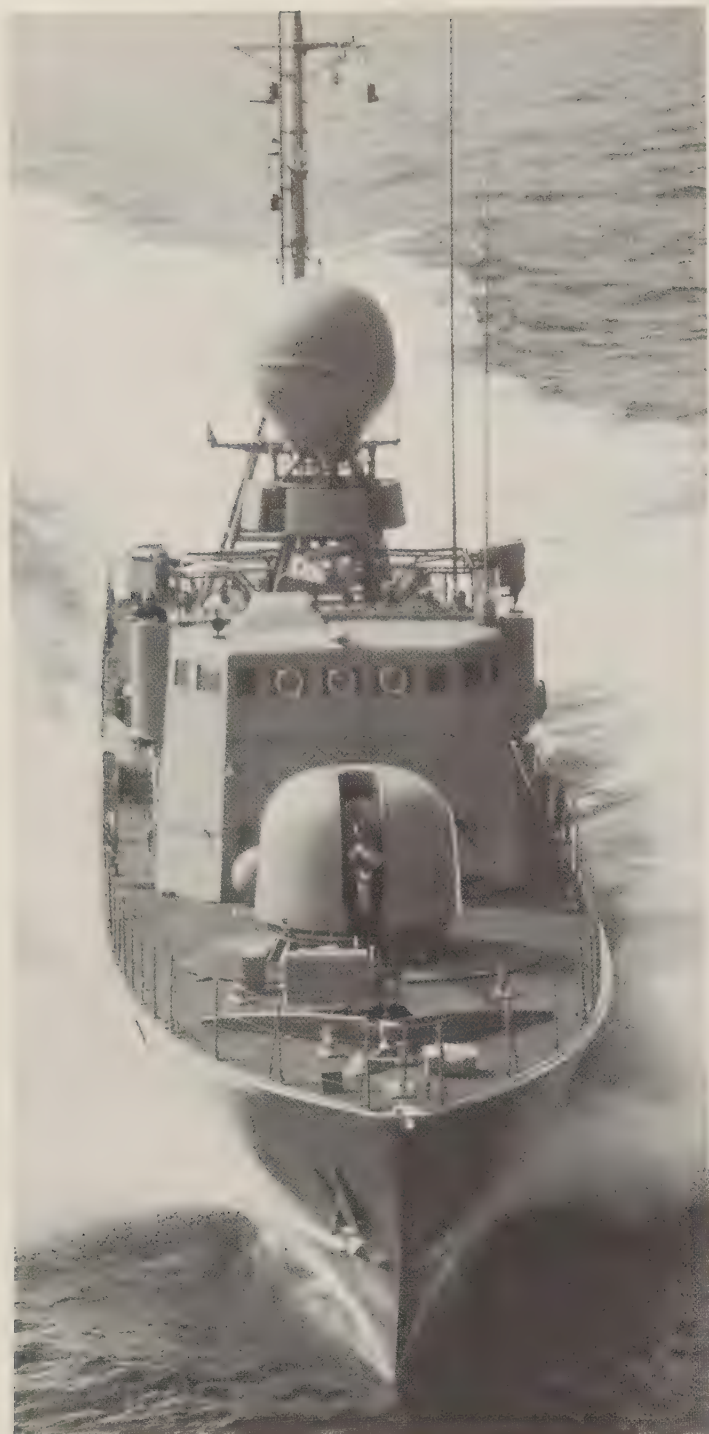
FL1800S on board a German fast patrol boat. The DF antennas are below the Signaal "egg" radome, and the jamming antennas are above the sides of the bridge. (AEG)
