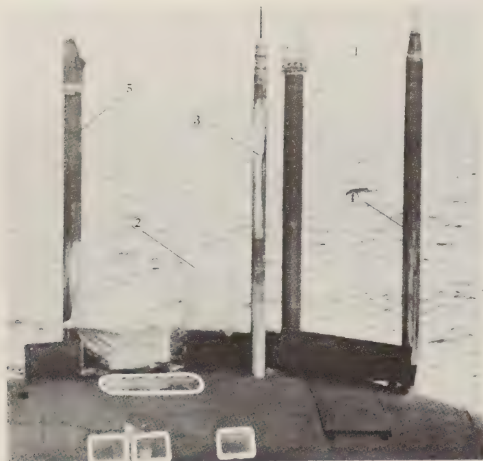
Brick Pulp (2) on board a Victor-class submarine. The other visible masts are: (1) the Snoop Tray radar, (3) the VHF antenna, (4) the VHF antenna, and (5) the search periscope. This type of submarine has a total of 9 masts, the others carrying Pert Spring (navigation) and Park Lamp (VLF/LF reception), an attack periscope, and a snorkel. ( Sea Power )
