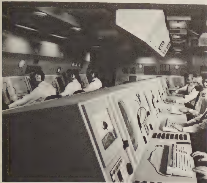
Full-scale mock-up of the M-frigate operations room at the Netherlands Institute of Perception at Soesterberg, showing the new standard consoles in use. Note the video (the helicopter) displayed on the console in the foreground. The full CIC (operations room) contains 14 GOS consoles. (Signaal)
