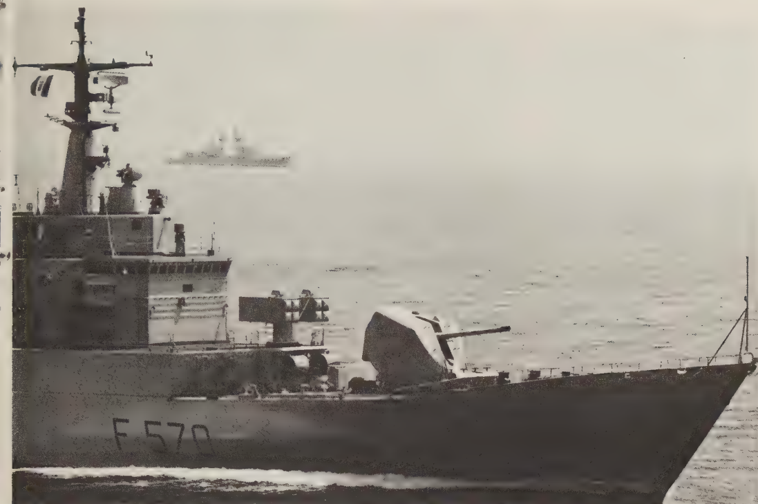
The Italian frigate Maestrale is equipped with the Lambda (SLQ-D/SLR-4) system. The cylinder above her bridge is an ELT 814 omnidirectional jammer. A similar centerline radome is mounted atop her helicopter hangar. (Coll. S. Cioglia)
