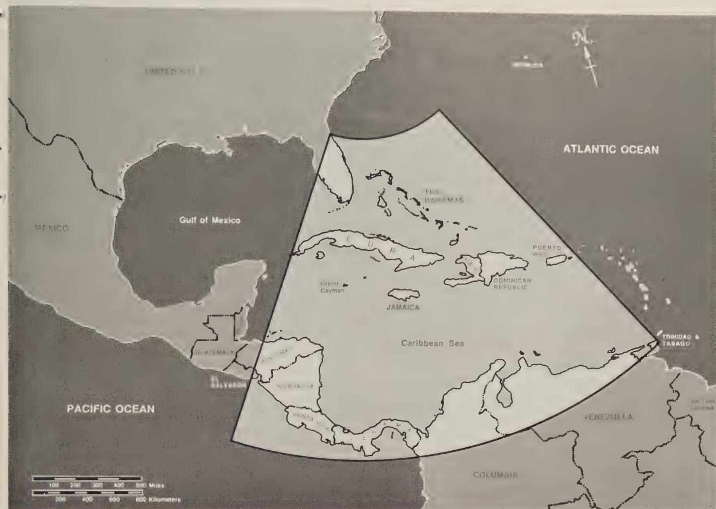
ROTHR coverage of 1.6 million square miles of the Caribbean, from a radar located in Virginia. (Raytheon)
