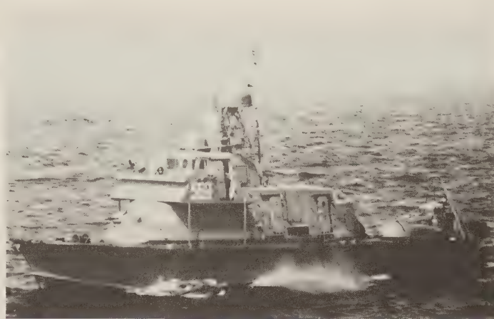
Twin 14.5-mm machine guns forward, on board a Pchela-class patrol boat. Although this class has been discarded, the same mount is used on board the replacement Zhuk class. The radar is Pot Drum. (U.S. Naval Institute)
