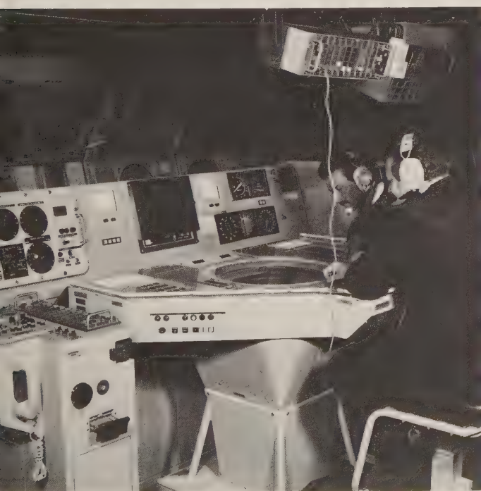
Standard Signaal horizontal display console (HDC) on board the Dutch air-defense frigate Jacob van Heemskerck . (Signaal)
