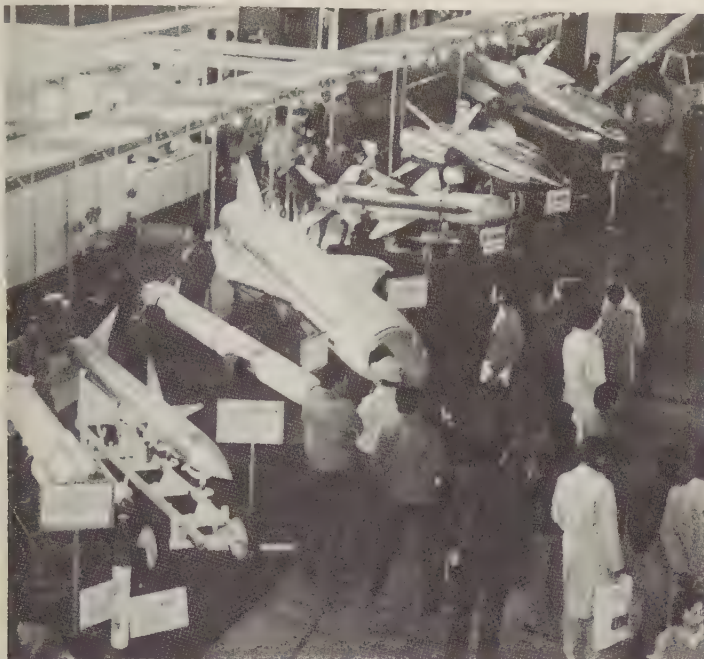
Chinese missiles manufactured by CPMIEC on display at ASIINDEX 1988. From the top, they are M-1B, C301, C101, C802, C201, M-1, and HQ-61 (SAM). M-1 and M-1B are army artillery rockets fired from multiple launchers; -1B is heavier and achieves a greater range. (CPMIEC)
