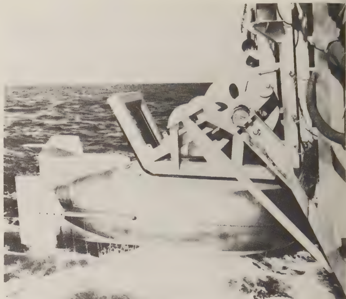
DE 1164 fish shown after it had been streamed and recovered by the Italian frigate Maestrale , March 1982. (Raytheon)
