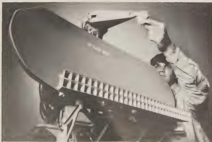
An APQ-156 antenna, showing the phase interferometer below the main reflector. (Norden Systems)
