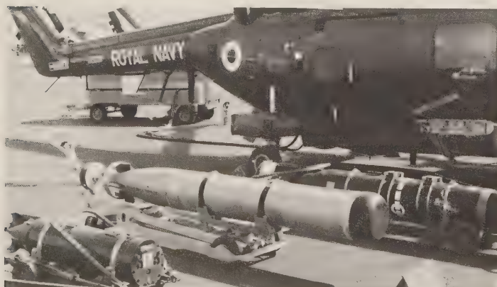
A-244/S at Farnborough, 1990. The shroud ring (used instead of fins for directional control) suggests its relationship with the earlier U.S. Mk 44. The object in the foreground is a dummy Mk 11 depth charge; in the background is a Stingray torpedo. (Author)
