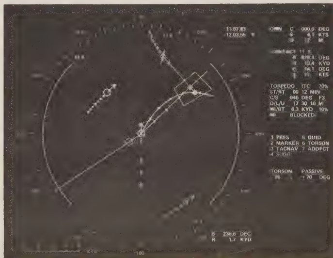
OSID threat-evaluation display, showing a calculated torpedo-intercept path. (KAE)
