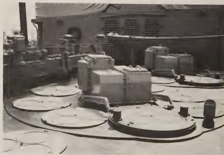
An SA-N-6 launcher on board the cruiser Marshal Ustinov . In contrast to Western vertical launchers, only 1 missile can be launched at a time (only 1 section opens); the triple circular plates over other missile positions are apparently blow-out plates. (S. Zaloga)
