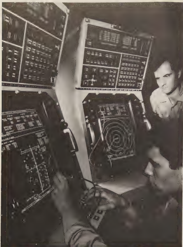
Librascope's SFCS Mk 1 consoles, showing an active sonar B-scan at left and a tactical summary plot (PPI) at right. (Librascope)
