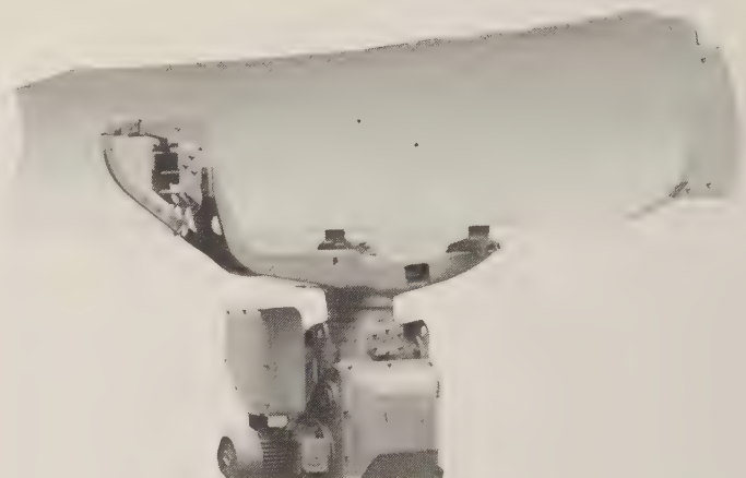
SPN-728 antenna, for navigation and surface search. This medium-power X-band radar is supplied with several alternative roll- and pitch-stabilized antennas. There are four alternative pulse widths, and the display is a raster rather than a rotating scan, partly so that the radar can use low-cost television-type monitors as repeaters. Targets are automatically detected. (SMA)
