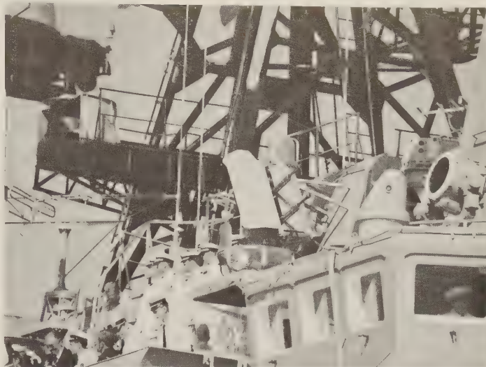
A heavily shrouded radome, apparently an auxiliary Bell Squat, on an outrigger on the foremast of the destroyer Admiral Vinogradov , 1990. The shielding testifies to considerable electromagnetic interference from shipboard radars and communications gear, such as the Round House tactical-air-navigation antenna in the upper right-hand corner of the photograph. (S. Zaloga)
