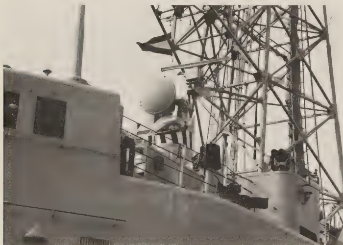
SPG-515 fire-control radar (MK 60 director) on board the Canadian destroyer Annapolis , 1989. (G. Till)
