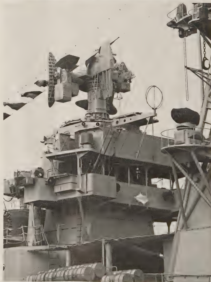
Peel Group missile (SA-N-1) fire-control radar directors on board the Kashin-class destroyer Strogii at Massawa, 1972, showing the characteristic pairs of large and small horizontal and vertical antennas, for target and missile tracking. (Royal Navy)
