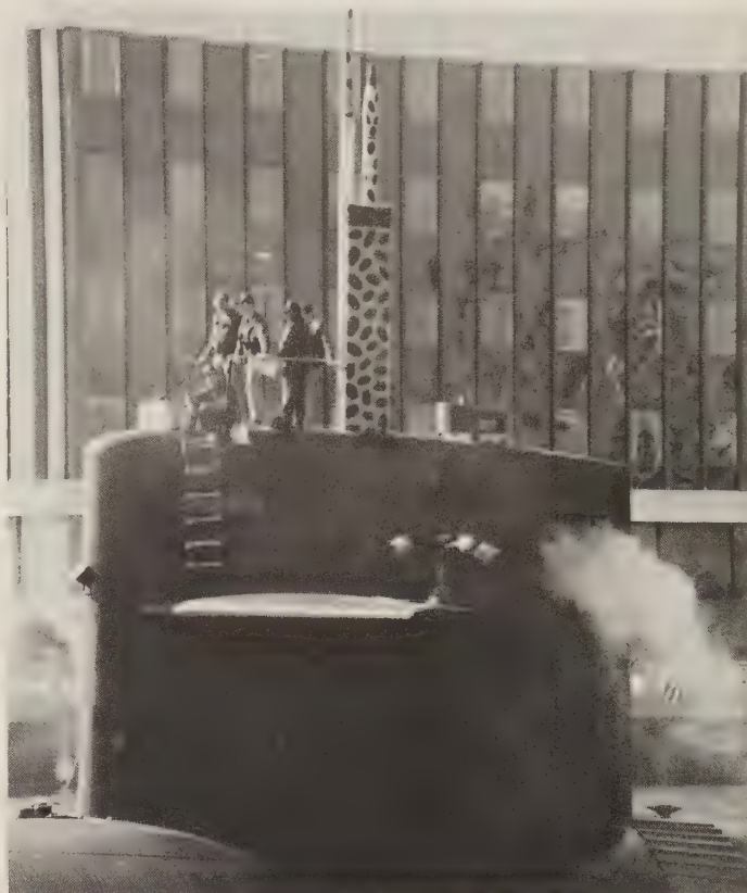
Typical U.S. faired periscopes aboard a Los Angeles -class submarine off Norfolk, October 1986. (Jürg Kürsener)
