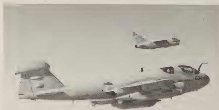
An EA-6B of VAQ-140, 1988, displays the leading features of the ALQ-99 system: the tail radome (for all-around view) and the underwing pods. The 2 strakes on the vertical tail are ALQ-99 receivers for Bands 1 and 2. The short stub protruding aft from the tail radome (the "beer can") is for ALQ-126, added during the ICAP-1 program. (U.S. Navy)
