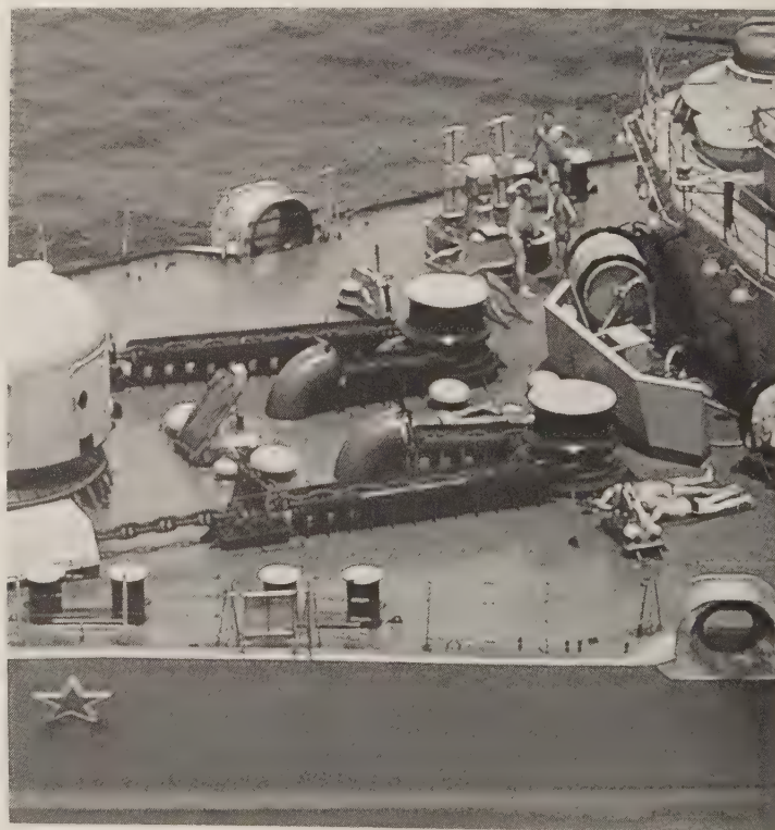
SA-N-10 launcher (upper center) on board the intelligence-gathering ship SSV-33. It is 1 of 3 on board (2 are aft). Immediately abaft it are a Kolonka remote visual sight and a pair of Tin Man remote optronic devices; forward is a 76-mm gun. The launcher presumably reloads automatically from below. (Sea Power)
