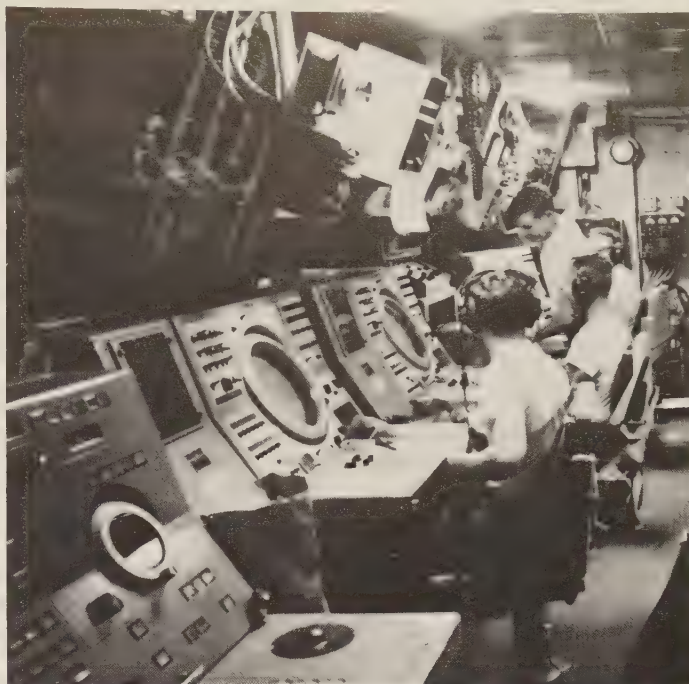
NTDS consoles on board the missile cruiser Wainwright , 1968. Each console has a trackball that the operator uses to position a cursor over the blip he wants to enter into the system; one such ball is visible on the table in the foreground, and one is being manipulated by the second man from the right. (U.S. Navy)
