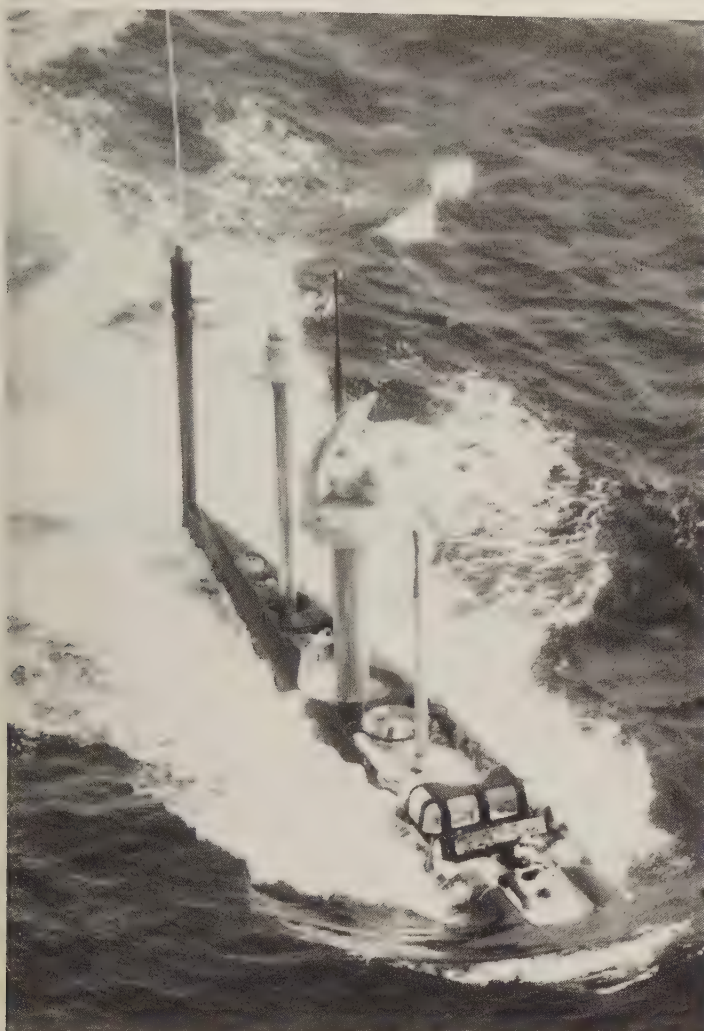
Snoop Slab search radar on board an Echo-II-class submarine. Aft it is a Stop Light C ESM antenna, a hemispherical antenna atop a series of monopulse DF antennas operating in 4 bands. The Front Door/Front Piece missile-guidance antennas are forward of the windshield, submerged, and the after end of the sail carries a standard HF whip.
