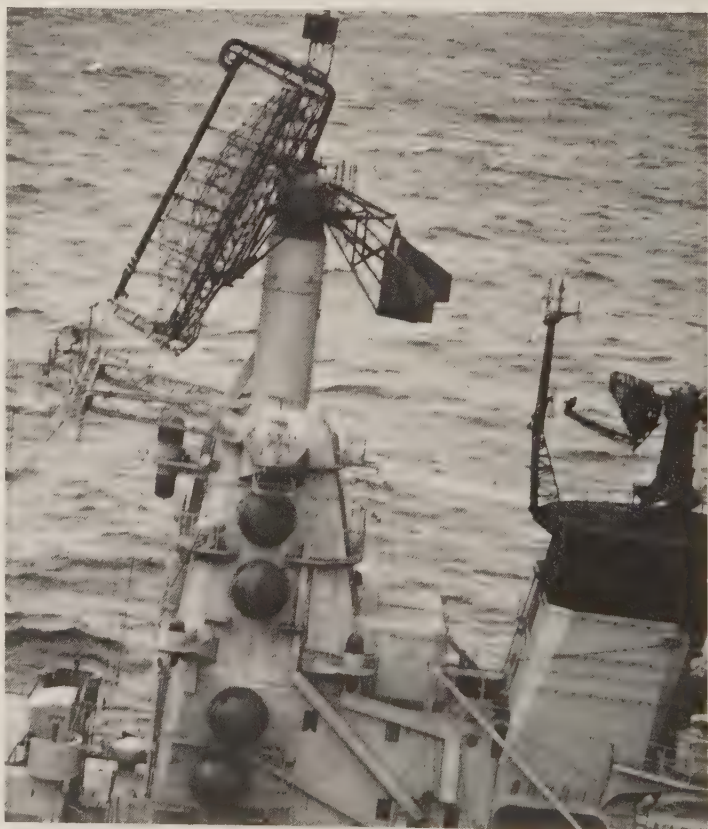
Top Sail on board a Kresta-II -class cruiser. The long straight element in front of the reflector is the twisted feed, which performs the same function as the sinuous feed in a U.S. frequency-scanning radar. The extra feed at the top is presumably for IFF. (U.S. Navy)
