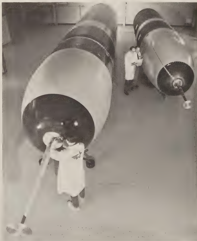
Trident C-4 (right) compared to Trident D-5 (left). Note the aerospikes. (Lockheed)
