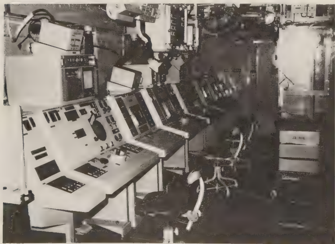
Operations room (CIC) of an Iranian Vosper-Thornycroft frigate, showing the target-designation console, with its pantograph, in the foreground. (Contraves)
