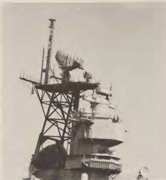
The battleship Iowa shows her Mk 13 radar, in the long nacelle above her range-finder, 1986. The mast above carries SPS-49 and SPS-67 (for surface search). (Author)
