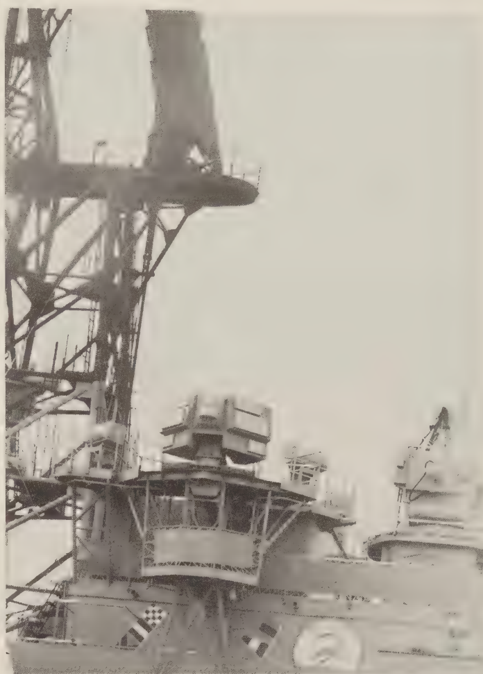
SLQ-32(V)3 on board the missile destroyer Dahlgren , 1986. The 2 flanking radomes contain lens antennas that improve Band 1 DF accuracy, for antiship missile targeting. (Author)
