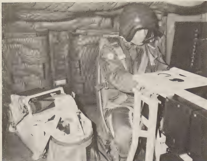
HS 12 on a Lynx helicopter. The dipping body and winch are on the left, the control panel on the right. (Thomson Sintra)
