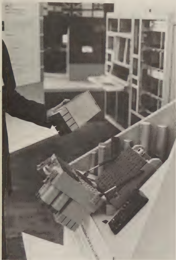
The ADS-10 helicopter-countermeasures dispenser, on display at the RNEE show in 1989. It is opened for loading, with a typical magazine at left. The contacts on the inner panel identify the magazine to the system and allow the system to launch cartridges. (Author)
