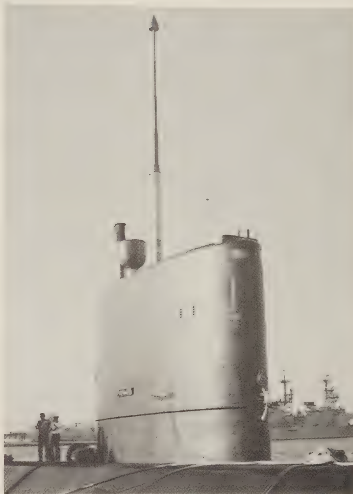
HMS Trafalgar shows her ESM search outfit (UAB) atop a telescopic mast. The other two masts are, fore to aft, the snorkel induction (air intake) and the diesel exhaust for her emergency diesel. Forward are a radar mast and two side-by-side periscopes, all retracted. This photograph probably dates from 1985; more recent ones show a much more elaborate ESM array, with at least four monopulse DF antennas (probably spirals) around the broad-band cone visible here, and a short dipole surmounting the cone. These two antenna systems may be part of UA-11/12, the simpler cone being the UAB antenna. (G. Arra via Ships of the World )
