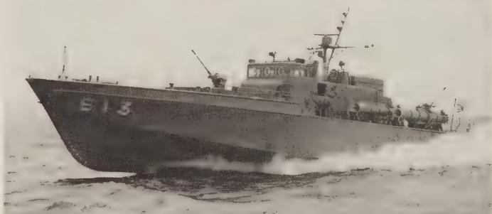
The Japanese torpedo boat PT 13 is equipped with an OPS-13 surface-search radar. ( Ships of the World )
