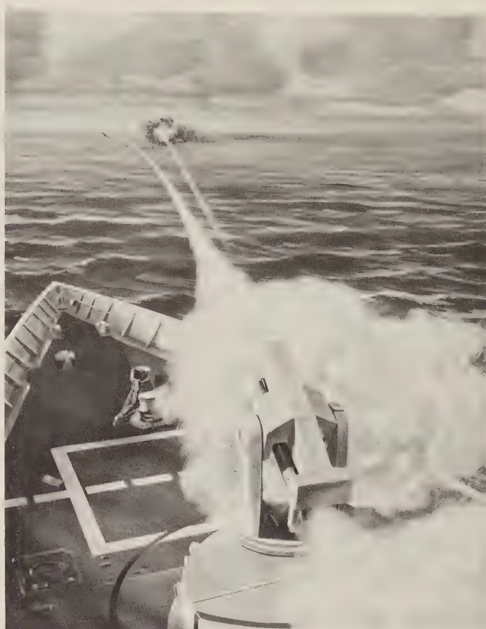
FMC is currently studying a variety of modified standard launchers, including the proposal to mix Standard Missiles and 2-RAM strongbacks in a Mk 13 magazine, illustrated here. The RAMs could be ripple-fired, and the strongback ejected as soon as they had been fired. FMC has proposed similar modifications to Mk 10, 22, and 26 launchers. The Mk 13 project is being funded as part of the Perry -class improvement program. (FMC)
