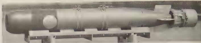
Mk 46 torpedo, showing its propeller shroud and parachute pack. (U.S. Navy)
