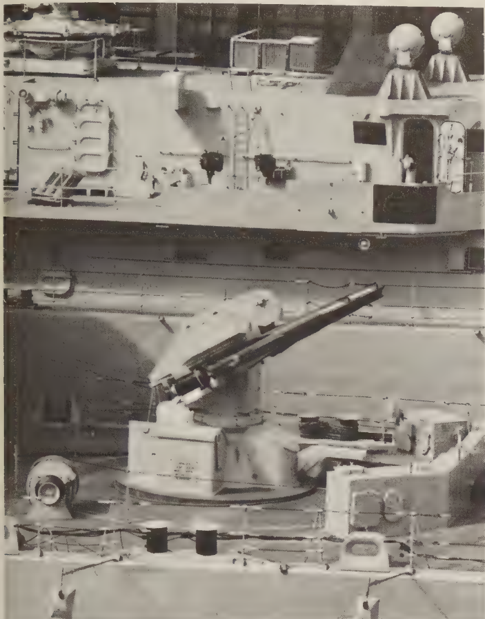
A Sea Dart launcher (Mk 30) on board the missile destroyer HMS Glasgow, 1990. In contrast to U.S. vertically loaded launchers, the blast doors project well above the ship's deck. (Author)
