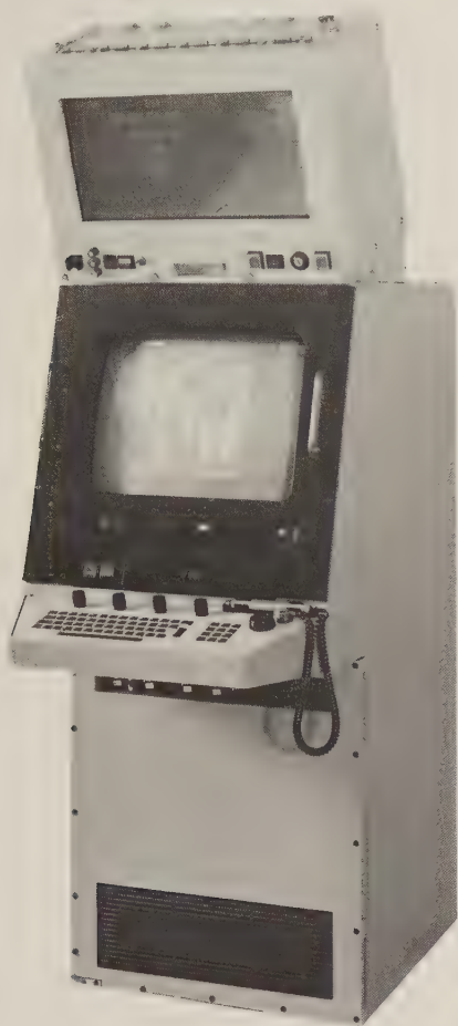
Librascope's multifunction console for SFCs Mk 2 (which uses 3 of them). (Librascope)
