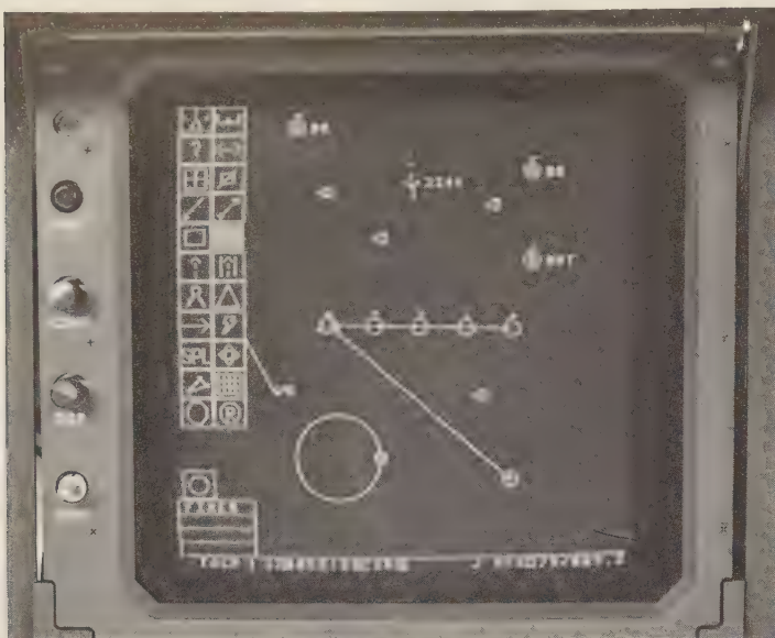
The horizontal (4 × 4-in) display of an Australian Seahawk shows, at the same time, navigational data and the tactical plot (at the center), with a fly-to point. (Rockwell)
