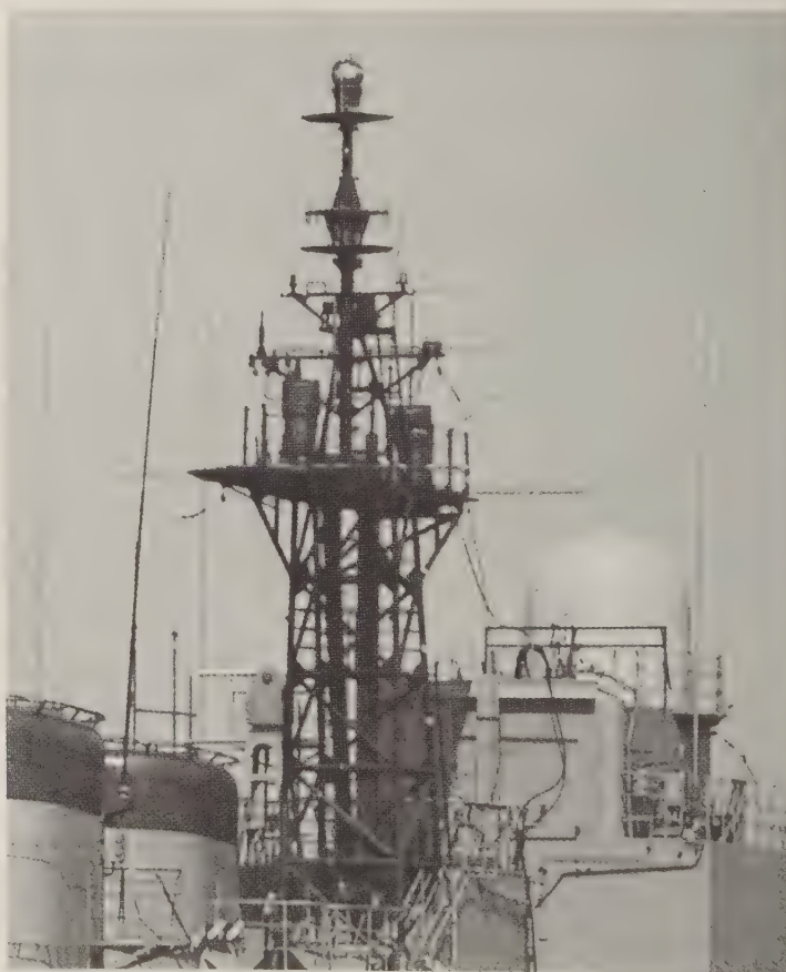
OLR-9 mainmast array (at maintop) and NOLR-6 mainmast array (radomes on platform) on board the destroyer Amagiri . The position of the cylindrical radomes varies among units of the class. The big radome is for Sea Sparrow fire control (FCS 2-12E). (Sea Power)
