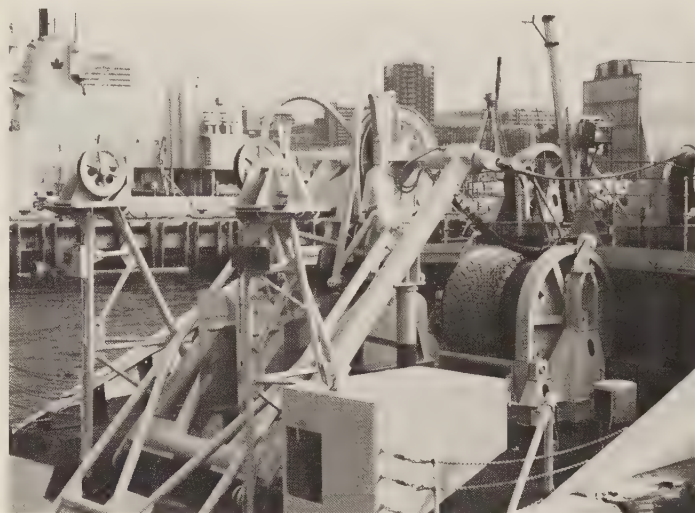
A towed array, probably SQR-18, on board a Canadian destroyer at Halifax, 1989. The fish is the towed body used in the U.S. SQS-35/SQR-18 combination. (G. Till)
