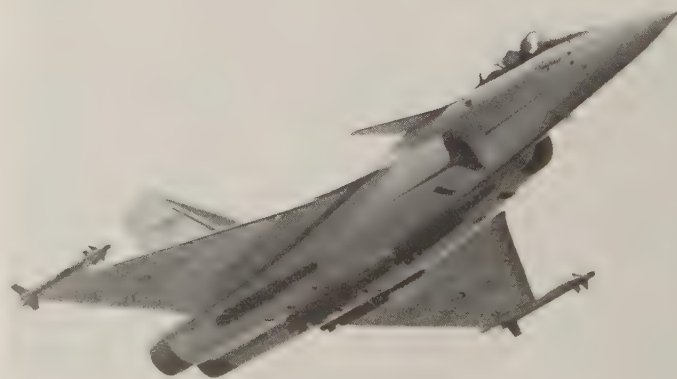
The French Rafale fighter carries Magic 2 missiles on its wing tips, with 4 Matra MICAs under its body. (MATRA)
