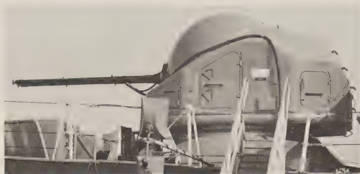
57-mm/80 Soviet-type twin mount on board the Indian frigate Ganga . The mount is designated AK-725 in Indian service. ( Ships of the World )
