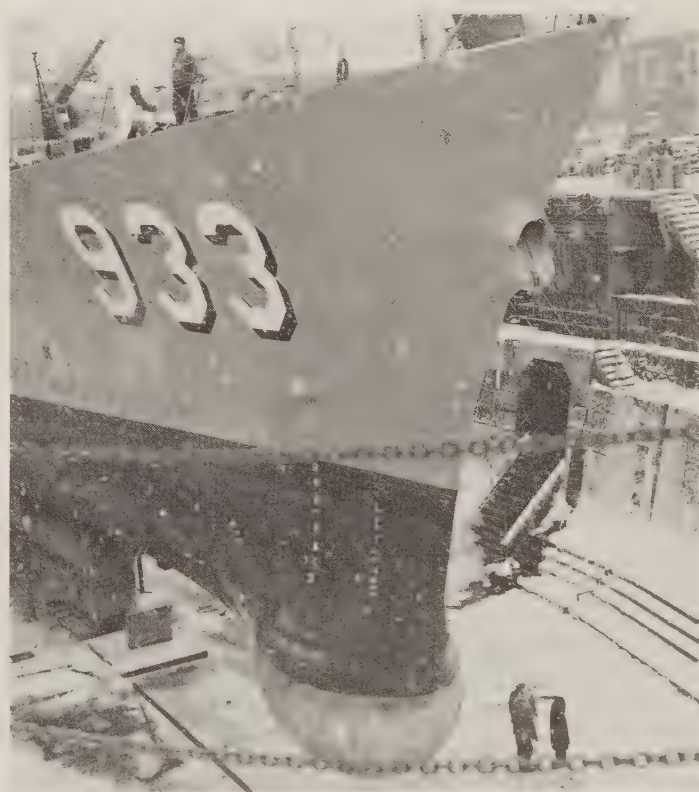
SQS-23 installed as a bow dome, USS Barry , 1959. This ship was the test installation. (U.S. Naval Institute)
