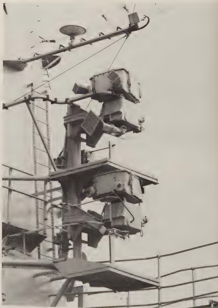
A Type 669 jammer on board a "County"-class missile destroyer (second series). Type 668 has 1 jamming unit (rather than 2) on each side, presumably sufficient to deal with 1 rather than 2 threats at a time. (R. Cheung)
