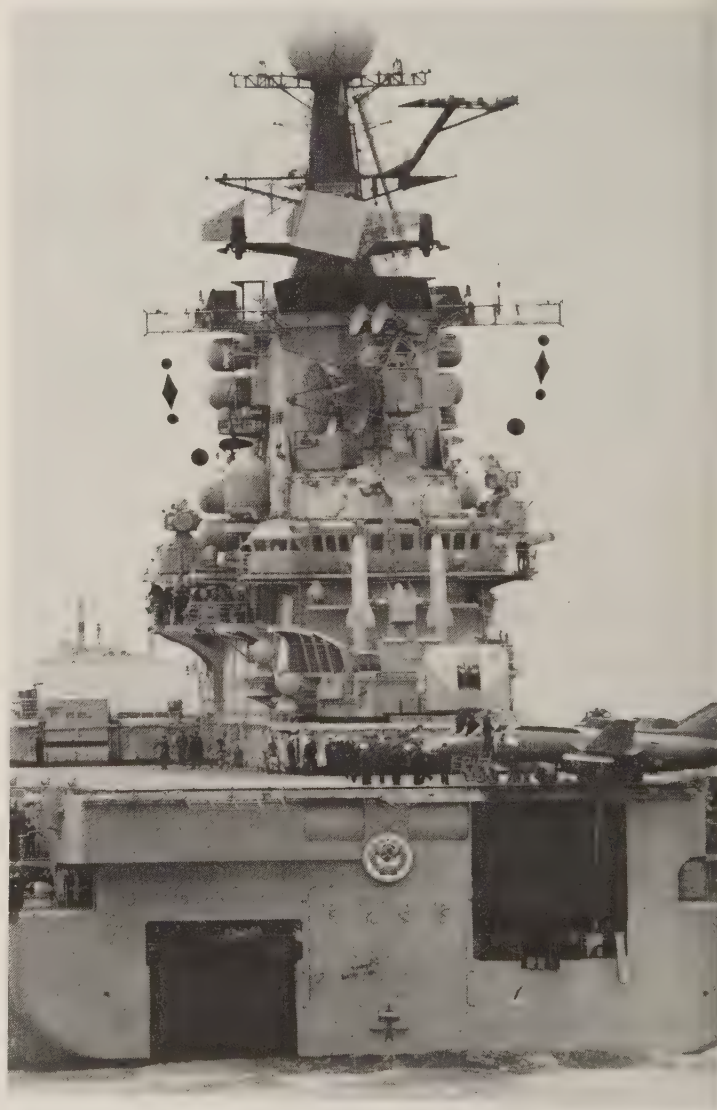
The Kiev shows a pair of SA-N-3 missiles on her after launcher. They appear blunter than they are because the dark nose radomes blend with the ship's superstructure. Note the 2 elevated dishes (missile trackers) of the ship's after Head Lights missile director. The small radomes alongside the lower one of the upper pair of Side Globes are Bell Bashes; the lower pair (not visible here) is associated with Bell Thump.
