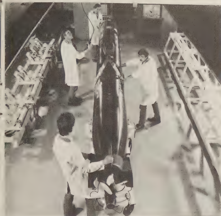
Tigerfish. This torpedo uses propellers. (Marconi)
