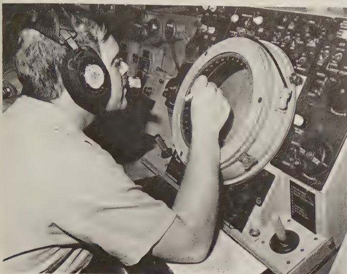
An SPA-66 precision radar scope in use in the CIC of the frigate T. C. Hart , 1986. Note the fade chart under the sailor's right elbow: it shows the fading and reinforcement of the radar beam, probably that of an SPS-49, at different elevation angles, because of interference between the direct path and the path of a signal reflected off the sea. Such a fading chart can be used for a rough estimate of aircraft altitude; frigates like this one have no long-range 3D radar. (U.S. Navy)
