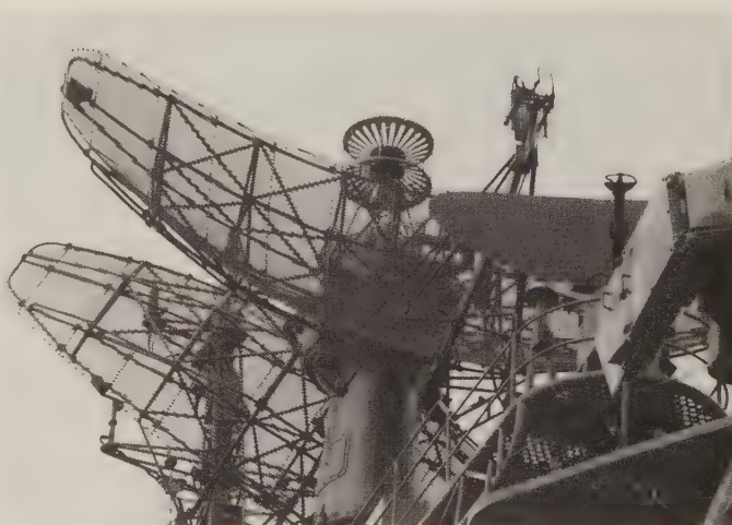
Head Net C with Hour Glass atop it on board a Soviet Krivak-class frigate, 1990. (H. J. Verhoefen)
