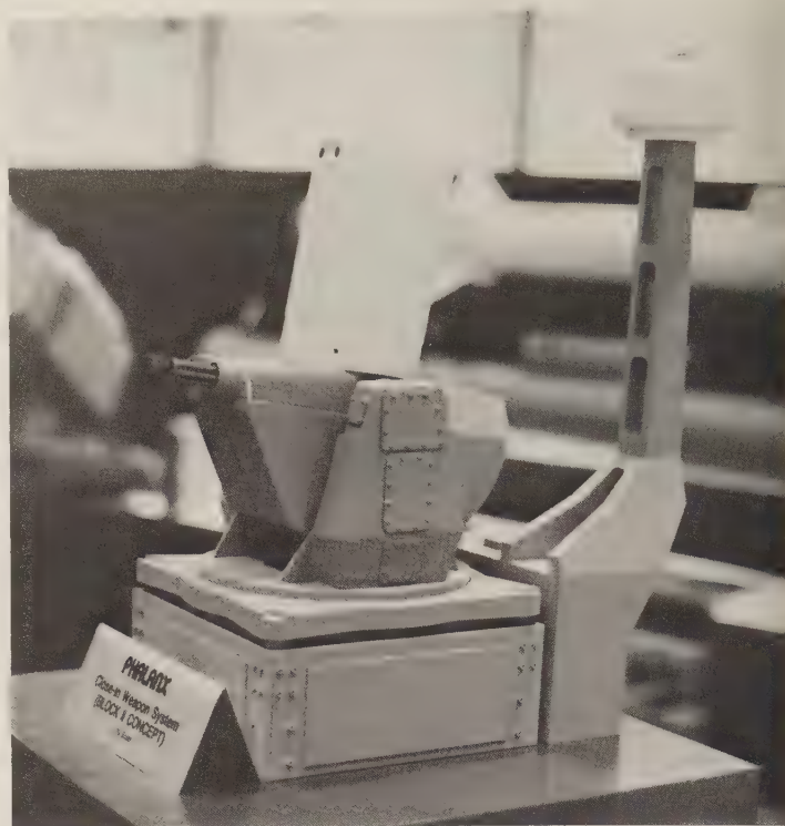
A General Dynamics Phalanx Block II concept using twin 25-mm telescoped-case guns. (Author)
