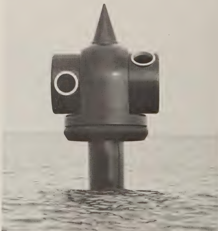
Plessey's optronic mast, with its 2 independent sensors. (Plessey)
