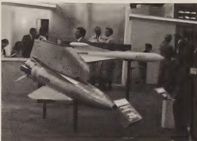
Standard French air-to-surface weapons on display at Bourget Naval 1990: AS 30L is in the foreground, and the lighter AS 15TT is behind. Note the laser-seeker window in the nose of the larger missile. As of February 1991, AS 30L had already been used in Desert Storm. (Author)
