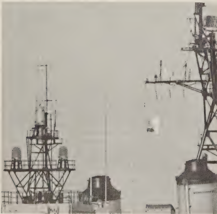
The Korean destroyer Jeong Buk is reportedly equipped with the WJ 1140 signal-collection system (the commercial version of WLR-14), presumably using the directional HF antennas visible here above the usual U.S.-type ESM radomes. ( Sea Power )
