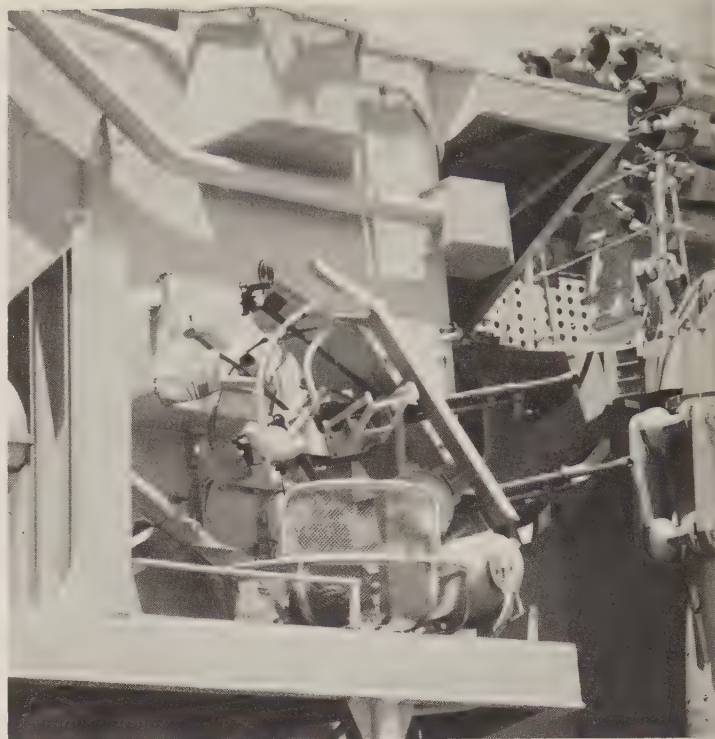
A Soviet under-and-over 12.7-mm machine gun on board the Udaloy -class destroyer Admiral Vinogradov , 1990. The ship carried 4 such mounts. (S. Zaloga)
