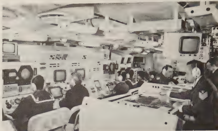
The operations room (CIC) of the Brazilian frigate Liberal (Vosper Mk 10), showing vertical consoles and a standard 2-operator horizontal display. This ship is equipped with 2 WSA 400-series systems and CAAIS 400. (Ferranti)
