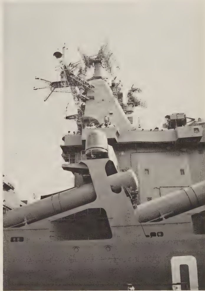
Punch Bowl, the targeting satellite data-link antenna, on board the Slava -class cruiser Marshal Ustinov , in Norfolk in 1989. (S. Zaloga)
