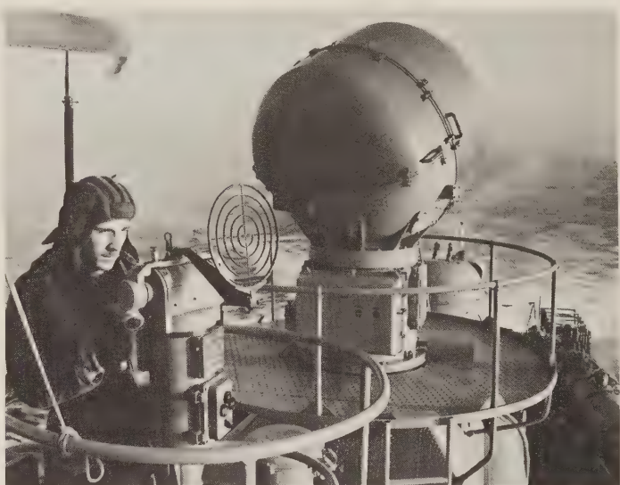
A Kolonka visual sight on board a Soviet torpedo boat. This is not a lead-computing sight; the operator uses simple speed rings to estimate the required lead. The radar in the background is Drum Tilt. (TASS from SOVFOTO)
