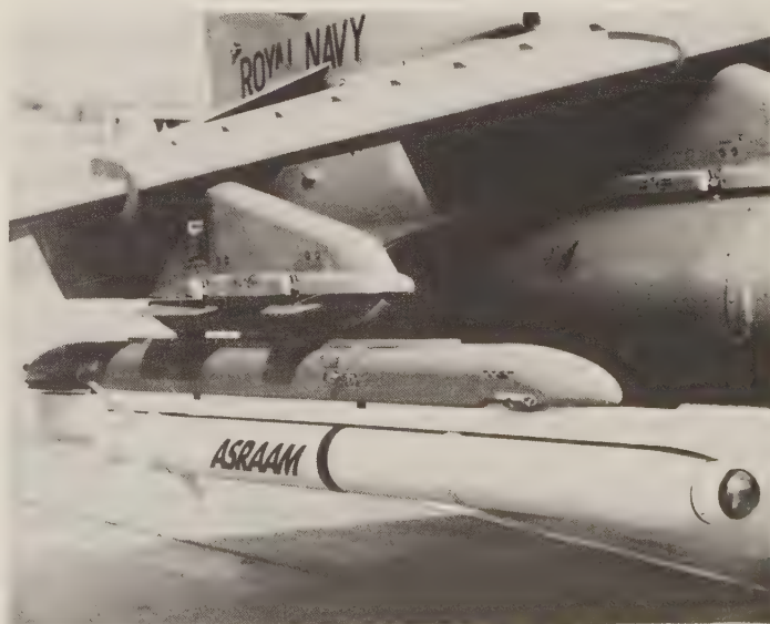
ASRAAM mock-up on a British Sea Harrier. The United States is trying to avoid using the launch-rail adapter. (British Aerospace)
