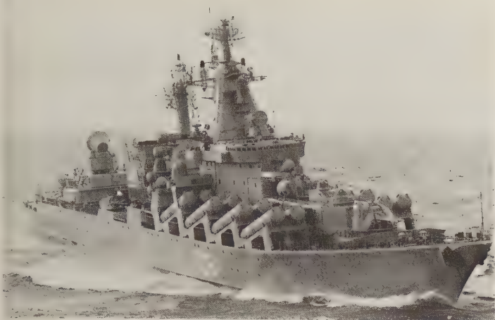
SS-N-12 missile launchers on board the cruiser Slava , 1984. Their tracker/data-link radar, Front Door/Front Piece, is on the forward side of the foremast, below the big air-search radar. Below it is a Kite Screech fire-control radar for the twin 130-mm gun forward. The air-search radar on the foremast is Top Steer; the larger back-to-back radar farther aft is Top Pair. The large fire-control radar aft is Top Dome. The small guns abaft the 130-mm turret are 30-mm Gatlings, controlled by Bass Tilt directors. (HMS Excellent )
