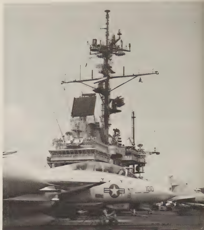
TAS Mk 23 on board the carrier Ranger , July 1986. It is the bar antenna on the mast, above the large flat plate of SPS-48C. The radar on the after side of the mast, just below it, is SPN-43, a short-range air-search set for carrier air control. (Hughes)
