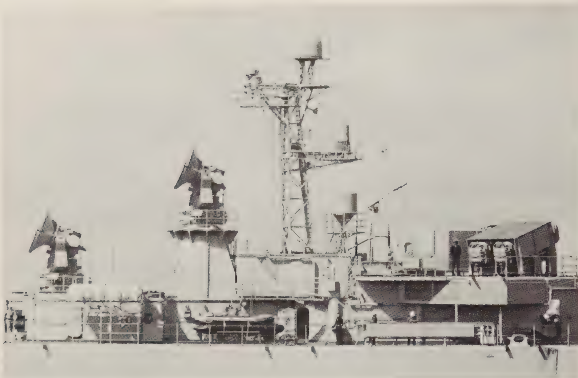
ARBB 31 occupies the squat cylindrical radome on board the destroyer Suffren (ARBB 32 is on the foremast). The radome above is for ARBR 10F. (Sea Power)
