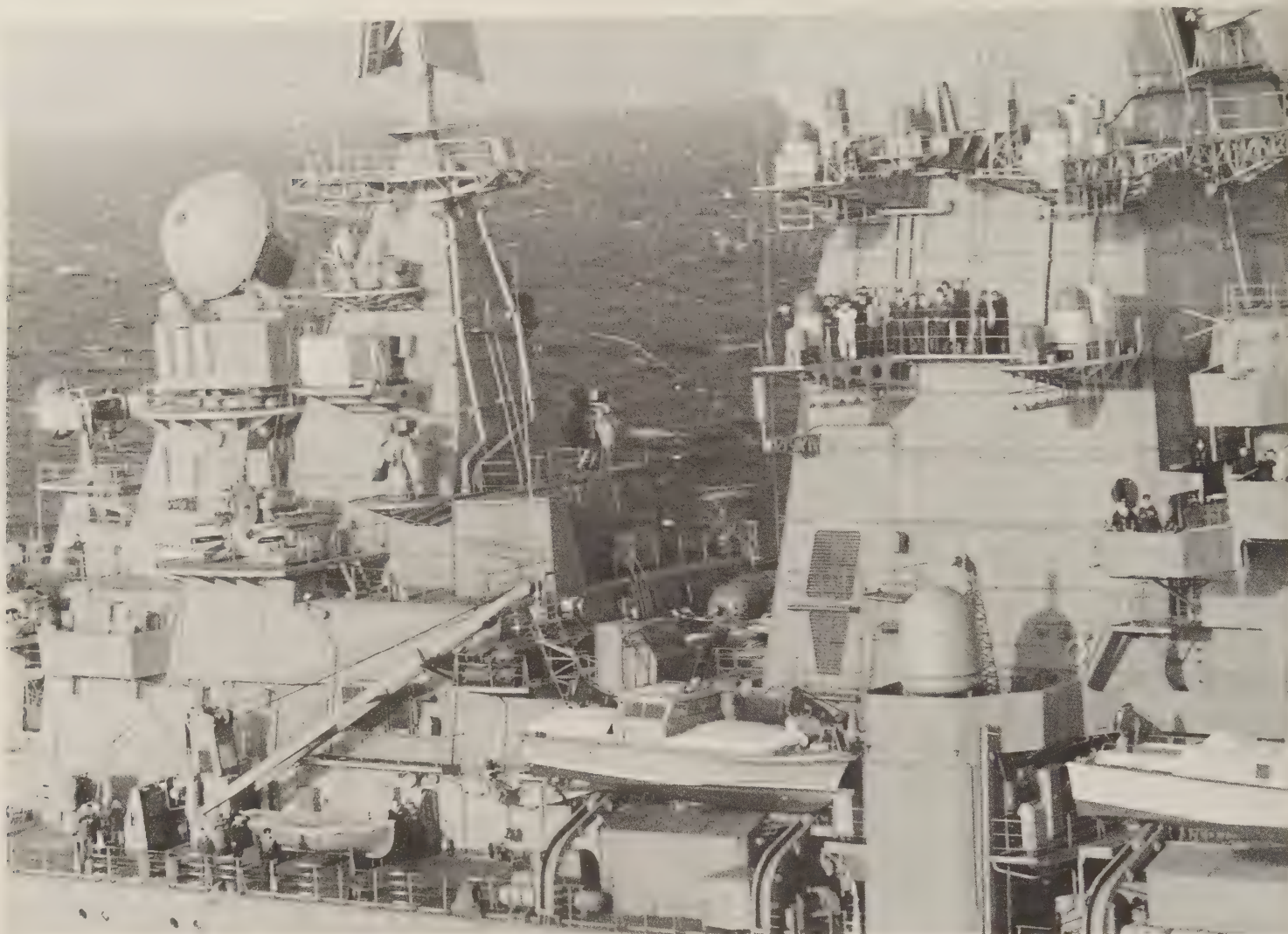
The CADS-1 air-defense system is shown on board the Soviet cruiser Kalinin , 1988. It occupies the platform below, and to the left of, the Tin Man optronic sensor. Pairs of missiles and Gatling guns flank a nodding height-finder dish. (German MoD)
