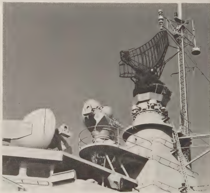
The ESM arrays around the mast (under the DA-08 radar) of this Dutch van Heemskerck -class missile frigate serve Rapids. The antennas on the mast are omnis for the system's IFM. (Signaal)
