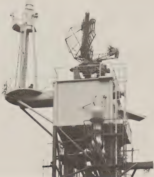
Ramses jammer (2 radomes, separated vertically, with radiation-reflecting plates between them) on board the former Dutch cruiser de Ruyter , now in Peruvian service. The radar above is DA-08. (Signaal)
