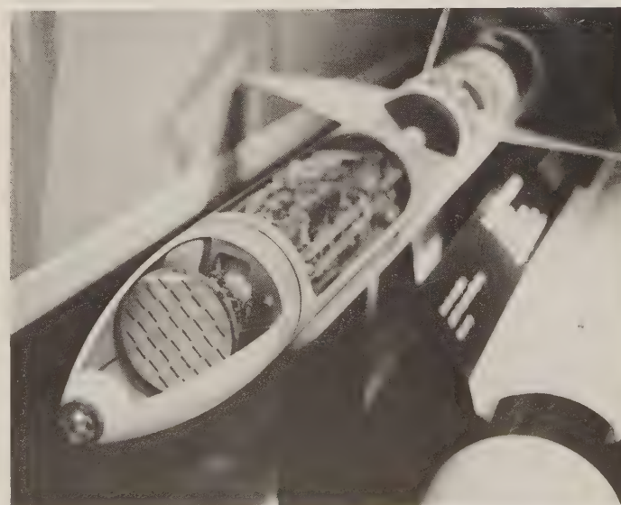
AIM-7R and RIM-7R will have both IR and semiactive radar seekers. This is the nose of an AIM-7R Sparrow, displayed at the March 1991 U.S. Navy League show. (Author)
