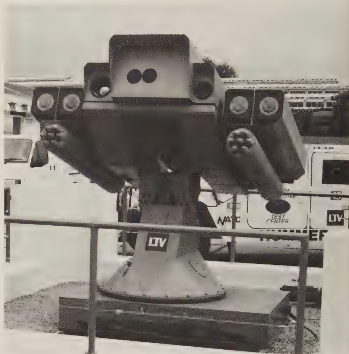
Crossbow at Farnborough, 1990, carrying a pair of 2.75-in rocket pods and 4 RBS-70 missiles. [Author]
