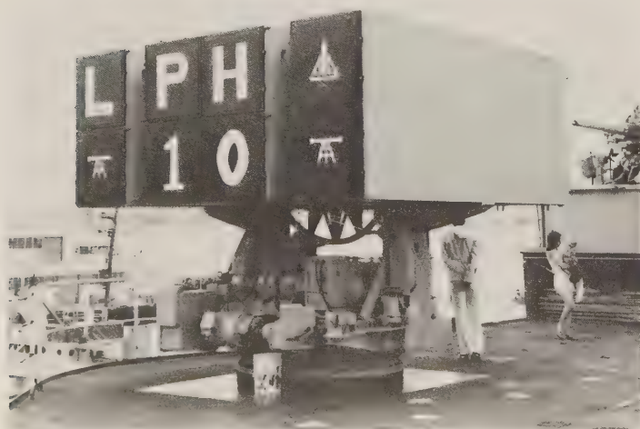
A standard Mk 25 launcher for the Basic Point Defense Missile System, on board the helicopter carrier Tripoli , July 1984. The girder in the background carries a ULQ-6 jammer. (Zeitlhofer)
