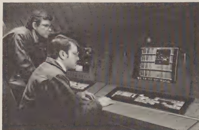
The horizontal (4 × 4-in) display of an Australian Seahawk shows, at the same time, navigational data and the tactical plot (at the center), with a fly-to point. (Rockwell)
