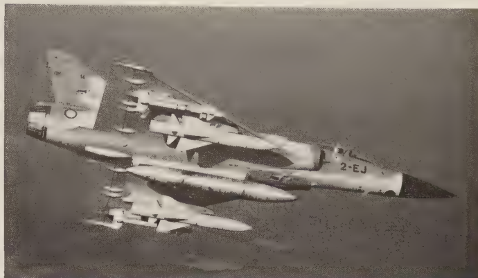
ARMAT antiradar missiles carried by a French Air Force Mirage 2000 (the smaller weapons are Magic 2s). (MATRA)
