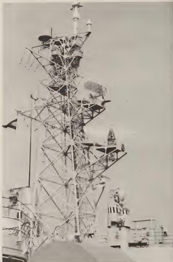
SPS-503 and (above it) SPS-10D radars on board the Canadian destroyer Annapolis , 1989. The director atop the bridge carries an SPG-515 radar. (G. Till)
