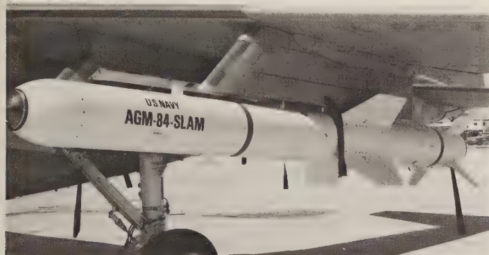
SLAM under the wing of an A-6. Note the nose window for its electro-optical sensor. (McDonnell Douglas)
