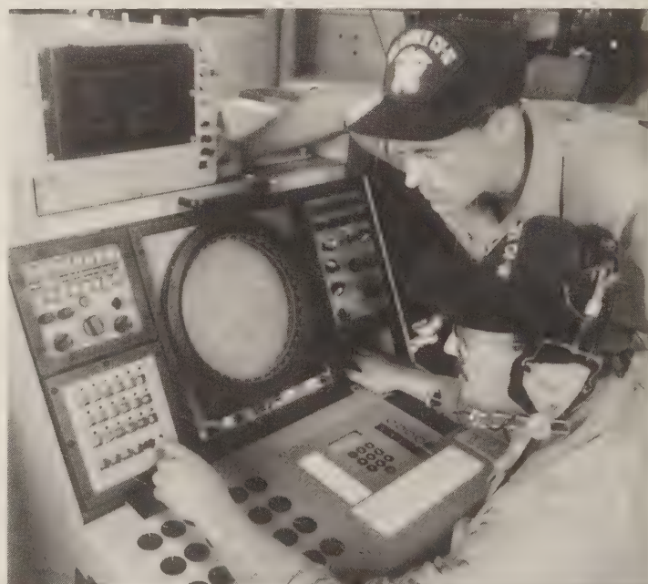
UYA-4 display of the TAS Mk 23 system, on board the carrier Ranger , July 1986. The display consists entirely of processed rather than raw video. (Hughes)
