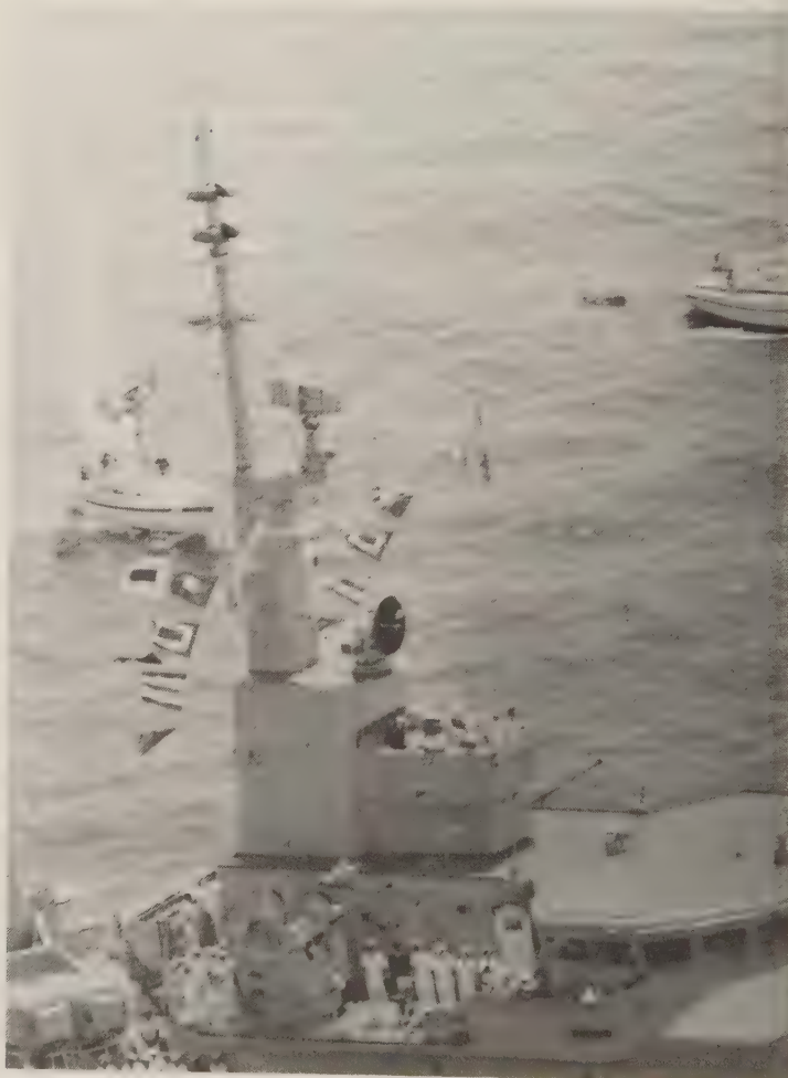
RDL-2/3 intercept and DF arrays around the foremast of a Brazilian frigate, 1986. Each array is split to fit around the mast.
