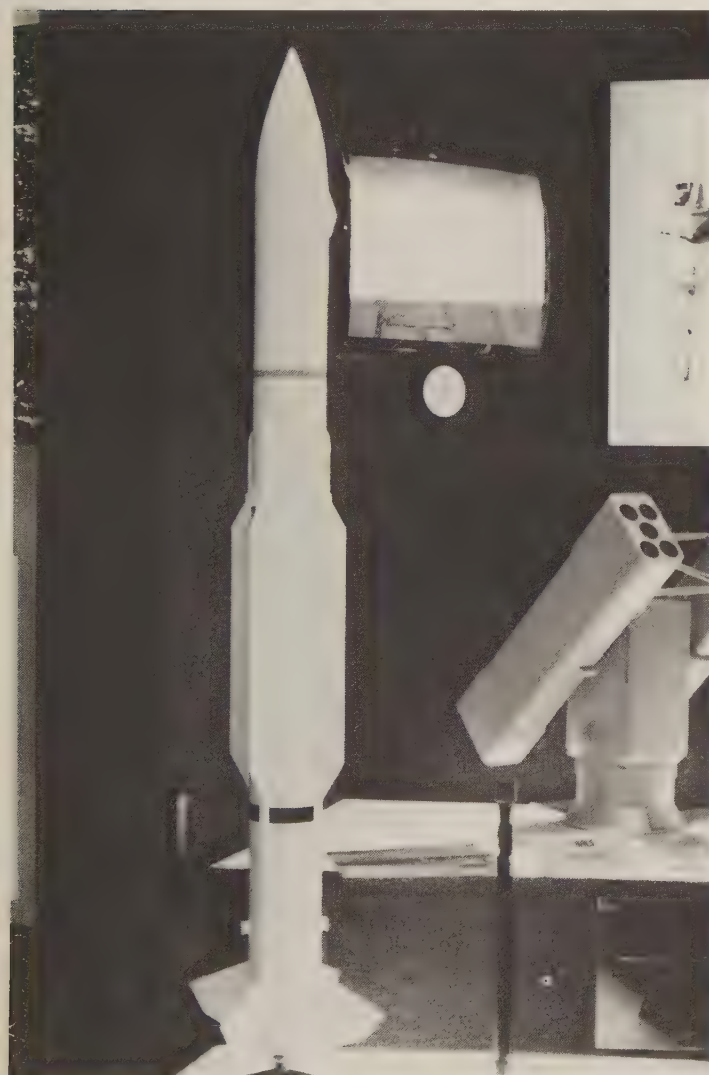
A model of SM-2 Block IIIB at the March 1991 U.S. Navy League show has a bulge forward for its IR sensor (visible on the right-hand side of the missile). The square objects visible near the tail are clips for the launch rail. (Author)
