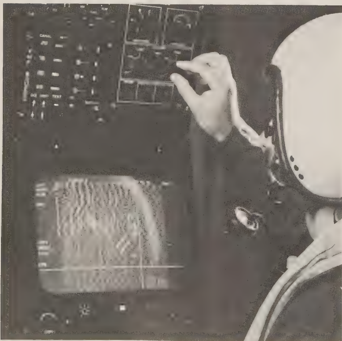
Lamparo LOFARgram display. The curved white area is a reflection from the pilot's helmet; the display proper shows the usual vertical lines, spread out over the frequency spectrum. The operator seeks lines that remain stable over time. (Thomson Sintra)
