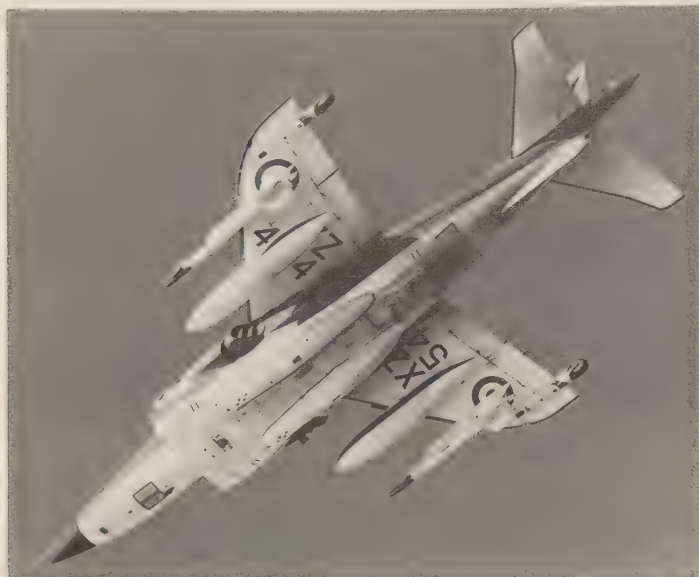
A Sea Harrier shows its 30-mm Aden gun pods, as well as 2 Sidewinder air-to-air missiles. (British Aerospace)
