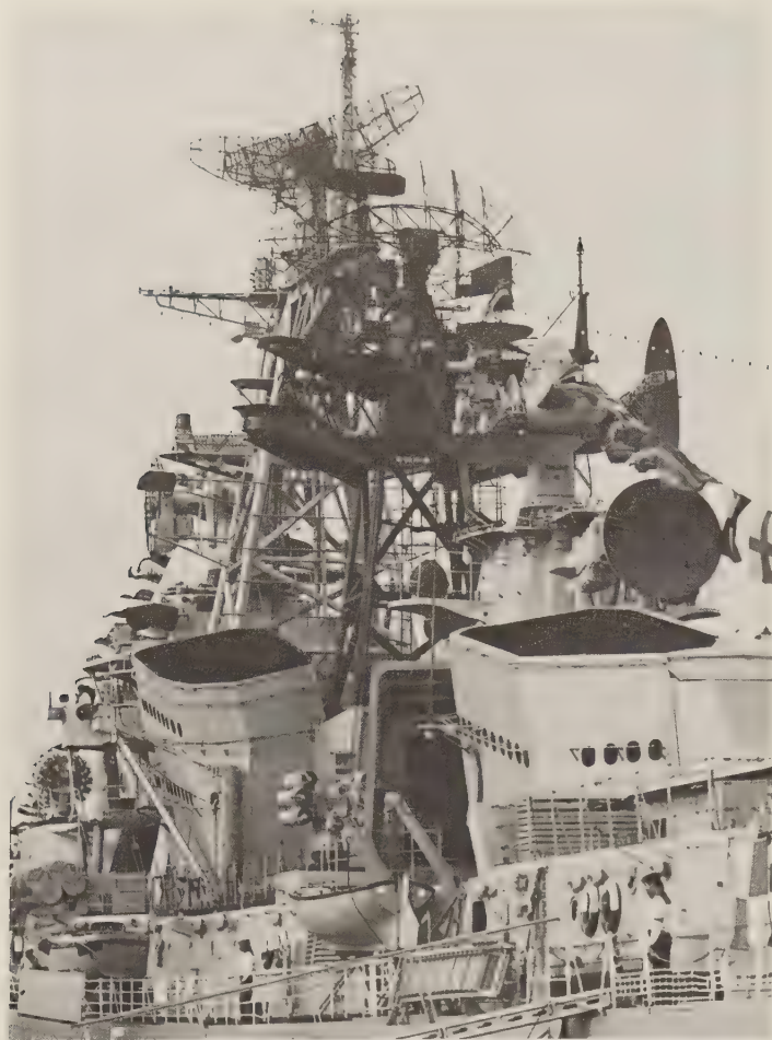
Watch Dog ESM (inboard of yardarm) and the Top Hat jammer it controls (lower left), on board the Kashin-class missile destroyer Strogii at Massawa, 1972. (Royal Navy)
