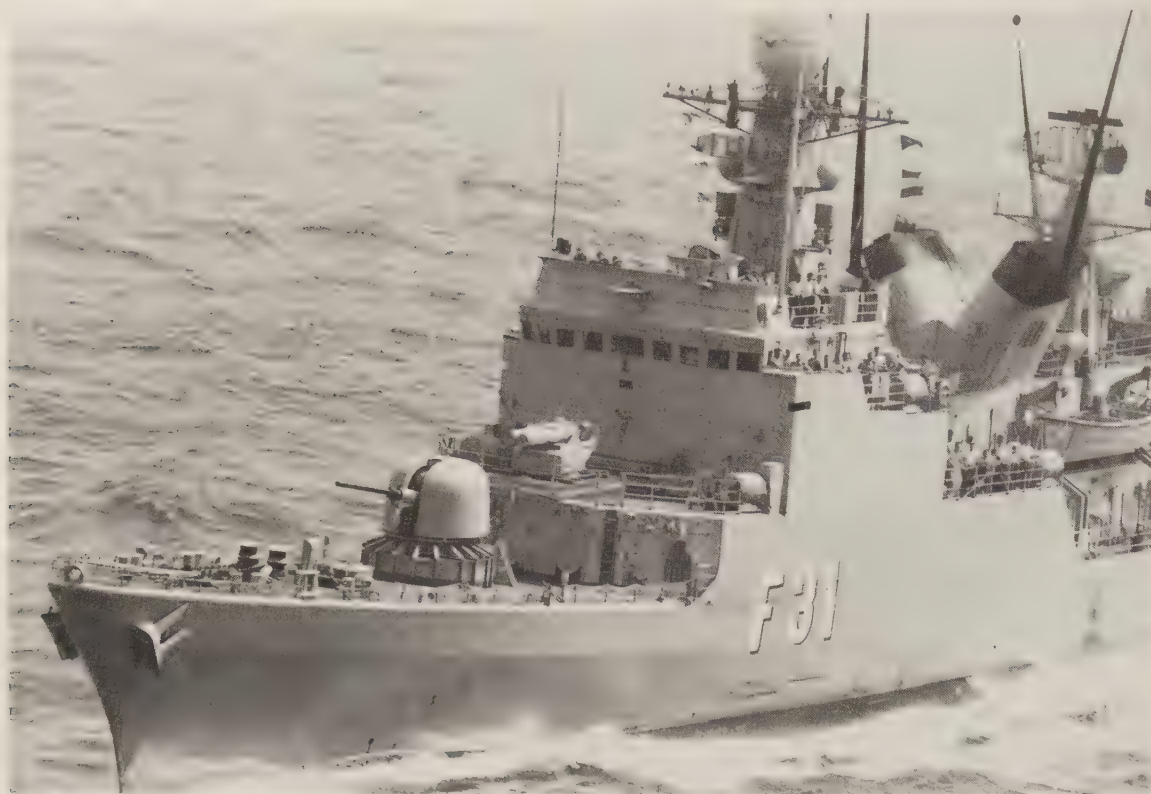
Beta radomes (a sphere above a cylinder on the side of the tower mast) are visible on board the Spanish frigate Descubierta , 1981. (Nick J. Waters III)
