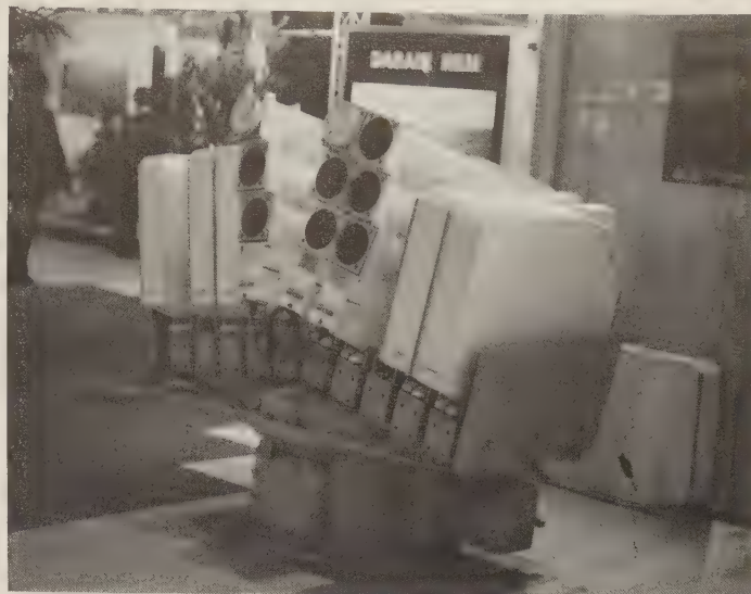
DAGAIE Mk 2 in 1990, showing the SAGAIE tubes between the standard "suitcases." (Author)
