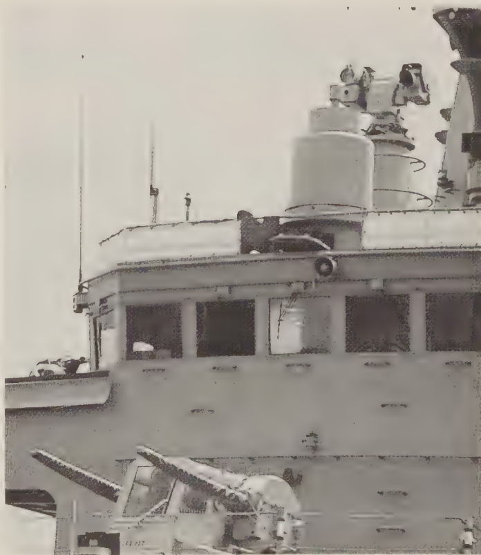
An ARGOSystems ESM antenna (probably Phoenix II) on board a Korean Ulsan -class frigate, with a Radamec HWK 409-029 electro-optical director visible behind it, and an Emerlec-30 mount below. Similar radomes can be seen on board Colombian FS 1500-type frigates, Finnish Helsinki -class fast attack boats, New Zealand Leander -class frigates, and Swedish Stockholm and Spica-II classes. ( Sea Power )
