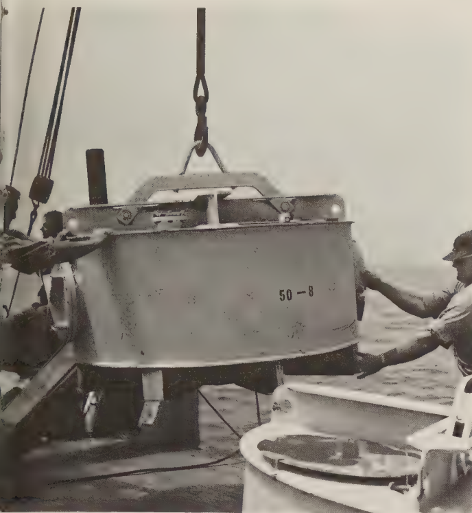
Mine Mk 51 (practice version). The vertical tube is the magnetic-induction sensor. This and Mk 18 are the only U.S. mines in the form of upright cylinders. (U.S. Navy)
