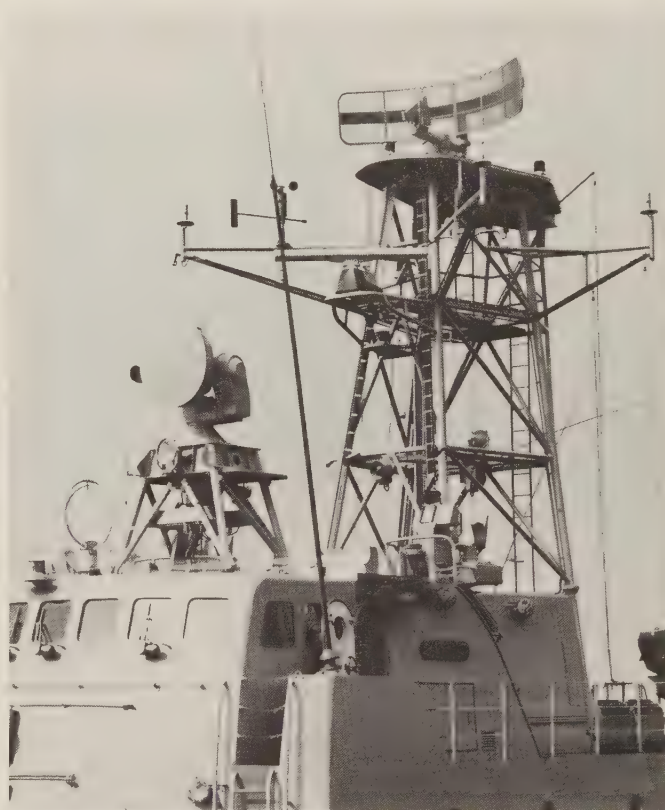
A Nigerian Combattante-IIIIB-class fast attack boat shows a Triton radar at her masthead, with a Castor II director; at the right, at the foot of the mast, is a Panda optical director. (U.S. Naval Institute)
