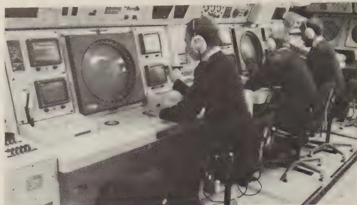
Standard ADAWS 2-operator vertical consoles. Note the use of the light pen for data entry. (Plessey)
