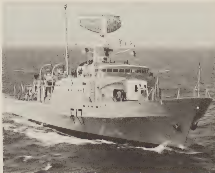
The Ghanaian corvette Kromantse uses AWS-1 as her air-search radar. The small slotted waveguide serves a Type 978 navigational set. This ship and her sister are armed with single 4-in and 40-mm guns and with Squid. (U.S. Naval Institute)
