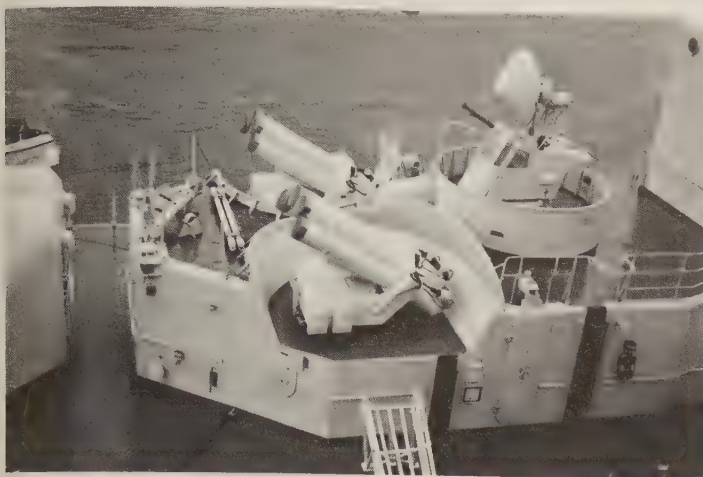
An M45 director on board the German training ship Deutschland , now discarded. A similar radar, without a manned cab, was mounted above the ship's bridge. (R. Cheung)
