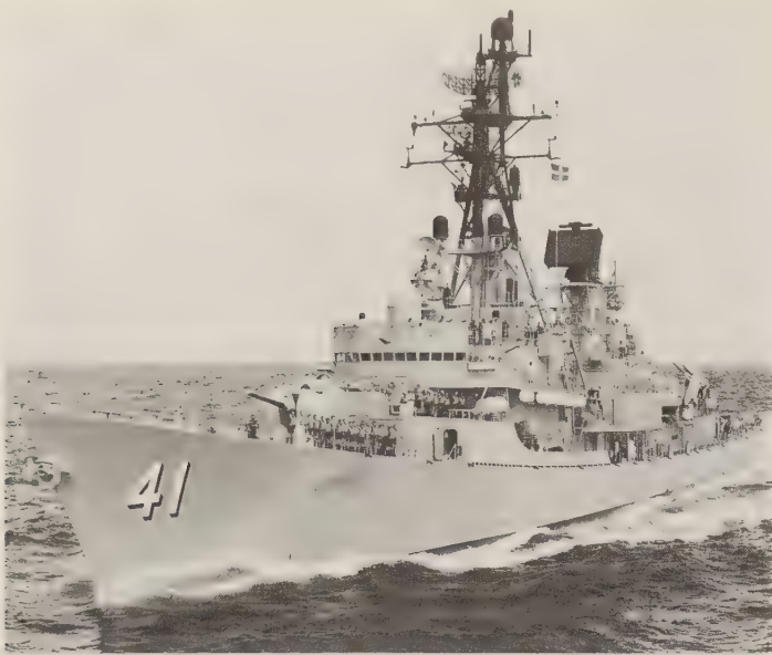
Ikara on board the Australian destroyer Brisbane , on the small launcher on the side amidships. The main radars are SPS-40 (foremast, with SPS-10 below it) and SPS-52 (the flat plate aft), with 2 SPG-51 missile-guidance radars below. The big radome atop the bridge is the Ikara guidance link. (U.S. Naval Institute)
