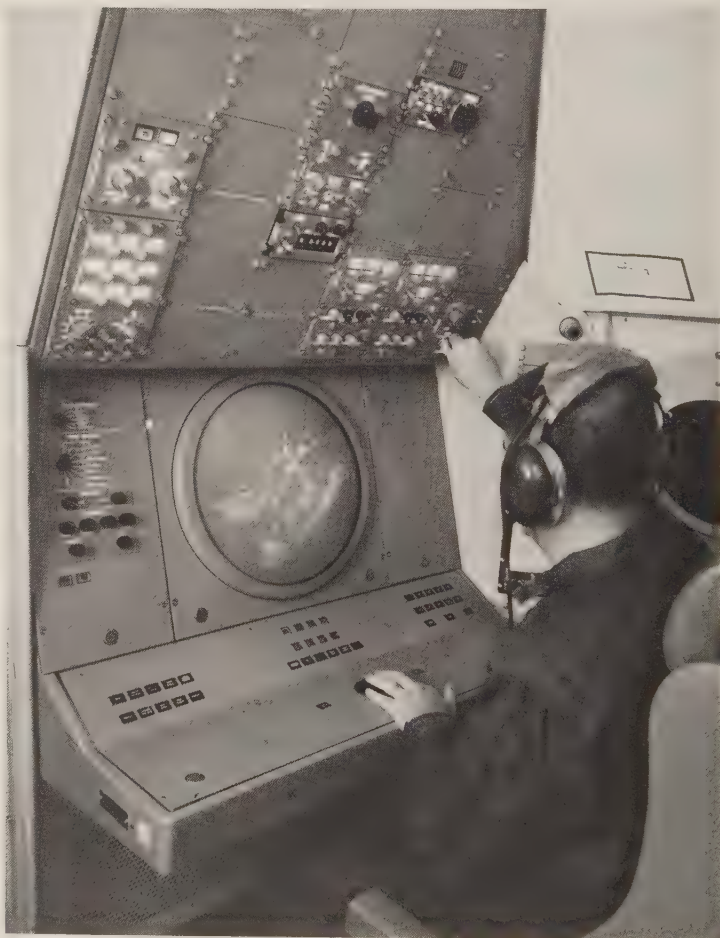
A computer can draw synthetic video on a screen. This is a cursive display, in which the synthetic video is superimposed over raw radar video. The next stage is a full raster-scan display, in which the computer can process the raw video on the screen. This ASA-70 console is on board a P-3C Orion. (U.S. Navy)
