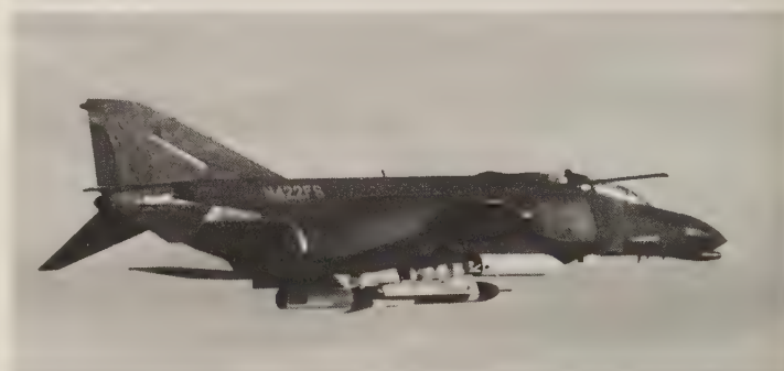
McDonnell Douglas and Hughes launched their first advanced interception weapon system (AIWS) on 10 December 1990. The AIWS is designed to replace current standoff weapons such as Maverick, Skipper, Walleye, and laser-guided bombs. (McDonnell Douglas)
