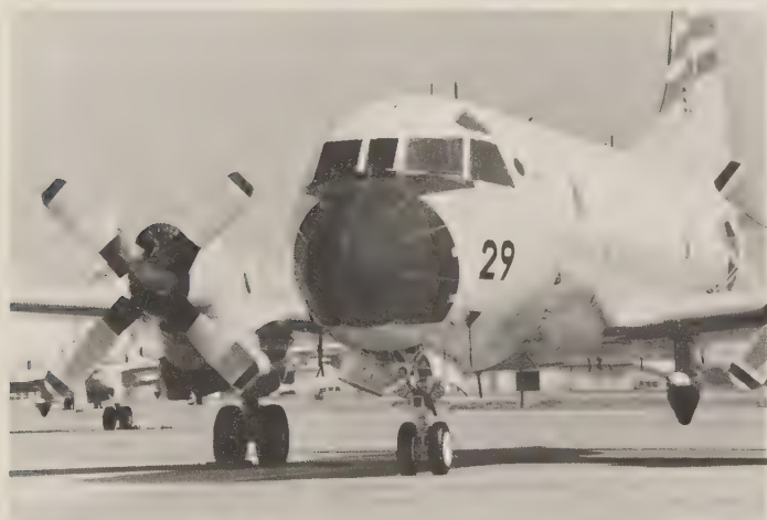
This Japanese P-3C shows an ALQ-78 radome under its port wing root (to the right in this picture). (W. Donko, 1989)
