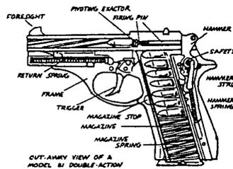
CUT-AWAY VIEW OF A MODEL 81 DOUBLE-ACTION BERETTA PISTOL
