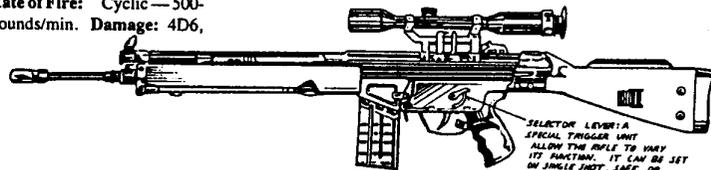
SELECTOR LEVER: A SPECIAL TRIGGER UNIT ALLOW THE RIFLE TO VARY ITS FUNCTION. IT CAN BE SET ON SINGLE SHOT, SAFE, OR AUTOMATIC.
