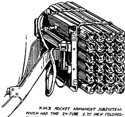
XM3 ROCKET ARMAMENT SUBSYSTEM
